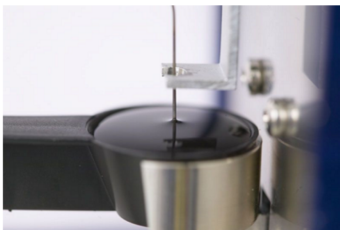
Figure 2.3: Representation of the probe position during the surface tension measurements. 123
