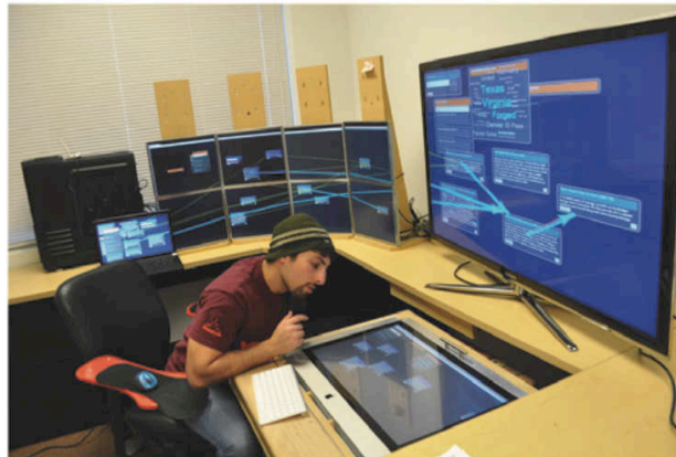
Figure 2.10. SAViL provides direct visual links among different types of objects on multiple heterogeneous displays [74].
