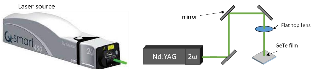
Figure II-44 Image of the Nd:YAG laser with frequency doubling crystal and corresponding schematic of the laser exposition setup
