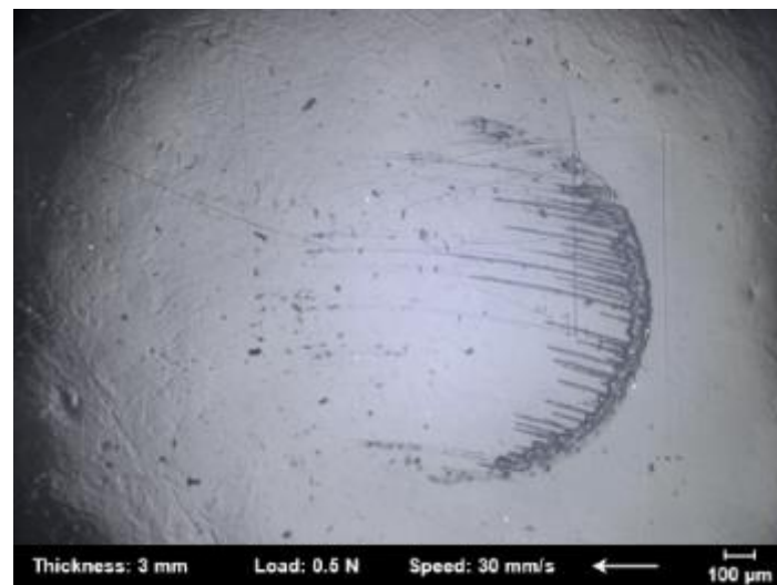
(b) After a friction of 0.5 N – 30 mm/s on a 3 mm thick DN gel
