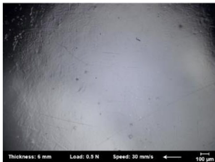
(a) After a friction of 0.5 N – 30 mm/s on a 6 mm thick DN gel
