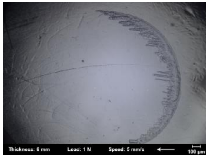
(a) After a friction of 1 N – 5 mm/s on a 6 mm thick DN gel
