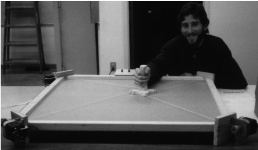
FIGURE 1.4 – Prototype de robot plan horizontal du CSHI [Williams (1998)]
