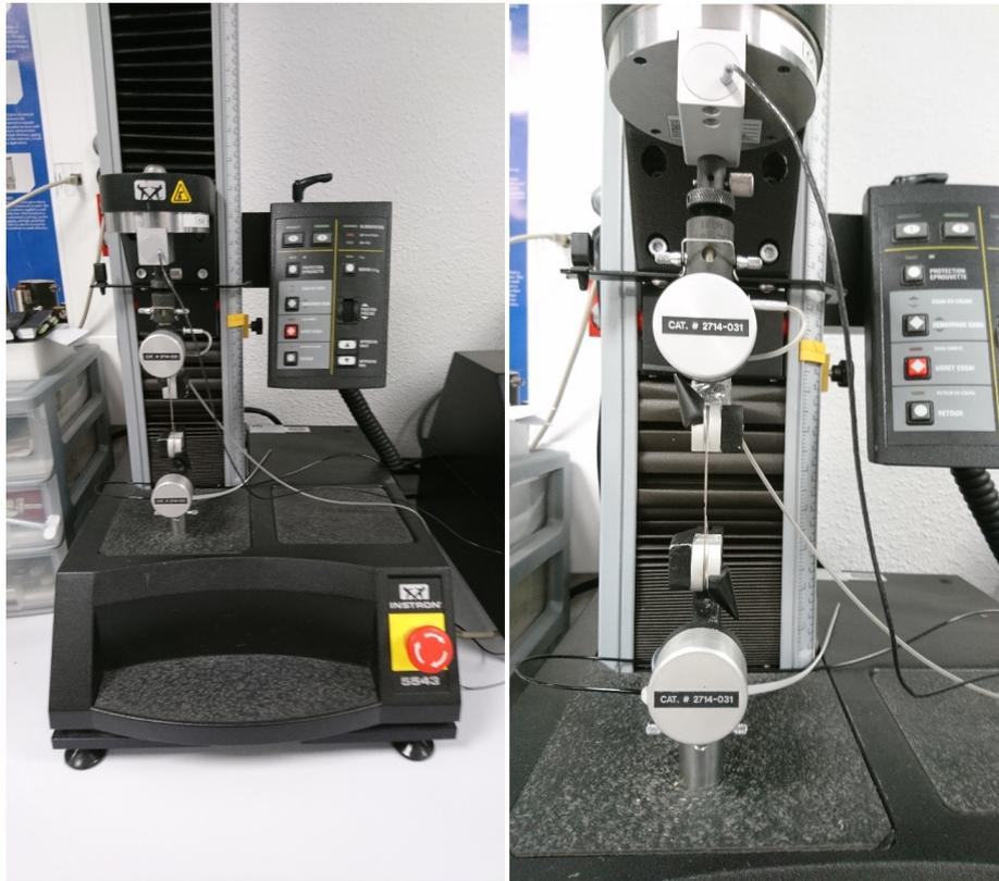
FIGURE 4.7 – Machine de traction Instron 5543.
