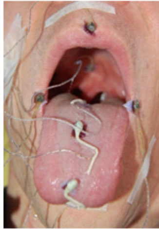
Figure 5. Electromagnetic articulography (EMA). Coils are glued to the lips, the jaw, the tongue and velum. The jaw sensor was glued at the base of the incisors and is not visible the images. This set-up was used for the recording of the BY2014 articulatory-acoustic corpus presented in section 7.2.3. Reprinted from Bocquelet et al. (2016c).
