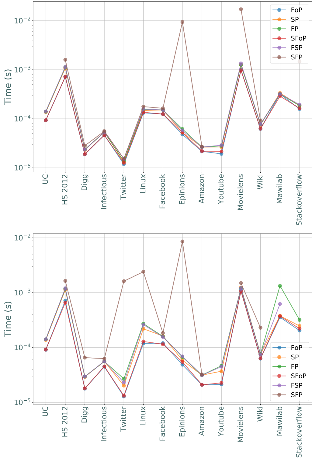
Figure 5-4: Running Times (s) of the L-Algorithm for the foremost, shortest fastest, shortest foremost, fastest shortest and shortest fastest path problems (top: random sources, bottom: high degree sources).
