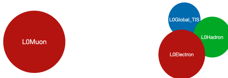
Figure 4.1 – The previous L0 trigger strategy of R_K and R_{K^*} analysis. The \mu\mu modes (left) only use the L0Muon while the ee modes (right) use the LOElectron as primary, L0Hadron as secondary and LOGlobal_TIS as tertiary categories.
