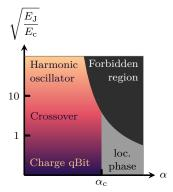
Figure **6.1**: The various parameter regions of the charge-boson model at fixed  $E_{\rm J}$ , sketched from Sec. **4.3**. The spin-boson line separates the localized phase. In the delocalized/superconducting region, a smooth crossover connects the damped harmonic oscillator to the damped charge qBit.
