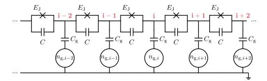
Figure 7.2: A one dimensional array of Josephson junctions. Each superconducting island is biased by a different charge offset  $n_{g,j}$ .
