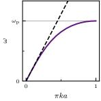
Figure 3.3: The expected dispersion relation as a function of adimensional wavenumber (a is the size of a junction).  $(--) \omega = f(\pi ka),$  (--) Long wavelength approximation.
