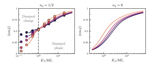
Figure 6.7: Phase fluctuations for several coupling strength, at  $n_{\rm g} = 0$  and  $n_{\rm g} = 1/2$ . The later displays two regimes: localized charge at  $E_{\rm J}/E_{\rm c}$  < 1, localized phase otherwise.  $E_{\rm J}$  is fixed at  $\omega_{\rm M}/10$ .  $(\bullet): \alpha/\alpha_{\max} = 0.1,$  $(\bullet): \alpha/\alpha_{\max} = 0.3,$  $(\bullet): \alpha/\alpha_{\max} = 0.5,$ (•) :  $\alpha/\alpha_{\text{max}} = 0.8$ ,
