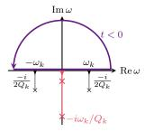
Figure 8.7: Green's function poles in complex  $\omega$  plane. (•) Q > 1/2, (•) Q < 1/2. (•) Residue theorem contour. <sup>3</sup> R. D. Mattuck. 1976. A Guide to Feynman Diagrams in the Many-body Problem.
