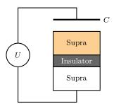
Figure 1.4: Single Cooper pair circuit. The top superconductor (•) forms an island.
