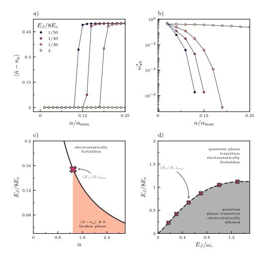
Figure 4.6: a) Order parameter as a function of dissipation strength for various  $E_{\rm J}/E_{\rm c}$ , at  $E_{\rm J}=\omega_{\rm c}/10$ , and degeneracy point  $n_{\rm g}=1/2$ . A critical point is only observed for  $E_{\rm J}/E_{\rm c}<1$ .
