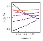
Figure **6.8**:  $E_1^{\star}$  as a function of the coupling strength, computed with and without  $w \neq 0$  winding numbers.  $E_{\mathrm{c}} = \omega_{\mathrm{M}}/10$  is fixed, and  $n_{\rm g} = 1/2.$
