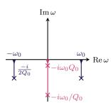
Figure **6.3**: Poles position in complex  $\omega$  plane. (•)  $Q \gg 1/2$ , (•)  $Q \ll 1/2$ .
