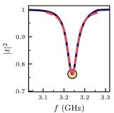
Figure 10.17: Close-up of (—) a transmission peak, and (--) its Lorentzian fit. (o) signals the numerically detected peak position.
