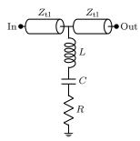
Figure **8.8**: Hanging resonator model.
