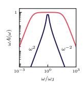
Figure 9.1: Band-pass filter effect in the spectral density. (•)  $Z_c/Z_J \gg 1$ ,
