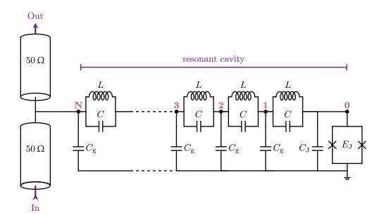
Figure 8.2: The boundary sine-Gordon circuit simulator. A long chain of N junctions forms a bosonic field, strongly coupled via a boundary Josephson term by the SQUID on site 0, with tunable Josephson energy  $E_{\rm J}$ . The chain is side-coupled to the probing 50  $\Omega$  pads.
