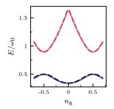
Figure **5.9**: ( $\bullet$ ) Ground state and ( $\bullet$ ) first excited level energy for admittance y=0.4 as a function of  $n_g$ . ( $-\bullet$ ) optimized ansatz, ( $-\bullet$ ) exact result.
