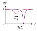
Figure 8.11: ( $\bullet$ ) Line shape at  $\Sigma=0$ . The width is finite, and minimum transmission is 0. ( $\bullet$ ) Line shape displaced of
