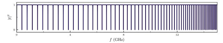
Figure 10.2: Transmission at  $\Sigma = 0$  and  $Z_{\rm tl} = 100 \,\Omega$ , for better peak visibility.
