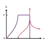
Figure 10.1: Wavenumber as a function of frequency. arrows indicate an asymptote to  $\infty$ .
