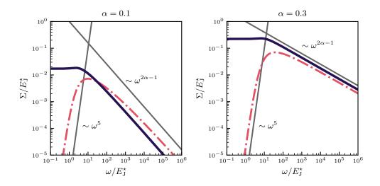
Figure 9.9: Self-energy in the scaling limit  $\omega_c \gg E_{\rm I}^{\star}$ , numerically computed on a logarithmic grid at two values of  $\alpha$  below the Toulouse point. The high and low frequency power laws matches with analytical predictions. (•): Im  $\Sigma(\omega)$ , (•): Re  $\Sigma(\omega)$ ,
