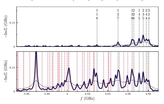
The resonances are labeled by the number of the modes involved, e.g. (1,2,7) peak corresponds to a splitting in 3 photons occupying modes number 1, 2 and 7. We see that this peak grove is composed of  $\omega \sim 10 \,\omega_{\rm min}$  resonances,  $\omega_{\rm min}$  the fundamental frequency of the array. For a linear dispersion relation, all these resonances would be
