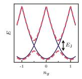
Figure 2.2: 2 lowest energy levels at ( $\bullet$ )  $E_J=0$  and ( $\bullet$ )  $E_J\neq 0$ .
