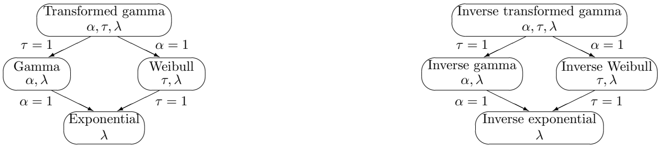
Figure 2.1 – Interrelations between distributions of the transformed gamma and inverse transformed gamma families. Diagrams derived from Figure 5.3 of Klugman et al. (2012).
