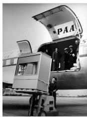
FIGURE 4.1: The IBM 305 RA-MAC introduced in 1956 and weighing 1 Ton could hold 5 MB for the monthly price of \$30.000.
