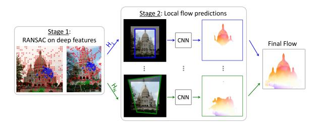
Figure 5.2: **Overview of RANSAC-Flow.** Stage 1: given a pair of images, we compute sparse correspondences (using off-the-shelf deep features), use RANSAC to estimate a homography, and warp second image using it. Stage 2: given two coarsely aligned images, our self-supervised fine flow network generates flow predictions in the matchable region. To compute further homographies, we can remove matched correspondences, and iterate the process.
