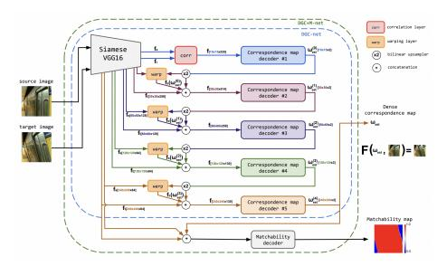
Figure 2.6: DGC-Net proposed in (Melekhov et al., 2019), which is an iterative architecture consisting of four major components: 1) the feature pyramid creator. 2) the correlation layer. 3) the fully convolutional correspondence map decoders. 4) the warping layer. The matchability decoder is a tiny CNN that predicts a confidence map of correspondences.
