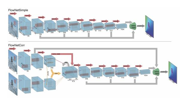
Figure 2.4: Proposed two CNN architectures in Flownet1 (Dosovitskiy et al., 2015).
