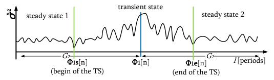
Figure 7.3: State selection V1: Visualizing the calculation of the start and end sample of a transient. The proposed event from stage one is marked blue whereas the calculated start and end positions are marked in green.
