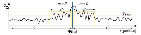
Figure 7.4: State selection V2: Exemplary representation of  $\hat{\sigma}^2$ , visualizing a transition between a SSts and a TSts. The yellow windows  $w_s$  and  $w_e$  with the length  $G_1$  start at  $\Phi_1$ .
