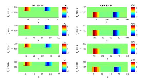
Figure 5.16: Different sampling rates of a turning on (left side) and off (right side) process of an energy saving lamp, from BLUED dataset [4], presented with FIT-PS. Sampling rates from  $12\,\text{kHz}$  to  $1.2\,\text{kHz}$  are illustrated. Thereby the numbers of dimensions k are variating from 200 to 25 while the number of 200 periods in l direction is constant. The amplitude of the current is represented colored.
