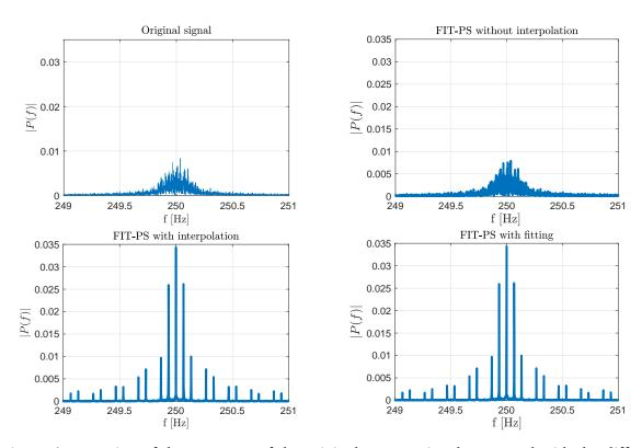
Figure 6.3: Section of the spectrum of the original current signal compared with the different FIT-PS methods
