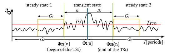
Figure 7.5: State selection V2: Exemplary representation of  $\hat{\sigma}^2$ , visualizing a transition between a SSt and a TSt. The windows have been moved by  $n_1$  or  $n_2$  values until all values are below the threshold  $Tr_{TSt}$
