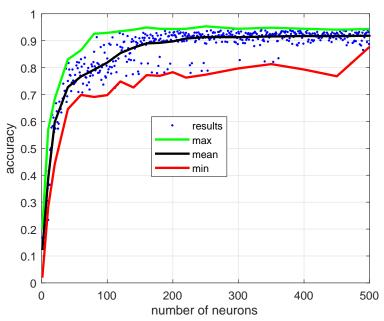
Figure 9.25: Validation results of a feed forward net using P, Q, and HARs for a different number of neurons. The limits of accuracy are calculated by 100 iterations with different initialization settings and different number of neurons. [68]
