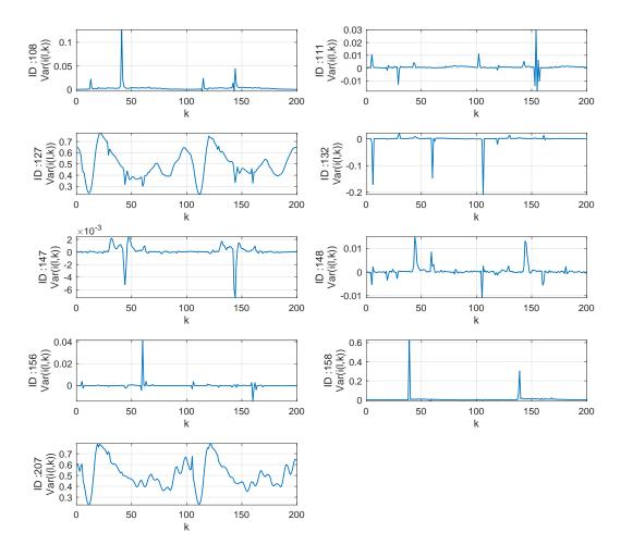
Figure A.2: Using the variance of the current amplitude transformed by FIT-PS as SSF of different devices of the BLUED dataset.
