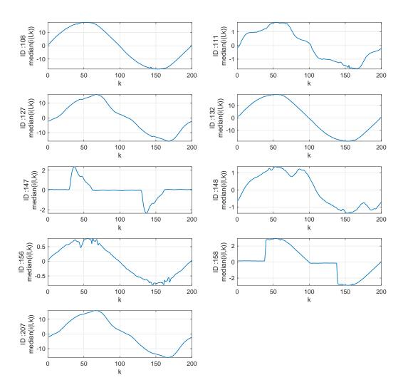
Figure A.3: Using the median of the current amplitude transformed by FIT-PS as SSF of different devices of the BLUED dataset
