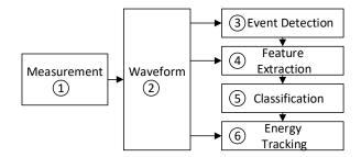
Figure 2.3: Common information flow in NILM. In comparison to the usual linear presentation of the processing chain of the NILM tasks, see Fig. 2.1, the information flow is not purely linear in a row.
