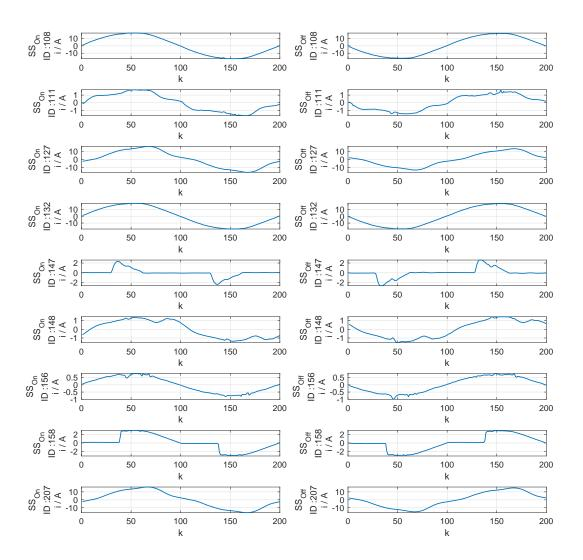
Figure A.1: Using the current amplitude transformed by FIT-PS as SSF of different devices of the BLUED dataset.
