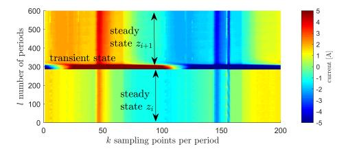
Figure 5.11: FIT-PS waveform with 200 sample points per period; SSt  $z_i$ : device one; TSt  $z_{i+1}$ : switching on procedure of a refrigerator; SSt  $z_{i+2}$ : device one and two. Published in [66].
