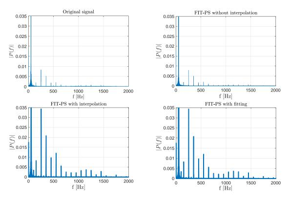
Figure 6.2: Frequency spectrum of the original current signal compared with the different FIT-PS methods (vertical axis clipped at 0.035)
