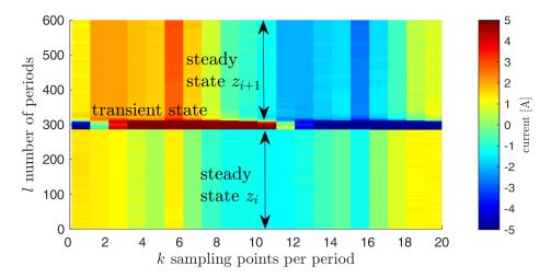
Figure 5.10: FIT-PS waveform with 20 samples per period SSt  $z_i$ ; TSt: switching on procedure of a additional device (refrigerator); SSt  $z_{i+1}$ : devices from SSt  $z_i$  and the refrigerator.
