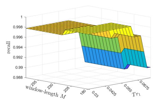
Figure 7.14: Representation of the recall dependency of two parameters of the event detection using the PCA. The results are based on phase A of the BLUED dataset. Modified from [70].
