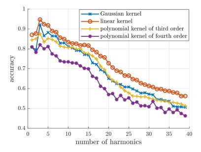
Figure 9.20: Validation results of the SVM for the feature combination P, Q, and HARs and a varying number of HARs
