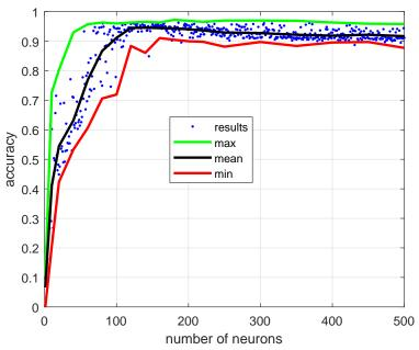
Figure 9.26: Validation result of a feed forward net using FIT-PS for a different number of neurons. The limits of accuracy are calculated by 100 iterations with different initialization settings and different number of neurons.[68]
