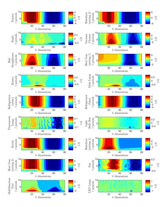
Figure 8.8: Illustration of the TSts with FIT-PS signal representation, for all appliances of the HELD1 dataset.
