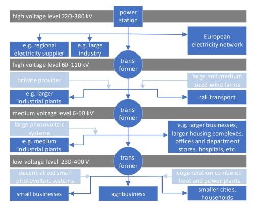
Figure 9.34: Structure of the power grid. Modified from [48]
