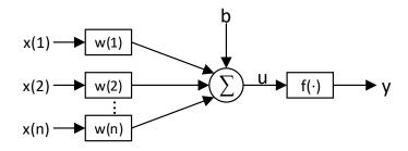
Figure 9.6: Model of an artificial neuron
