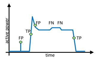
Figure 2.11: Example of possible results for the event detection; detected events are marked green.
