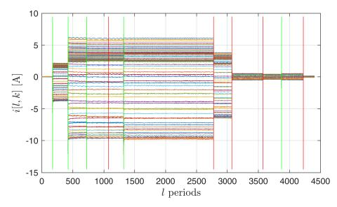
Figure 8.3: Different SSts of the FIT-PS waveform. The off events are marked red while on events are marked with green line.
