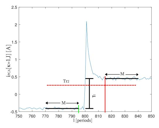
Figure 7.9: Second stage of the event detection. The difference before and after the suspected event is calculated. Modified from [143].
