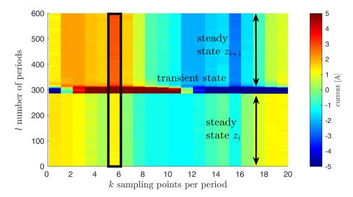
Figure 7.1: Event detection applied on FIT-PS
