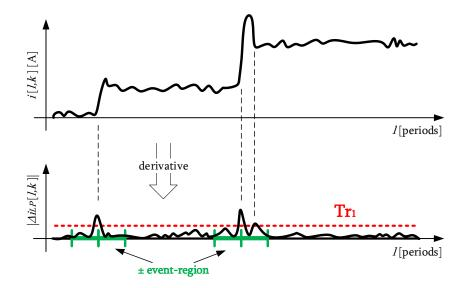
Figure 7.2: First stage of the event detection. The derivative is calculated from each dimension k of the FIT-PS concerted current signal over the periods l.
