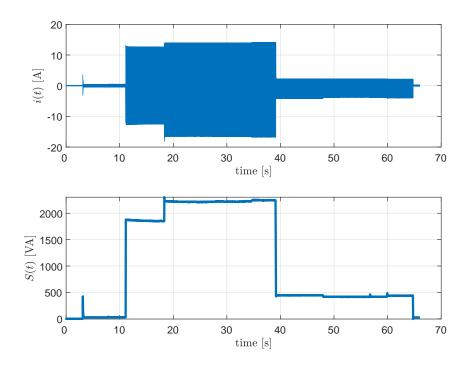
Figure 2.5: Comparison of the periodical, the original current signal (i(t)) to the non-periodical complex power (S) signal form
