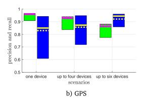
Figure 7.16: Results of the test measurements of the HELD1 dataset achieved with the parameters from 100 training iterations of the GPS or ten training parameters of SA. Recall: green, precision: blue; corresponding result to the best training iteration are marked pink respectively yellow with a dotted line; the median is marked with a solid line.
