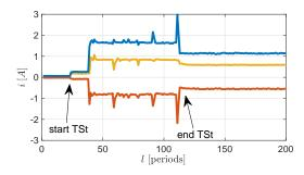
Figure 7.12: Envelope of a fluorescent lamp; maximum of the envelope  $i_{env}[l,1]$  (orange), minimum of the envelope  $i_{env}[l, 2]$  (red), absolute difference  $i_{envD}$  (blue).
