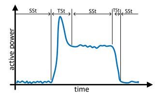
Figure 8.1: SSt and TSt illustrated on a active power waveform.
