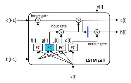
Figure 9.8: Structure of a LSTM cell
