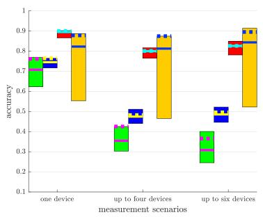
Figure 9.29: Accuracy of a FFNN using P and Q (green); P, Q, and HARs (blue); FIT-PS (red); LSTM net using FIT-PS (orange). The dotted lines represent the accuracy using the best initialization setting derived from the validation data. The solid lines represent the median of the accuracy of the test data.[68]
