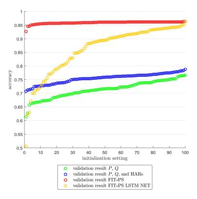
Figure 9.27: Results of a FFNN using different features for the validation data 0003, 0116, 0201. The accuracy is calculated by 100 iterations with different initialization settings and different number of neurons.[68]
