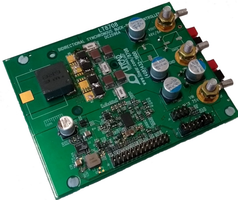
Figure 69: LT8708 Custom evaluation board (DC2596A)
