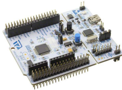
Figure 76: ST Nucleo-STM32L476RG with debug interface (right side) [103]
