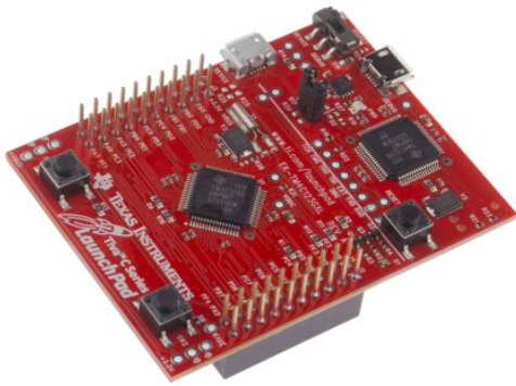
Figure 75: TI Tiva C-Series LaunchPad with debug interface (right side) [102]
