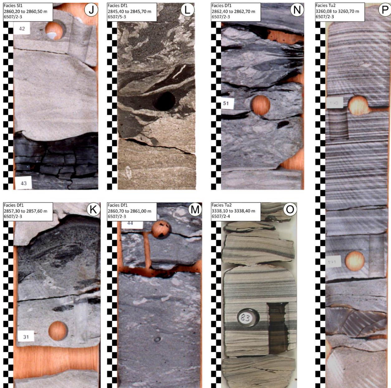
Fig. 3.5 (continued): ... and flame structures (J). Facies Df1 consists of muddy sandstones to sandy mudstones containing mudstone clasts, sand injectites and pseudonodules (K, L, M, N). Facies Tu2 consists of alternating fine to very fine-grained sandstone laminae (<1 mm up to 2 cm) with finer siltstone to mudstone laminae (<1 mm up to 2 cm). Tu2 is a well-structured very fine to fine-grained sandstone grading upwards into mudstones of facies O1. Laminations are parallel to sinusoidal (O, P, Q, R, S, T), and supercritical climbing-ripples ( sensu Storms et al. (1999) ) are also commonly observed (R, S, T, U) ...
