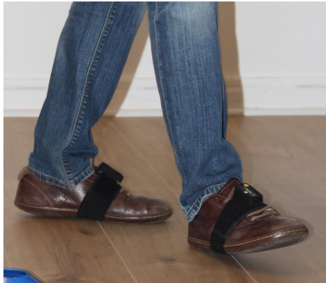
Figure S1: Placement of foot-worn inertial Physilog® sensors
