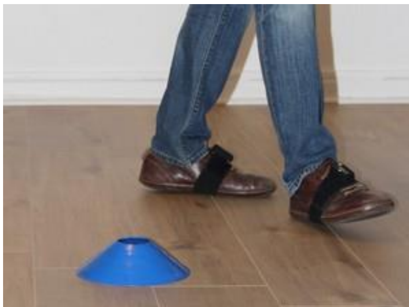
Figure 1. Picture showing the placement of the two foot-worn inertial sensors
