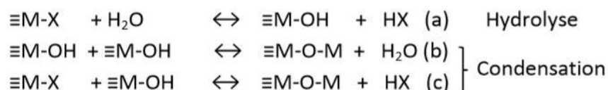
Figure 1. Equation of sol-gel process reactions [2] .
