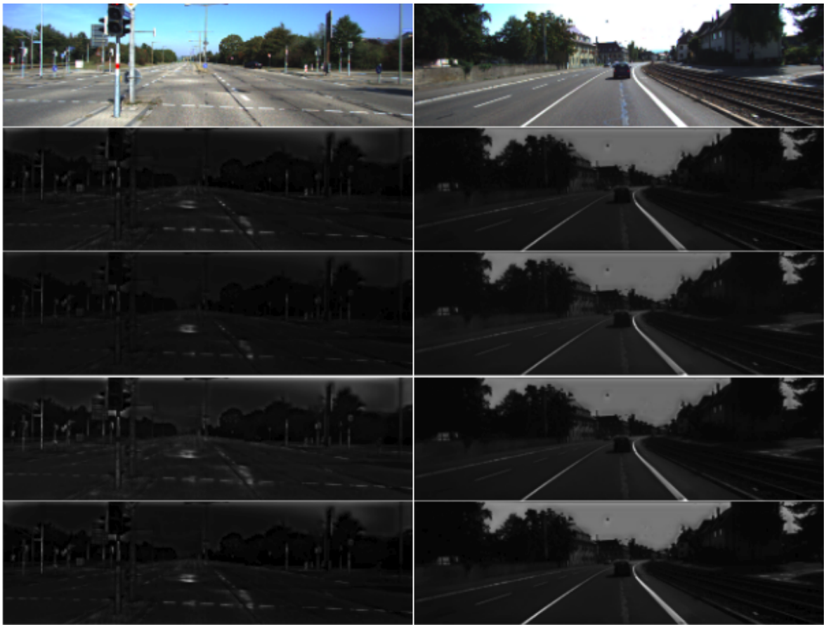
Figure C.2: Examples of generated polarimetric images from the KITTI dataset. From top to bottom, original image, I_0 , I_{45} , I_{90} and I_{135} .
