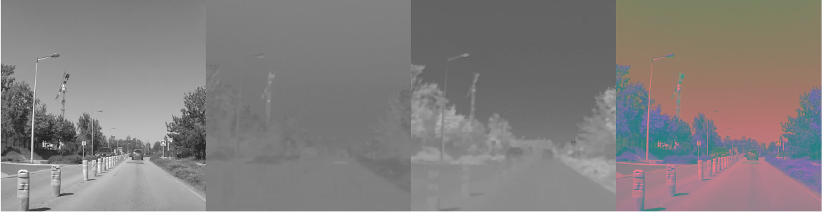
Figure 1.12: Example of a CIE Lab image and its channels decomposition. From left to right, the luminance, the offset towards the cyan (-a) \rightarrow magenta (+a) axis, the offset towards the blue (-b) \rightarrow yellow (+b) axis and their concatenation to constitute a CIE Lab image.
