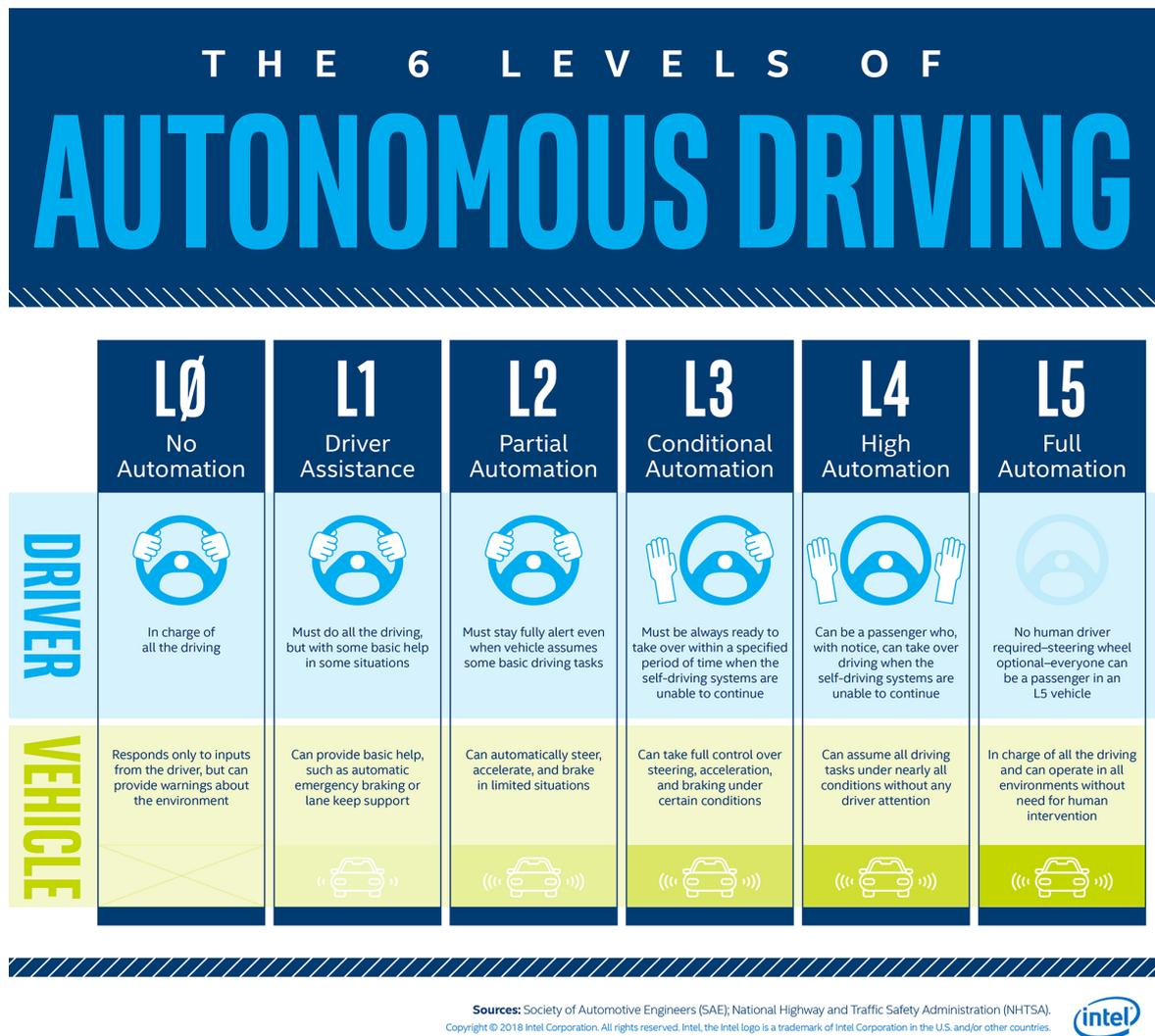
Figure 2: The six automation levels of autonomous systems.
