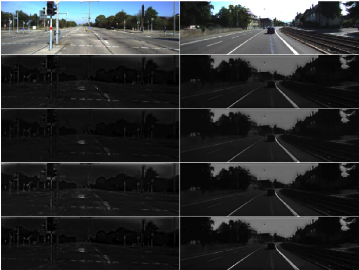
Figure C.2: Examples of generated polarimetric images from the KITTI dataset. From top to bottom, original image,  $I_0$ ,  $I_{45}$ ,  $I_{90}$  and  $I_{135}$ .
