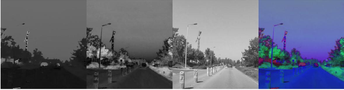
Figure 1.10: Example of an HSV image and its channels decomposition. From left to right, the hue, the saturation, the value and their concatenation to constitute an HSV image.
