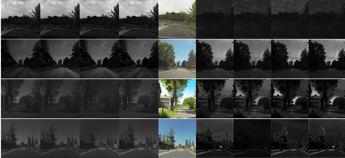
Figure 4.17: Examples of polarimetric image generation. From left to right:  $I_0$ ,  $I_{45}$ ,  $I_{90}$  and  $I_{135}$  ground truth, RGB image and  $I_0$ ,  $I_{45}$ ,  $I_{90}$  and  $I_{135}$  generated from RGB image.
