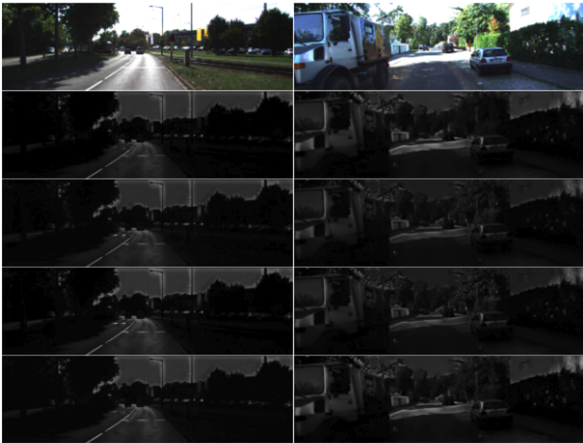
Figure C.1: Examples of generated polarimetric images from the KITTI dataset. From top to bottom, original image, I_0 , I_{45} , I_{90} and I_{135} .
