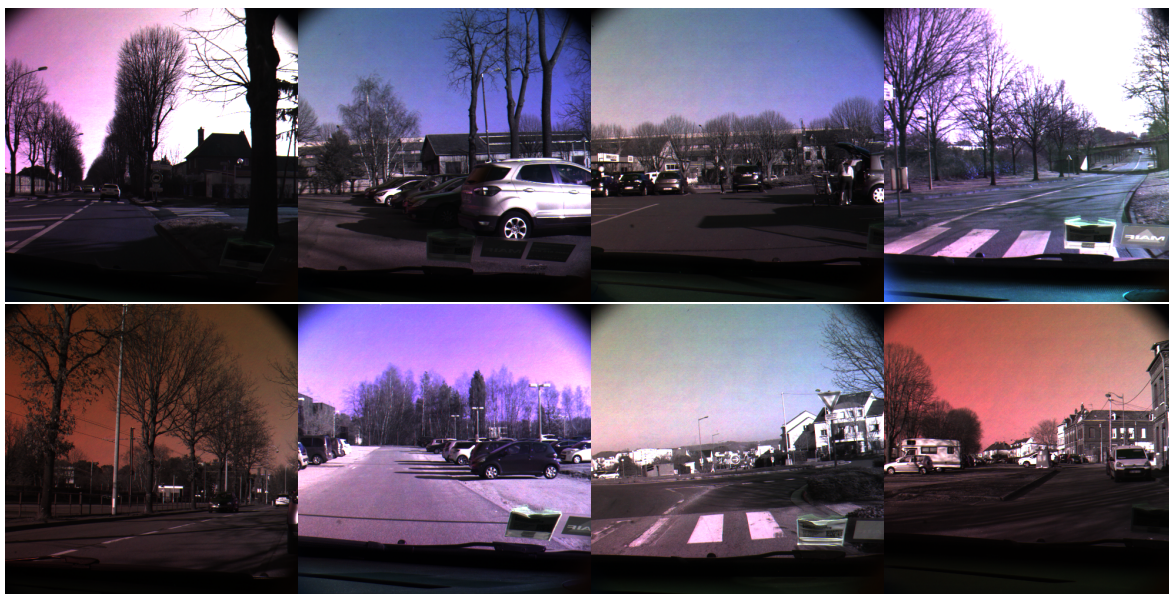
Figure 4.2: Examples of road scenes captured during the polarimetric acquisition campaign. Here (I_0, I_{45}, I_{90}) are placed as the (R, G, B) format.
