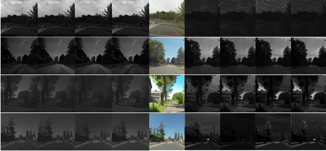
Figure 4.17: Examples of polarimetric image generation. From left to right: I_0 , I_{45} , I_{90} and I_{135} ground truth, RGB image and I_0 , I_{45} , I_{90} and I_{135} generated from RGB image.
