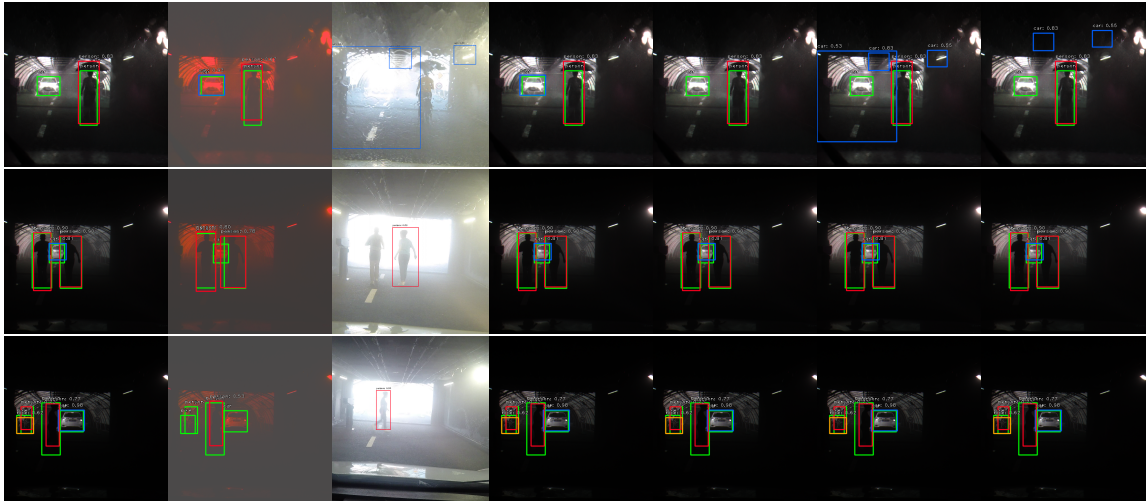
Figure 6.10: Detection results in several adverse weather conditions. From top to bottom: tropical rain and fog with respectively 35m and 60m visibility. From left to right: I , S , RGB, I + S (Double soft-NMS), I + S (OR filter), I+RGB (Double soft-NMS) and I+RGB (OR filter). Bounding boxes in green, blue, red and orange denote respectively the ground truth, car, person and bike detection.
