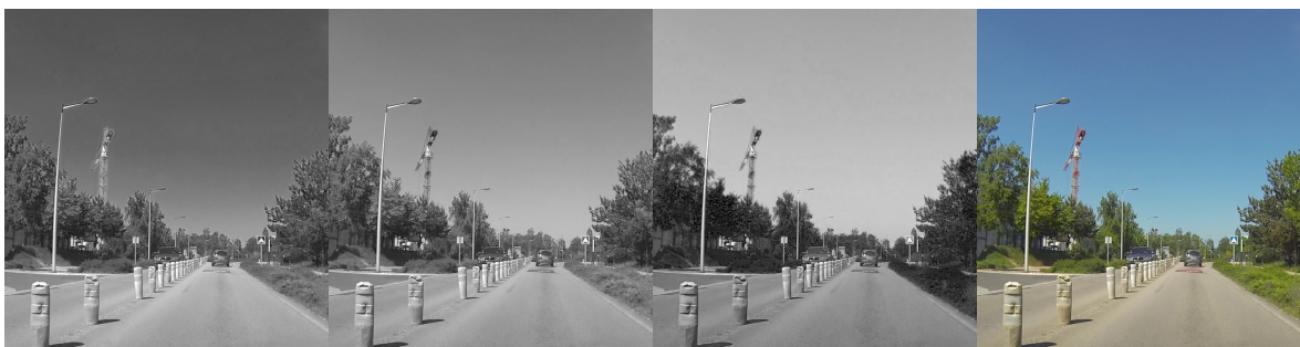
Figure 1.8: Example of an RGB image and its channels decomposition. From left to right, the red channel, the green channel, the blue channel and their concatenation to constitute an RGB image.
