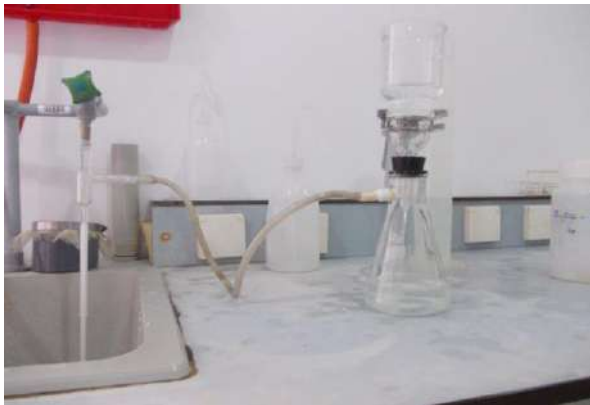
Figure 12. Water filtration device.
