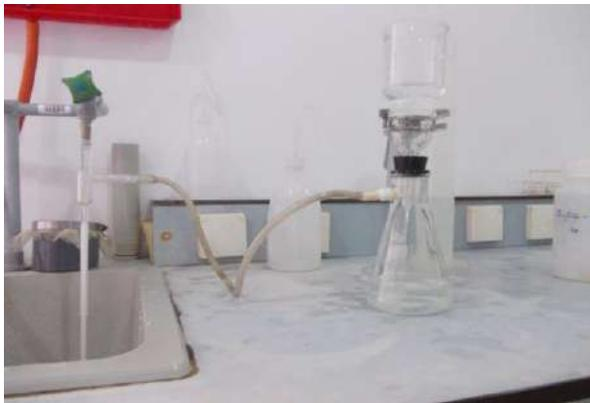
**Figure 12. Water filtration device.**
