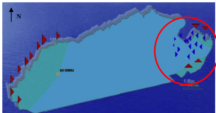
Figure 4. Water circulation in the North Lagoon of Tunis before restoration
