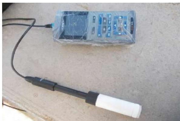
**Figure 9. Conductivity meter.**
