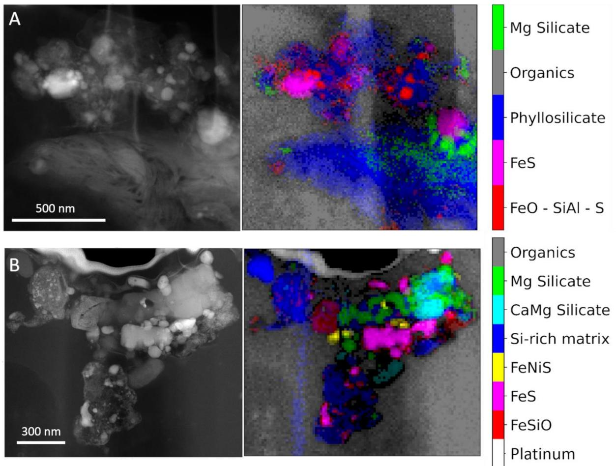
Figure 4-24: (left) High angle annular dark field (HAADF) images and (right) False color images corresponding to the map of the different phases identified by Principal Component Analysis of the EDX hyperspectral maps.. (A) Phyllosilicate-like phase (fibrous phase) decorated with a mineral assemblage. (B) Mineral assemblage located at the border of a vesicle. Both assemblages are embedded in the organic matter.
