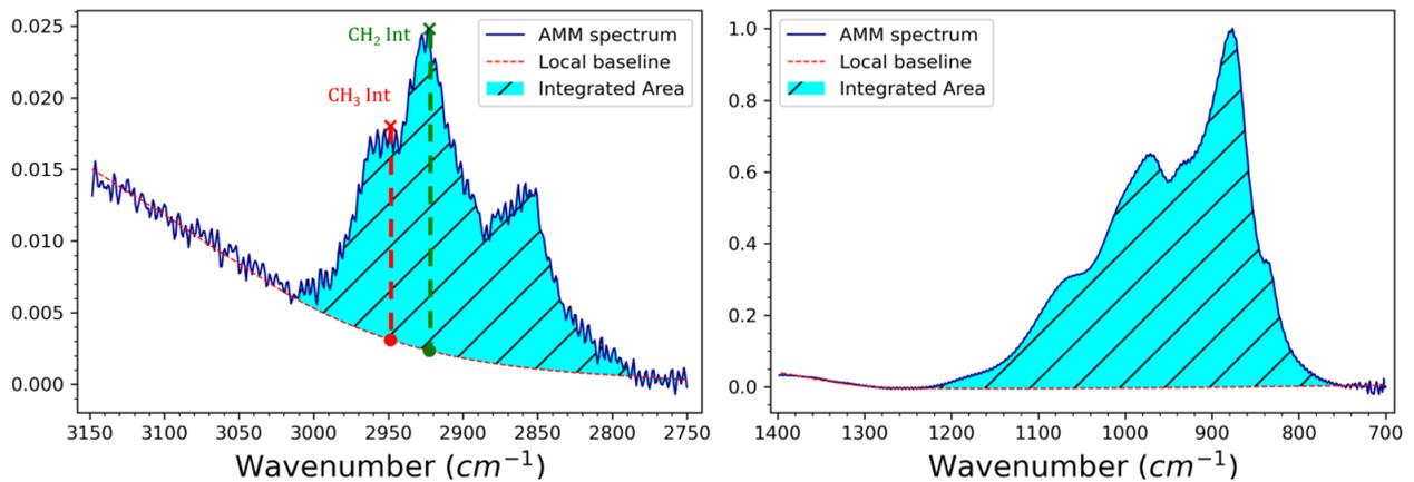
Figure 2-14: Example of area calculation under the aliphatic (left) and silicate(right) absorption peaks. The vertical lines on the left corresponds to the value of the CH<sub>2</sub> and CH<sub>3</sub> direct intensity measurements.
