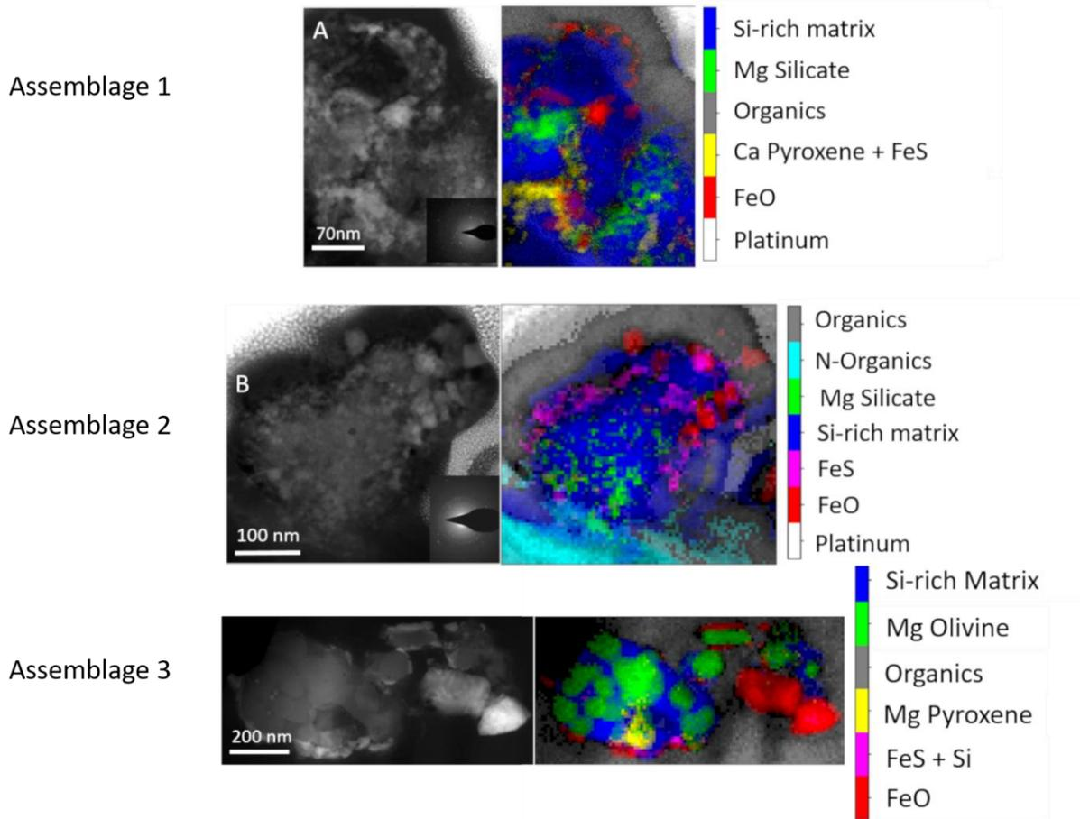
Figure 8-1: (left) High Angle Annular Dark Field (HAADF) image of 3 mineral assemblages in DC06-308. (right) False color images corresponding to the EDX maps of the different phases identified by Principal Component Analysis (PCA). The phases are ordered by decreasing number of counts in the respective spectra
