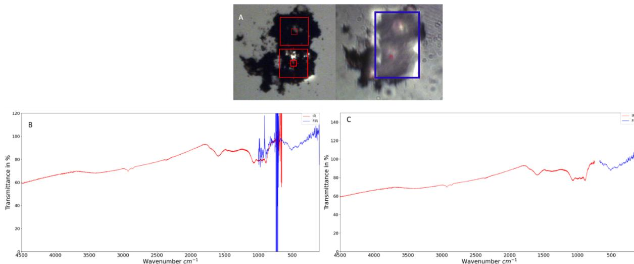
Figure 2-12: (A) Areas covered by the mid-IR measurement (red squares, left) and the far IR measurement (blue square, right). In order to cover the same area, two mid-IR spectra must be averaged. (B) Merged spectrum of the sample before cropping and scaling with the MIR part in red and the FIR part in blue (C) Final version of the total spectrum with both measurements merged and corrected.
