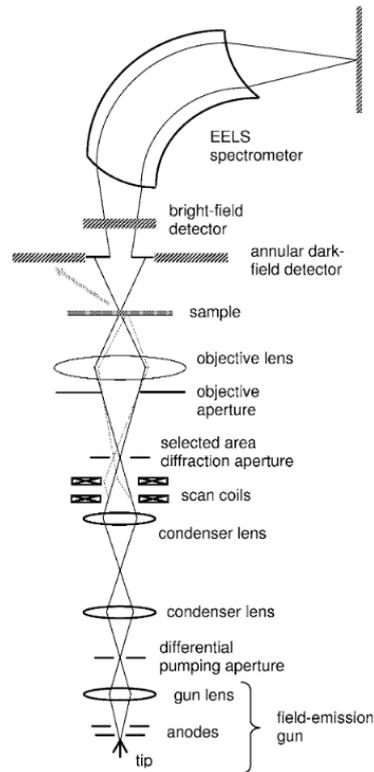
Figure 2-9: Diagram of the different component of a Scanning Transmission Electronic Microscope. Image from (Nellist, 2007)
