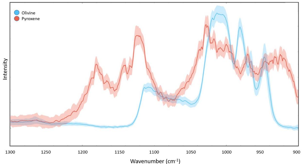
Figure 6-1: Comparison of pyroxene (red) and olivine (blue) absorption bands over the  $900\text{ cm}^{-1}$  –  $1300\text{ cm}^{-1}$  region for the polished micrometer-thick sample preparations. The light halo surrounding the different spectra represents the spectral variation for the averaged set of spectra.
