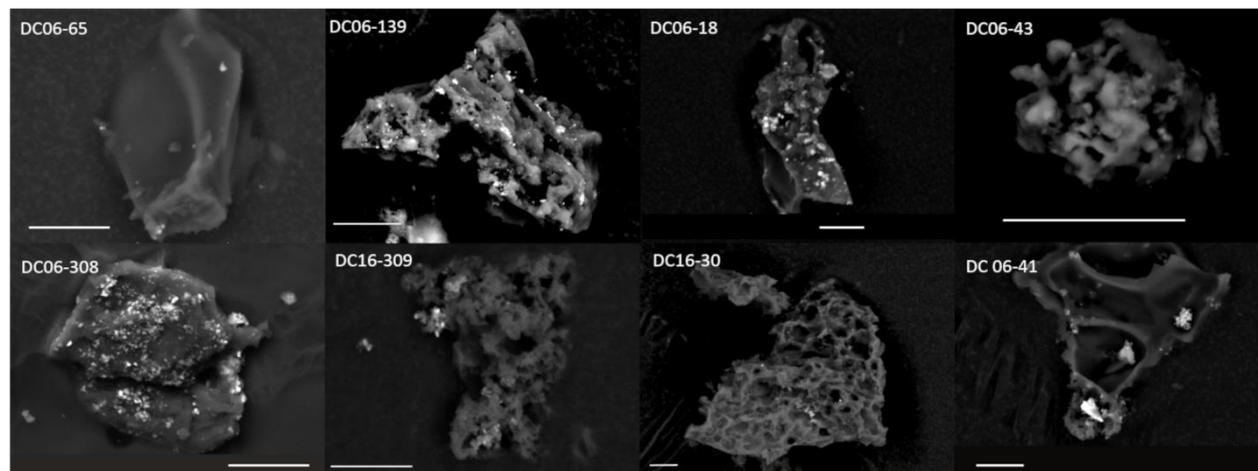
Figure 4-2: Back-scattered electron images of fragments of Ultracarbonaceous Antarctic Micrometeorites used for the analyses with STXM-XANES and STEM. Scale bar are 10 microns.
