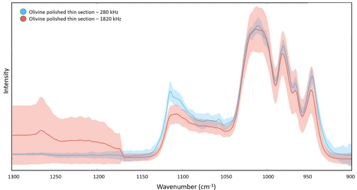
Figure 6-5: AFMIR spectra for olivine polished section at two laser frequencies. The light halo surrounding the different spectra represents the spectra variations for the averaged set of spectra.
