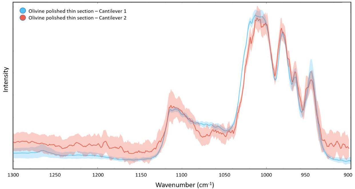
Figure 6-7: AFMIR spectra for olivine polished section with two different cantilever. The light halo surrounding the different spectra represents the spectra variations for the averaged set of spectra.
