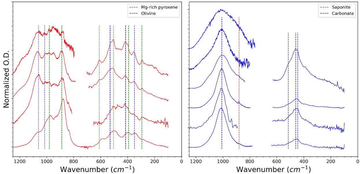
Figure 3-4: Z Zoom over the silicate absorption range of the IR spectrum in the different chondritic (right) and hydrated (left) AMMs. The main bands for Mg-rich pyroxene, olivine, saponite and carbonate are indicated in the spectra.
