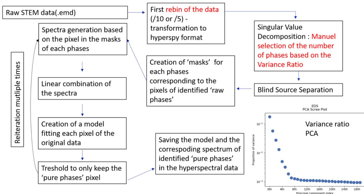
Figure 2-10: Workflow of the data processing method used to deconvolve hyperspectral data of STEM cartography.
