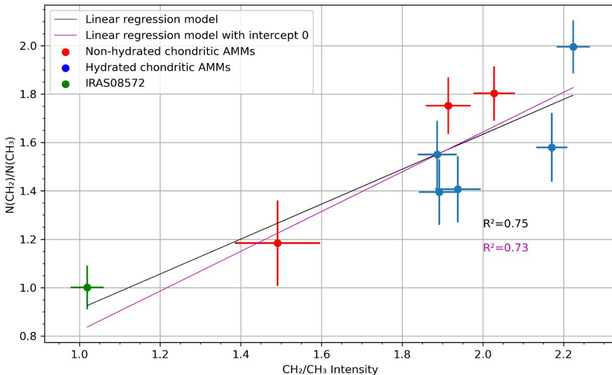
Figure 3-7: Measured  $\text{CH}_2/\text{CH}_3$  intensities compared to the  $\text{N}(\text{CH}_2)/\text{N}(\text{CH}_3)$  ratio extracted from Gaussian area calculation of  $\text{CH}_2$  and  $\text{CH}_3$  asymmetric modes. The two lines represent linear regression results with a fixed intercept at 0 (pink) and with no intercept fixed (black)
