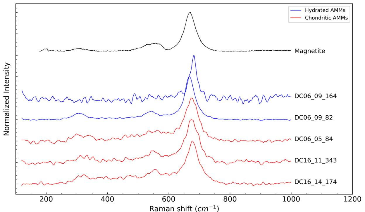
Figure 3-13: Spectra of both hydrated (blue) and chondritic (red) AMMs displaying the peak attributed to magnetite. The standard magnetite spectrum is displayed in black (Lyon Raman database: [www.geologie-lyon.fr/Raman](http://www.geologie-lyon.fr/Raman))
