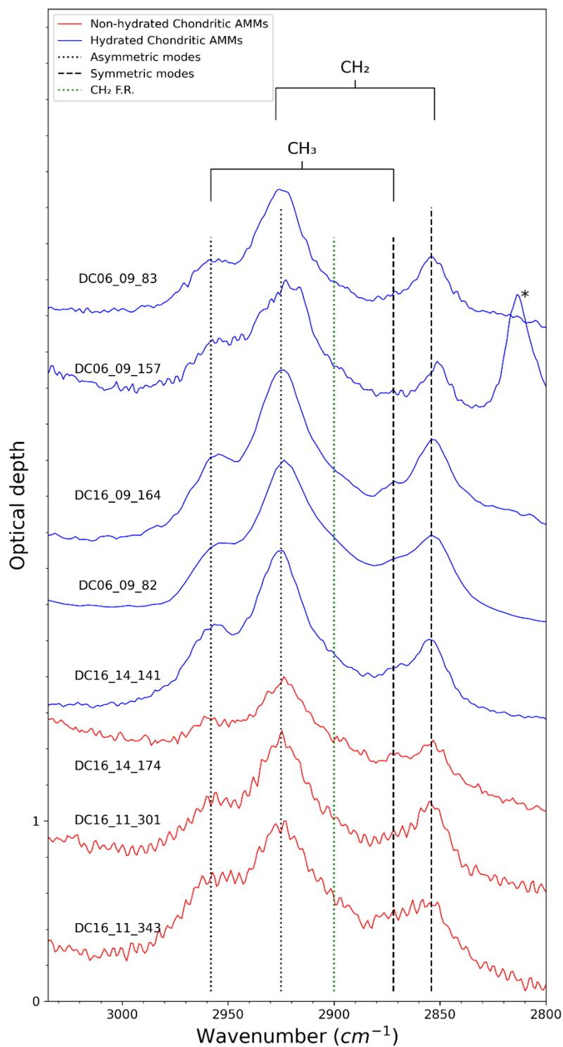
Figure 3-5: Zoom on the aliphatic absorptions region of the MIR spectra for the different AMMs. The spectra have been normalized to the asymmetric mode of  $\text{CH}_2$  and vertically shifted for clarity. AMMs DC 06\_06\_84 and DC 06\_11\_70 are not displayed because of their low aliphatic content.  $\text{CH}_2$  F. R. :  $\text{CH}_2$  Fermi resonance. \*The peak at  $2815\text{cm}^{-1}$  observed in DC06-09-157 has been characterized as contamination.
