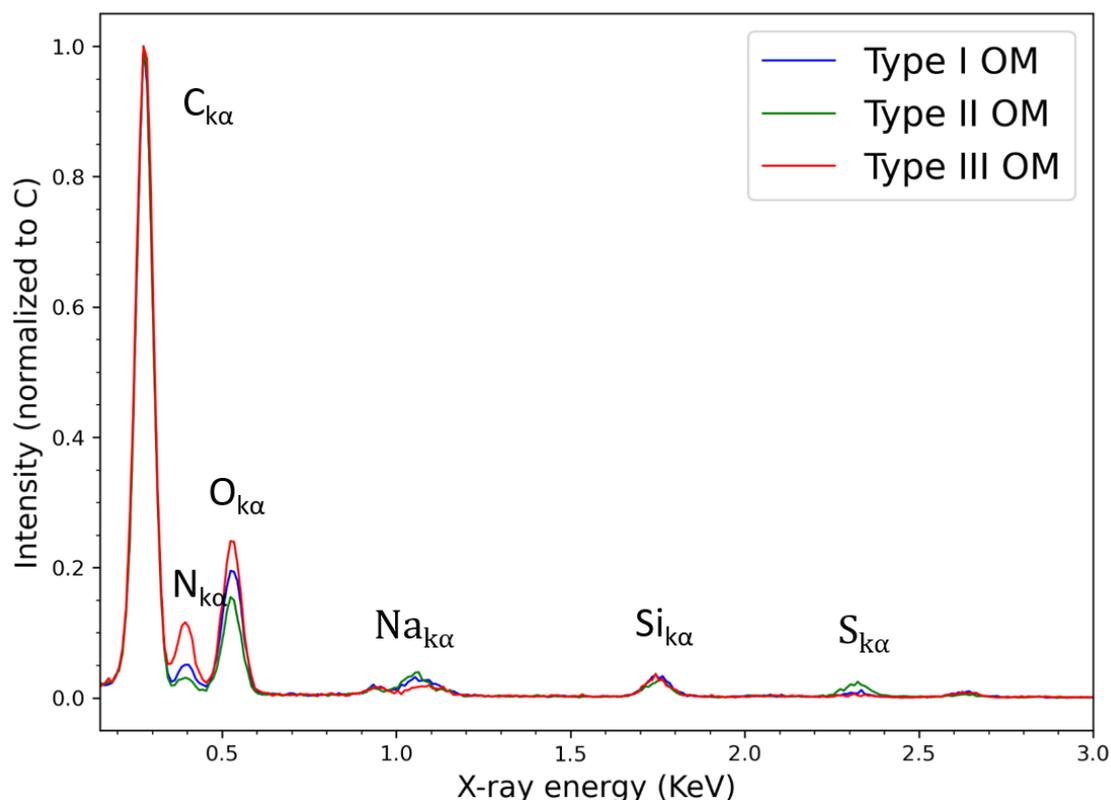
Figure 4-14: EDX spectra of the three types of organic matter in DC16-309. Each spectrum has been normalized to its maximum carbon intensity for easier comparison.
