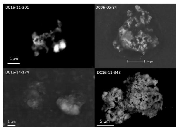
Figure 3-2: Back-scattered Electron images of the fragments of the 4 anhydrous chondritic AMMs studied in this work
