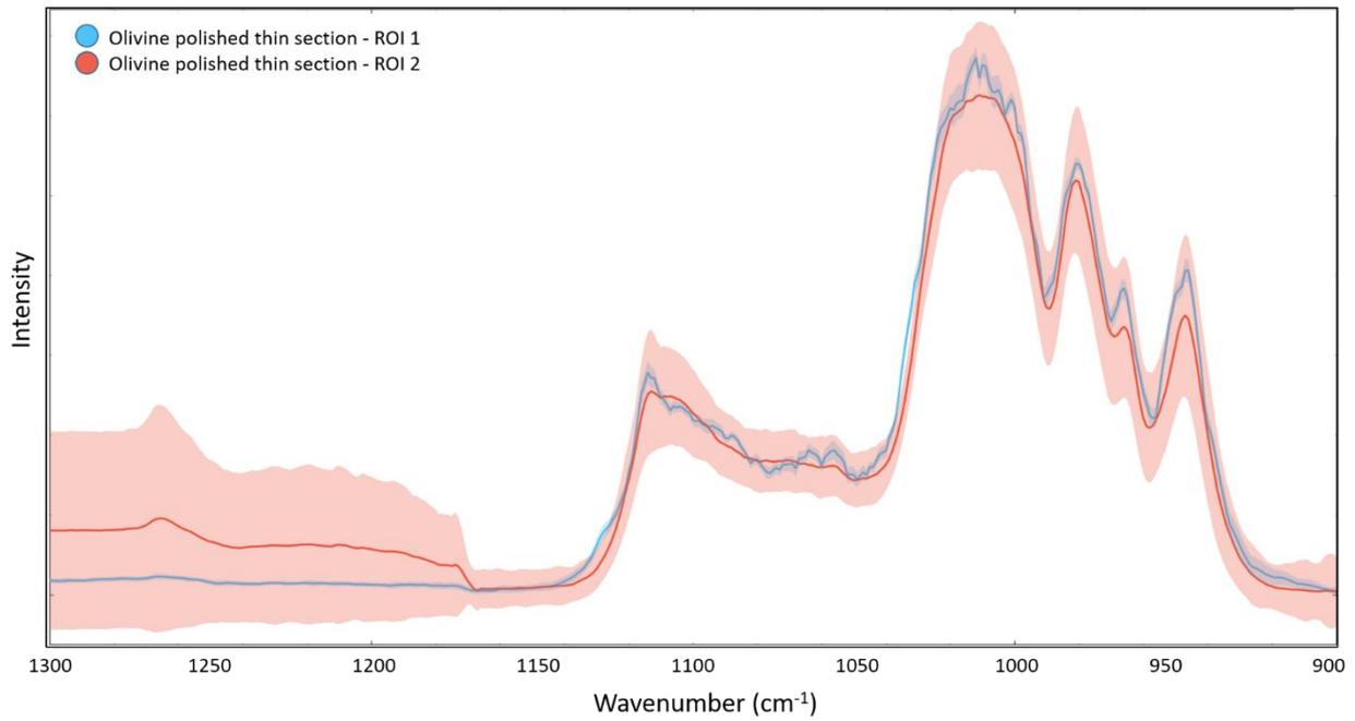
Figure 6-3: Comparison of the averaged spectra obtained for olivine polished thin section for two distinct regions of interest. Analyses were realized in similar analytical conditions. The light halo surrounding the different spectra represents the spectral variation for the averaged set of spectra.
