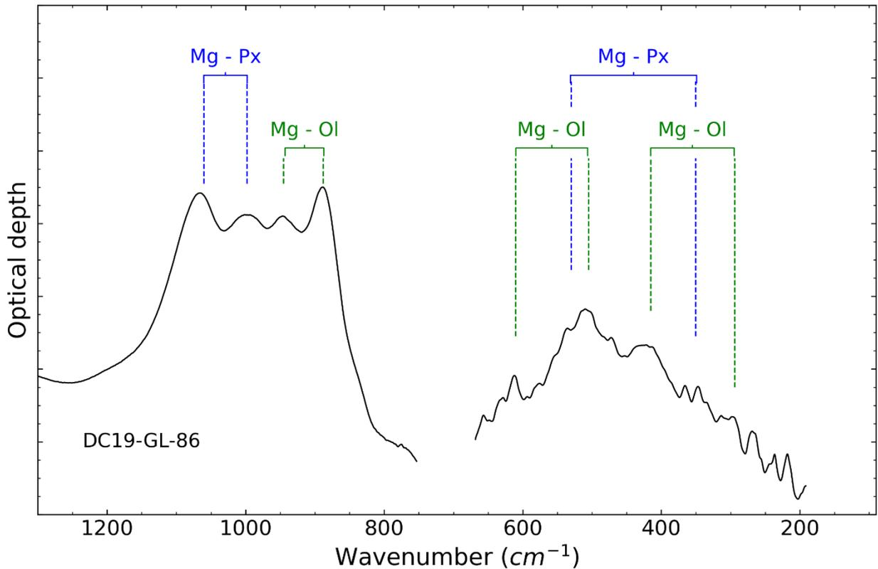
Figure 4-16: Zoom of the infrared spectrum over the 100  $cm^{-1}$ - 1200  $cm^{-1}$  absorption range for UCAMM DC19-86. The spectrum for DC16-98 is not displayed as it has no mineral-related absorption over the silicate range (see Figure 4-4).
