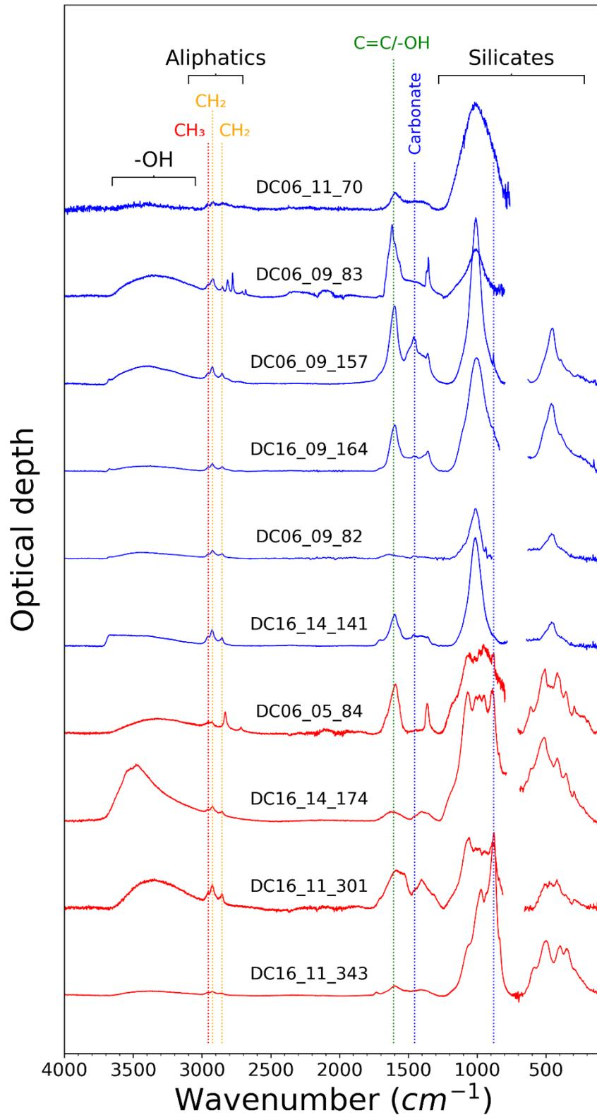
Figure 3-3: Merged far and mid infrared spectra (after baseline correction) of 10 AMMs from the Concordia collection collected during Antarctic expeditions in 2006 (DC06) and 2016 (DC16). Blue spectra correspond to hydrated chondritic AMMs containing phyllosilicates and red spectra correspond to non-hydrated chondritic AMMs.
