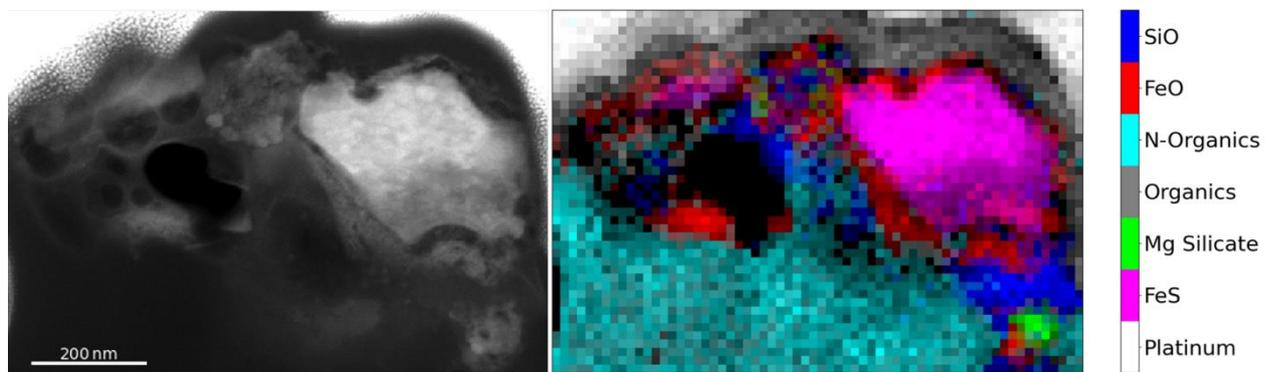
Figure 4-22: (left) High Angle Annular Dark Field (HAADF) image of a complex mineral assemblages in DC06-308 located on the top edge of the FIB section. (right) False color images corresponding to the EDX maps of the different phases identified by Principal Component Analysis (PCA). The phases are ordered by decreasing number of counts in the respective spectra.
