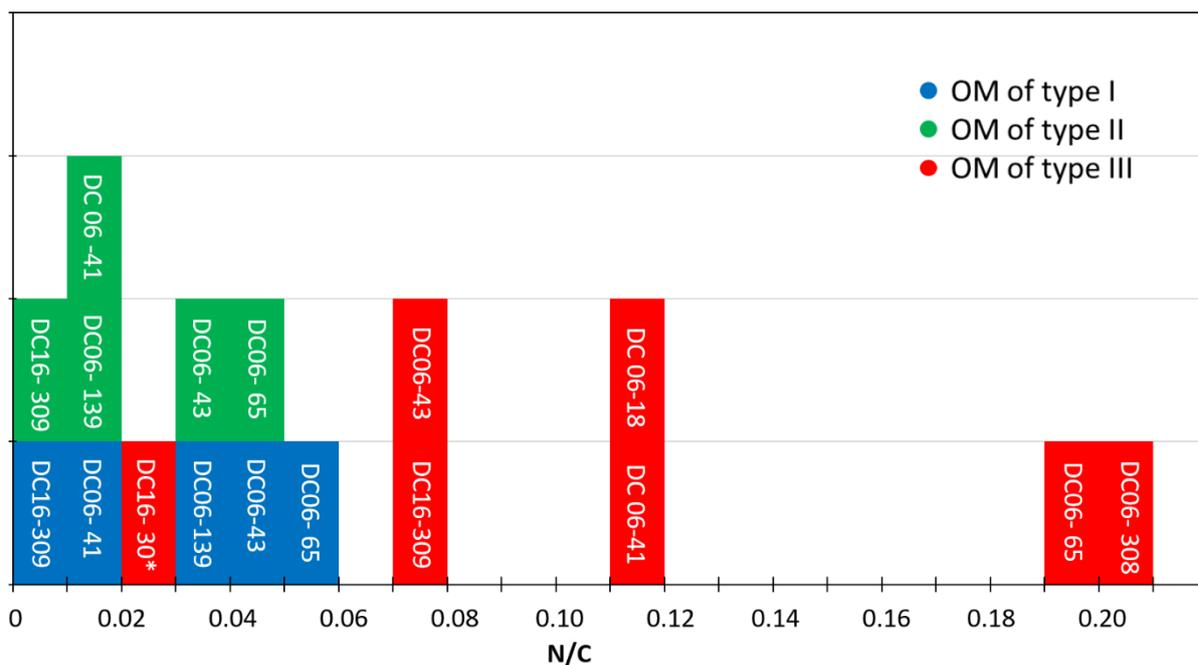
Figure 5-4: Histogram of the distribution of N/C atomic ratios for the 3 different organic matter types found in each UCAMM presented in this study. \*The low N/C atomic ratio for type III OM in DC16-30 could be explained by a higher heating during atmospheric entry, see section 5.3
