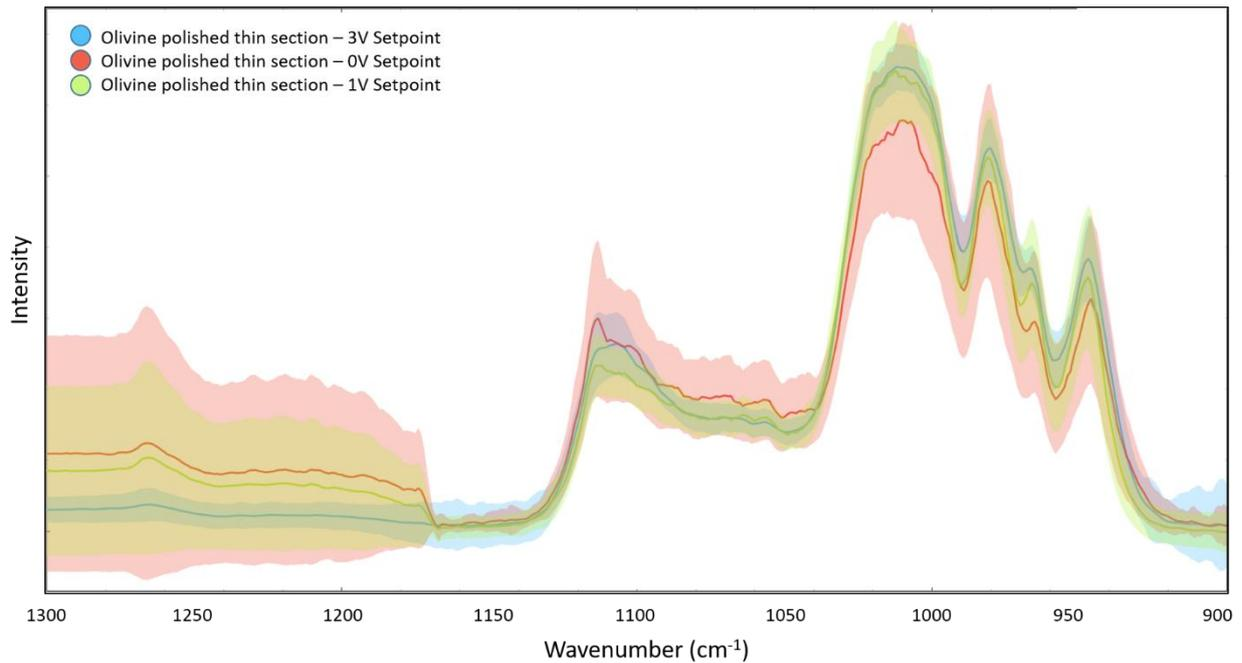
Figure 6-6: AFMIR spectra for olivine polished section at three cantilever setpoints. The light halo surrounding the different spectra represents the spectra variations for the averaged set of spectra.
