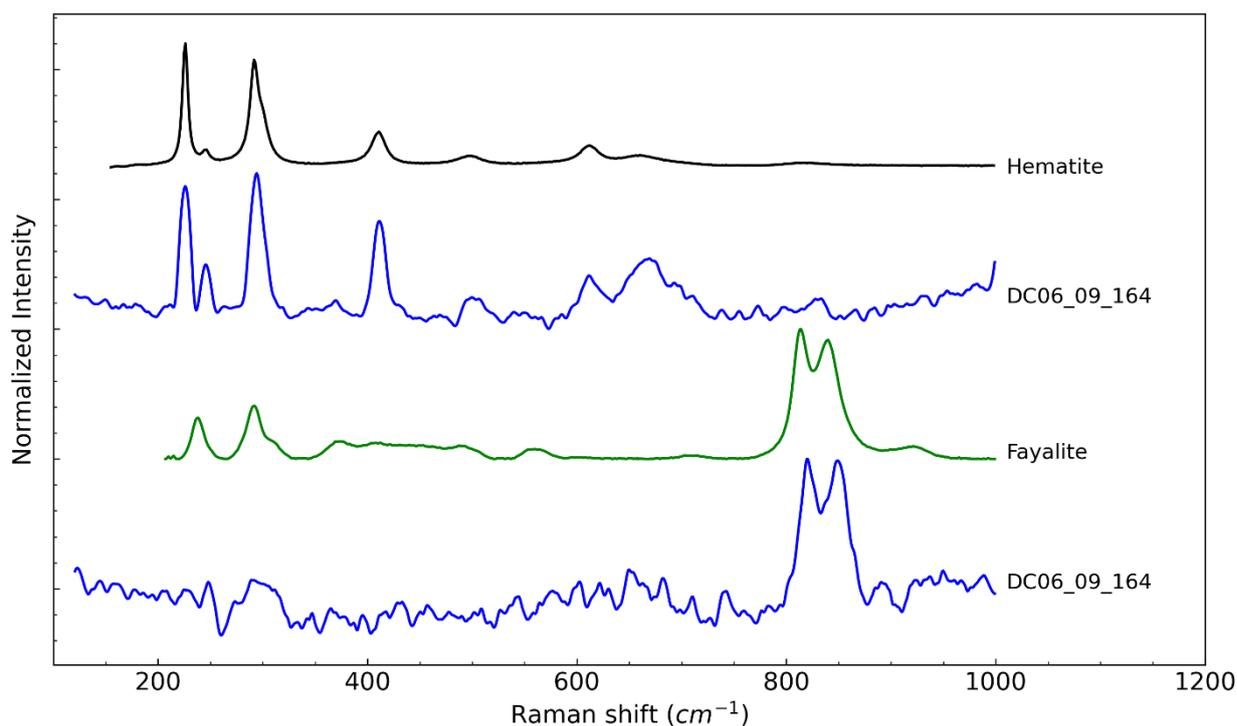
Figure 3-14: Punctual mineral phases corresponding to fayalite and hematite found in DC06-09-164. Pure mineral spectra are from RRUF (<https://rruff.info/>) and Lyon spectral database ([www.geologie-lyon.fr/Raman](http://www.geologie-lyon.fr/Raman)).
