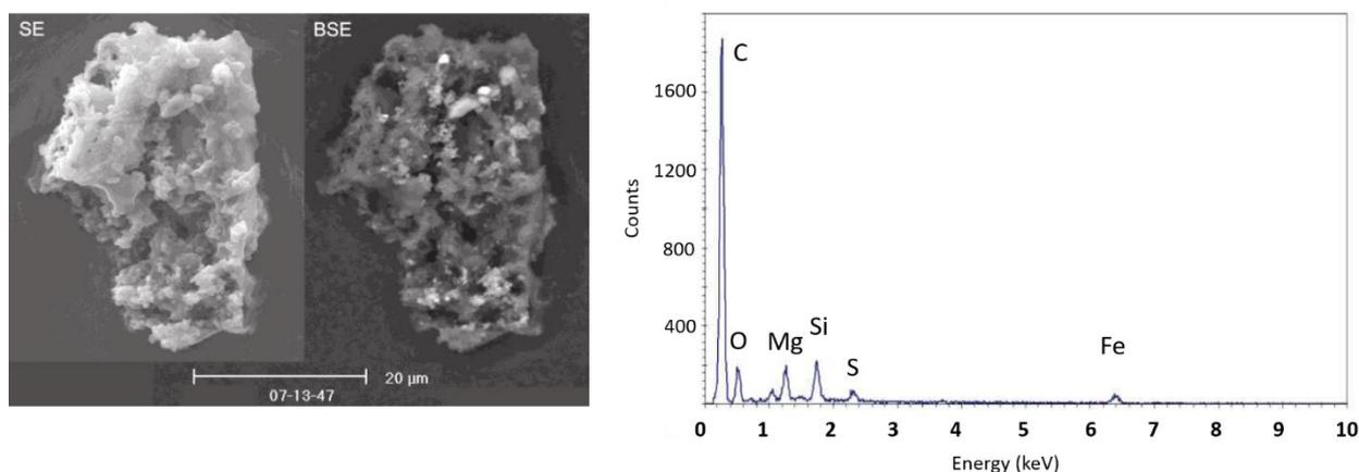
Figure 2-3: (left) Secondary Electron (SE) and Back-Scattered Electron(BSE) images of the UCAMM DC06-09-119. (right) corresponding EDX spectrum with the dominant  $K\alpha$  emission of carbon for UCAMMs.
