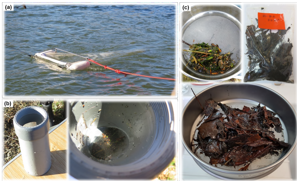
Figure 2.6: Water surface sampling with (a) manta trawl equipped with (b) a removal cod-end. Samples were filtered in the field (c) using a 500 µm sieve and stored in a plastic bag before processing in the laboratory.
