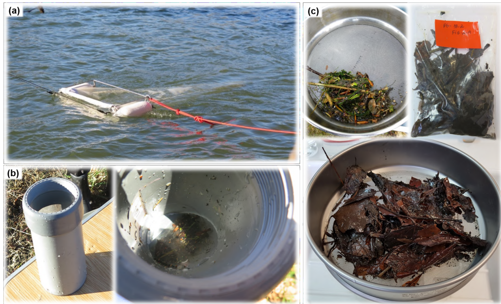
Figure 2.6: Water surface sampling with (a) manta trawl equipped with (b) a removal cod-end. Samples were filtered in the field (c) using a 500 \mu\text{m} sieve and stored in a plastic bag before processing in the laboratory.
