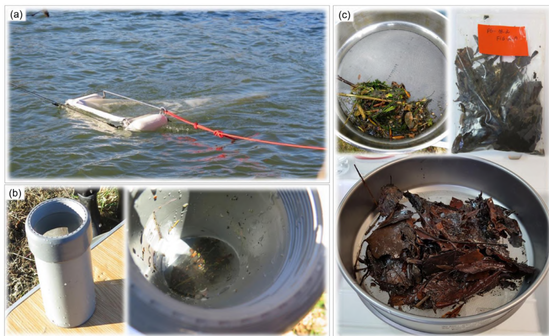
Fig. 2. Sample collection in the field with (a) Manta trawl equipped with (b) a removal cod-end. Samples are filtered in the field (c) using a 500 \mu\text{m} sieve and stored in a plastic bag before processing in the laboratory.
