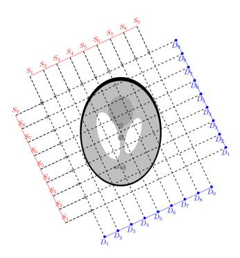
**Figure 1.5** – Functioning principle of computed tomography. The arrays of sources and detectors are respectively represented in red and blue at two different times during acquisition. In fact, the system needs to rotate to perform a full data acquisition. The dashed lines represent the corresponding X-ray paths.
