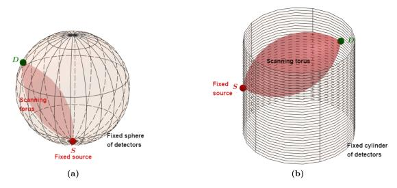
**Figure 5.2** – Possible extensions of CCST in three dimensions. (a) SCST with detectors on a sphere and (b) CylCST with detectors on a cylinder.
