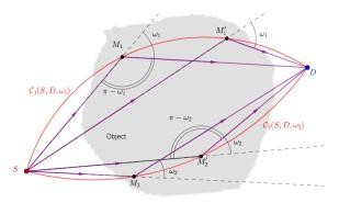
Figure 1.6 – General functioning principle of a CST system. Photons are emitted by source S (in red), interact at sites M, and are recorded at site D (in blue). When a photon is detected carrying an energy  $E(\omega_1)$  (resp.  $E(\omega_2)$ ), the possible interaction sites lie on the upper (resp. lower) circle are which subtends the angle  $(\pi - \omega_1)$  (resp.  $(\pi - \omega_2)$ ).
