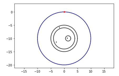
Figure A.2 – Setup of the system and the phantom. The source is represented by a red star, and detectors are depicted alternatively in black and blue. The numbers 1, 2 and 3 refers to the number of the considered circle according to Table A.1
