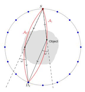
Figure 3.1 – Presentation of CCST. The dotted line represents the ring containing point-like detectors in blue. We find also the source, in red, on the ring. For an arbitrary detector  $D_k$  and a scattering angle  $\omega$ , the corresponding double scanning arc  $A_1 \cup A_2$  is showed in red.
