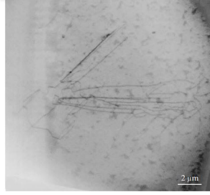
FIGURE 1.7: Transmission electron microscopy (TEM) picture of dislocations in a steel (Cordier et al., 2014).
