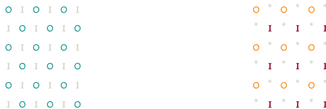
(a) The first detected feature is the diagonal offset. It decides whether the pixel was sampled in green. (b) The second feature is the evenness of the line/column of the pixel on the main diagonal. It decides whether the pixel was originally sampled in red or in blue.
