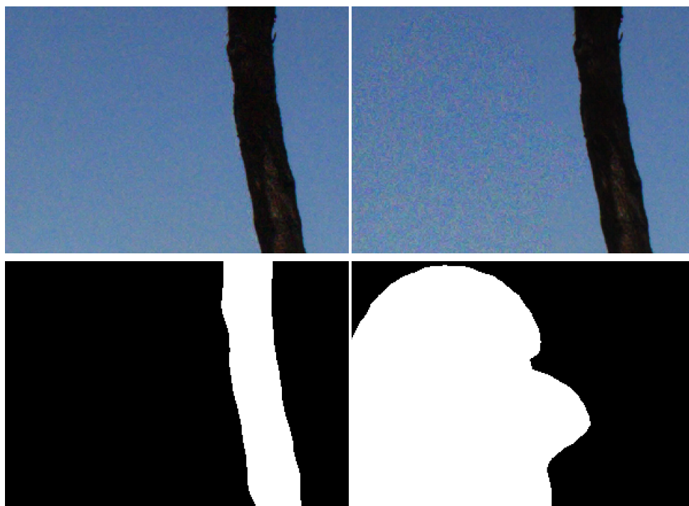
Figure 1.4: Details of the same image with forgeries made using the two masks. On the left, the endomask coincides with the image’s structure, here a tree. The forgery is less conspicuous than on the right where the exomask is in the sky, where the borders do not coincide with the images’ content.
