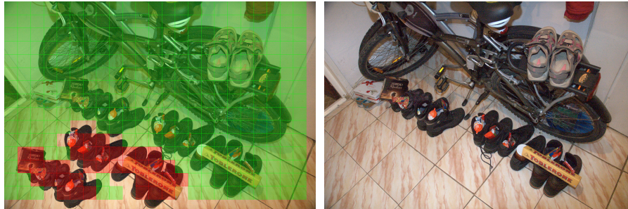
(a) Found forged regions are in red, and regions where the exact CFA grid was identified are in green
