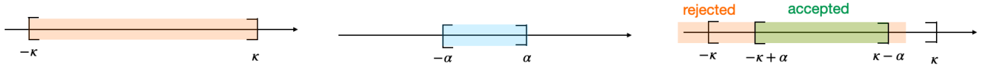
Figure 3.6: Graphical intuition for computing P[\|\mathbf{s}_1\mathbf{c} + \mathbf{y}_1\|_\infty > \kappa - \alpha] = P[\|\mathbf{s}_2\mathbf{c} + \mathbf{y}_2\|_\infty] . Without loss of generality, we only consider \mathbf{y}_1, \mathbf{s}_1, \mathbf{z}_1 . To the left, we represent the distribution for the coefficients of \mathbf{y}_1 . In the middle, we represent the possible values for the coefficients of \mathbf{s}_1\mathbf{c} . To the right, the distribution of \mathbf{y}_i is shifted by \mathbf{s}_i\mathbf{c} to obtain the distribution of \mathbf{z}_1 . The accepted (resp. rejected) \mathbf{z}_1 are in green (resp. in orange). We see that, no matter the shift of \mathbf{s}_i\mathbf{c} , the fraction of rejected coefficients will stay = \frac{2\alpha}{2\kappa+1} .
