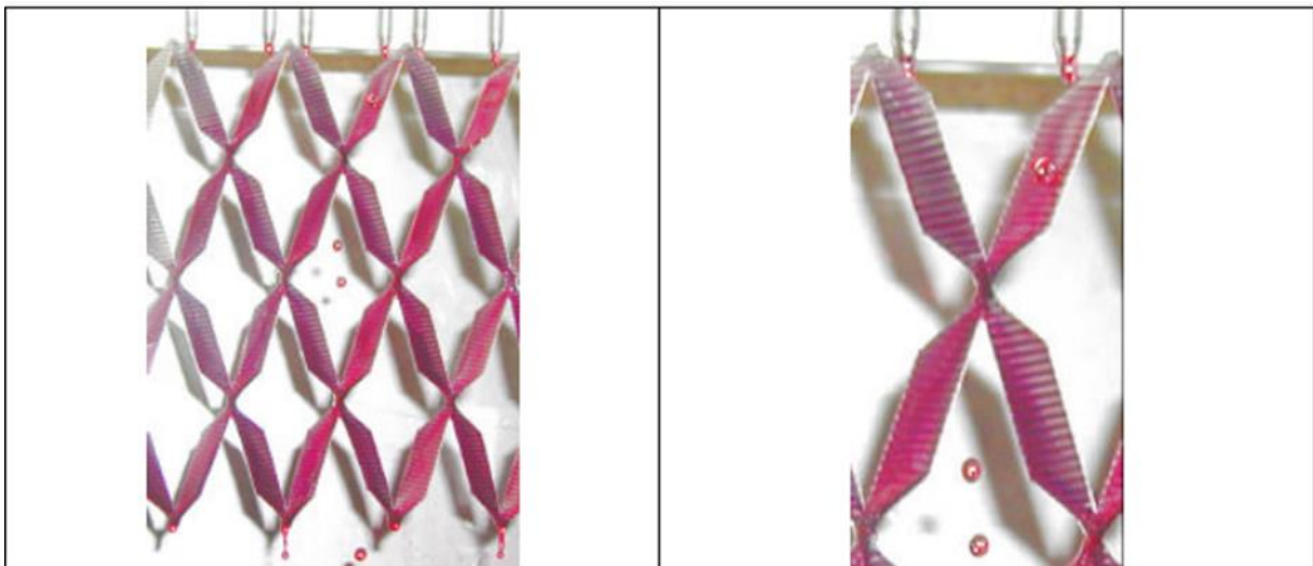
Figure 1-12: Liquid flow pattern for chlorobenzene – ethylbenzene 50% (16.9 ml/min.plate) with capillaries or irrigation points 10 mm distance apart from the plates surfaces 30
