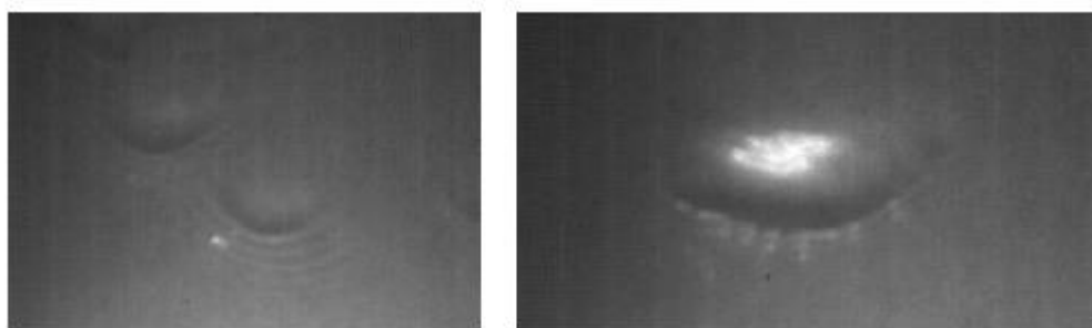
Figure 1-22: Visualizations of different wave forms for moderate gas backflow velocities ( Re_L = 56 ; Re_G = 11200 ): U-shaped waves (left) and pocket waves (right).
