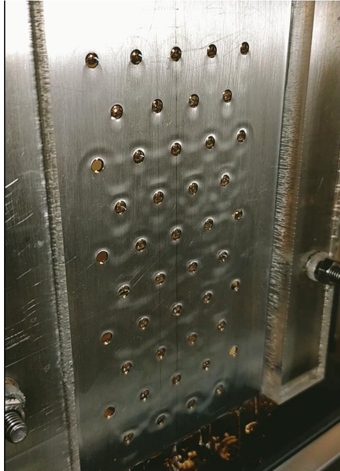
Figure S4.10. Liquid film pattern on a staggered array of perforations at Re = 35 \cong Re_{cr} when all perforations are in curtain mode. Plate thickness t = 1 mm, perforation diameter d = 4 mm and spacing s = 14 mm. Full view of the back of the plate.
