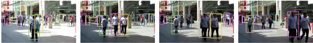
Figure 3.13: RNN Tracking output on the MOTChallenge sequence. The colour of each bounding box indicates the person identity (Milan et al., 2016).
