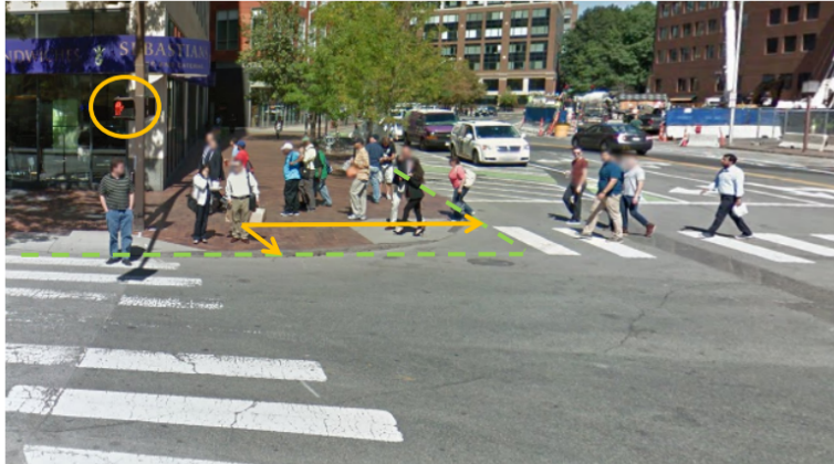
Figure 1.6: Example intersection scenario. Dashed green line denotes a rectangular approximation to the curbside in view. Orange arrows denote relative distance of a pedestrian from the two curbsides, which can indicate pedestrian intention. Pedestrian traffic light status is highlighted in orange, which also influences pedestrian movement (Habibi et al., 2018)
