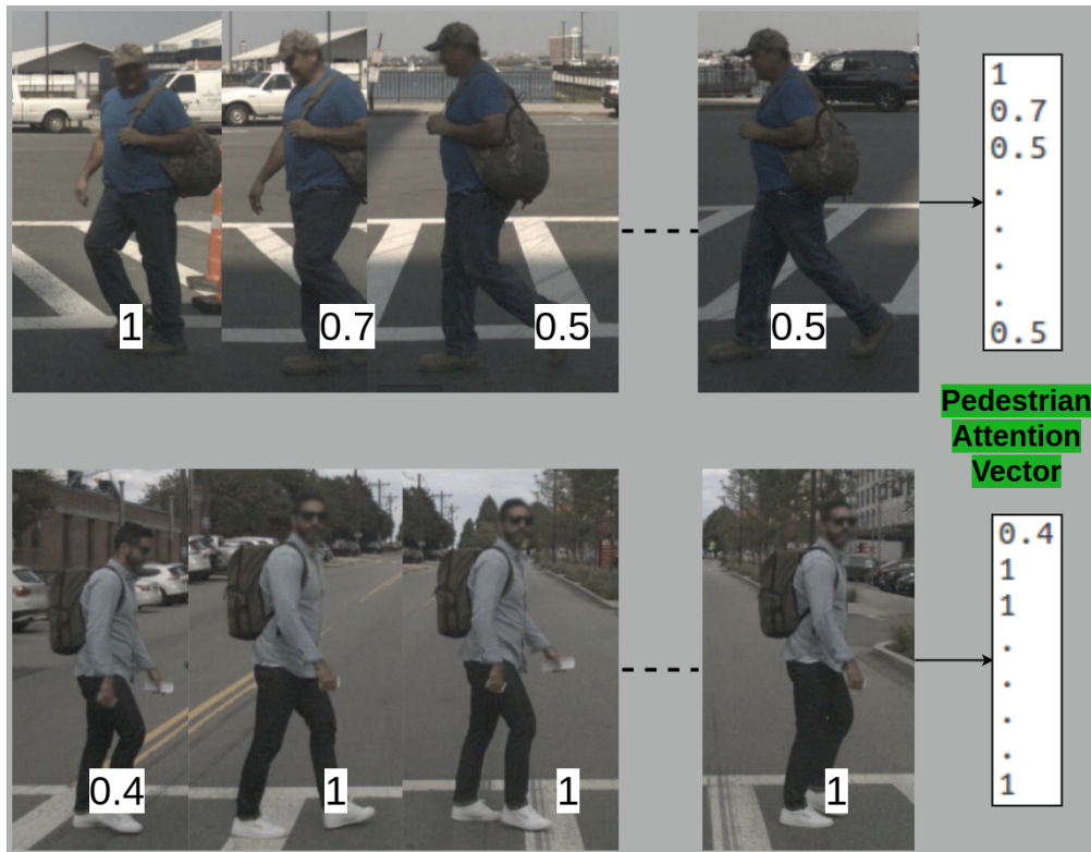
Figure 6.5: Pedestrian images used as visual input to annotate the Pedestrian Attention Vector
