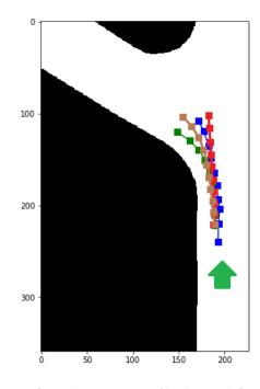
Figure 5.6: Comparison of trajectory prediction with classical methods: Green is ground truth, red is constant velocity, brown is constant curvature and blue is mapmask based prediction. The green arrows in the images show the direction of motion of the ego-vehicle
