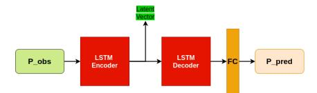
Figure 4.3: A basic LSTM encoder-decoder trajectory prediction model.
