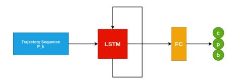
**Figure 4.4:** System Architecture for the LSTM based Trajectory Classification. (Class of interest are cars, pedestrians and bicycles, represented by scores c, p and b)
