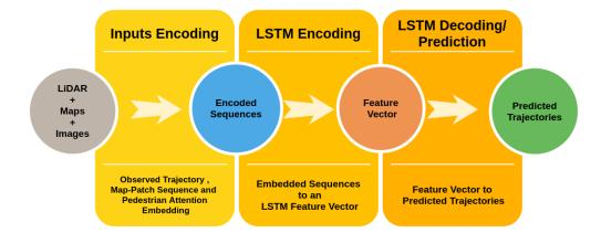
Figure 6.2: The process involved in Pedestrian Trajectory Prediction
