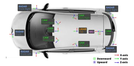
Figure 1.4: Sensor setup on a Renault Zoe used for building the NuScenes dataset (Caesar et al., 2019)
