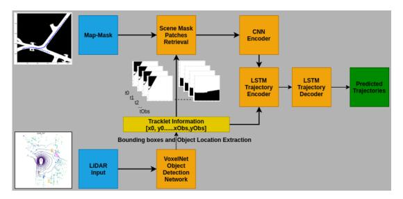
**Figure 5.3:** System Architecture: The prediction module has two inputs: sequential historical trajectories of all traffic-agents and the associated map-mask patches of each agent for the observed time instances
