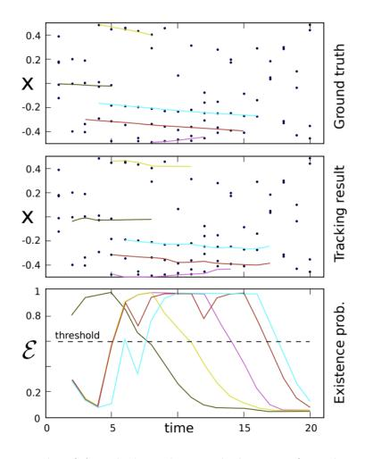
Figure 2.3: Results of A. Milan's tracking method on a 20-frame long synthetic sequence with clutter. Top: Ground truth (x-coordinate vs. time). Middle: Reconstructed trajectories. Bottom: The existence probability  $\epsilon$  for each target. Note the delayed initiation and termination, e.g. for the top-most track (yellow) in the middle. (Milan et al., 2016)
