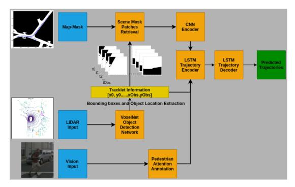
**Figure 6.6:** System Architecture: The Prediction Network has three inputs: sequential historical trajectories of all traffic-agents, the associated map-mask patches around each agent for the observed time instances and the confidence of pedestrian attention towards the autonomous agent.
