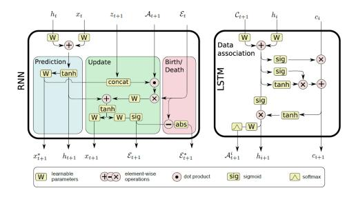
Figure 3.12: RNN-LSTM architecture used in Milan et al. (2016). Left: An RNNbased architecture for state prediction, state update, and target existence probability estimation. Right: An LSTM-based model for data association.
