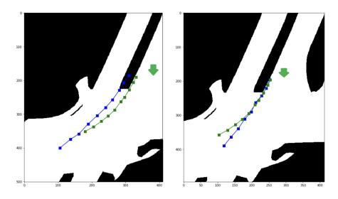
**Figure 5.9: Better behaviour in non-drivable areas:** Behaviour of Trajectory Prediction Models without (Left) and with Map-mask (Right) input. The green arrows in the images show the direction of motion of the ego-vehicle. The green trajectories are the ground truth and the blue one is the predicted trajectory
