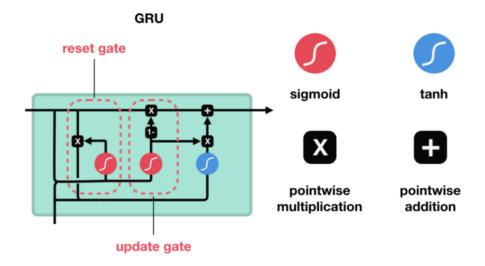
Figure 3.14: Gated Recurrent Unit Architecture (GRU, 2018)
