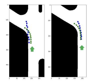
**Figure 5.8: Trajectory prediction at turnings:** Behaviour of Trajectory Prediction Models without (Left) and with Map-mask (Right) input. The green arrows in the images show the direction of motion of the ego-vehicle. The green trajectories are the ground truth and the blue one is the predicted trajectory
