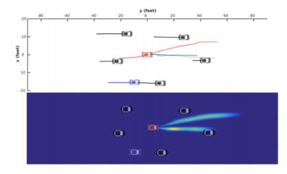
**Figure 2.4:** Illustration of Multi-modal predictions of future motion of the surrounding vehicles, along with prediction uncertainty shown here for the red vehicle. Blue is the ego-motion vehicle (Deo and Trivedi, 2018)
