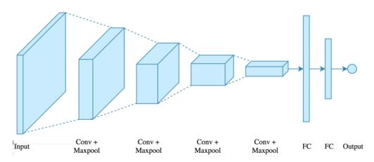
Figure 3.4: A CNN architecture with 4 convolution + pooling layers, followed by 2 fully connected layers. Input is an image and the output is a score for the class. Illustrations from Dertat (2017)
