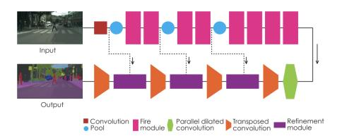
**Figure 3.6:** Architecture of network for semantic segmentation proposed in Treml et al. (2016).
