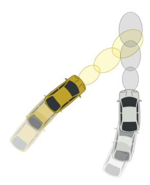
Figure 2.2: Trajectory prediction with a constant velocity motion model and Gaussian noise simulation. Ellipses represent the uncertainty on the predicted positions (Ammoun and Nashashibi, 2009). Illustrations from Lefèvre et al. (2014)
