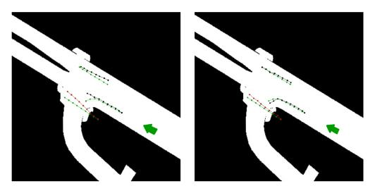
**Figure 5.10:** Multi-agent Trajectory prediction: Predictions from a model without interaction information and map-input (Left) and one with interaction information and map-input (Right). The green arrow in the image shows the direction of motion of the ego-vehicle. The green trajectories are the ground truth and the predicted trajectories are plotted in red for pedestrians and black for cars.
