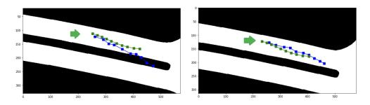
**Figure 5.7:** Straight path trajectory predictions: Behaviour of Trajectory Prediction Models without Map-mask (Left) and with Map-mask (Right) input. The green arrows in the images show the direction of motion of the ego-vehicle, ground truth (in green) and predicted trajectory (in blue).
