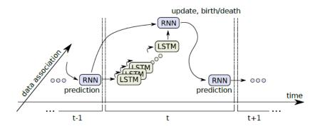
Figure 3.11: RNN Tracking architecture in Milan et al. (2016)
