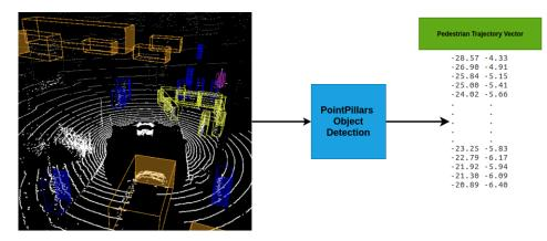
**Figure 6.3:** Observed Pedestrian Trajectory generation applying the PointPillars Algorithm (Lang et al., 2018)
