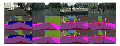
**Figure 3.7:** Example output (bottom) of the network with ground truth (centre) on images from the Cityscapes validation set. Treml et al. (2016)
