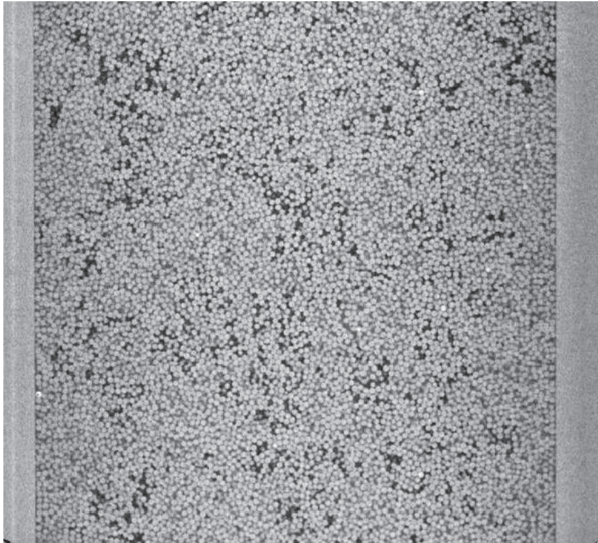
Figure 12. Packed bed millireactor section obtained via \mu -tomography [19]. The glass beads appear in white, the heptane in grey and the gas in black
