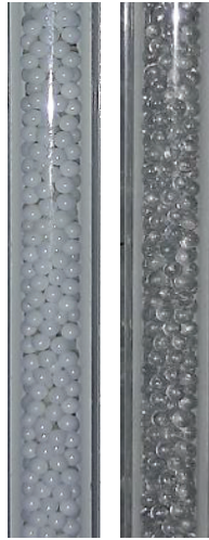
Figure 92. Packed bed millireactors used for the study of the non-porous particle material effect ( D_r=4 mm). On the left d_p=1 mm ZirBlast ® , on the right d_p=1 mm glass
