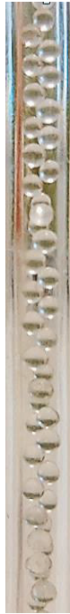
Figure 87. Photography of a reactor with internal diameter D_r=4 mm packed with glass spheres of d_p=2 mm
