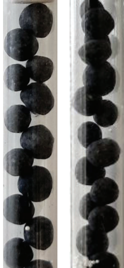
Figure 110. Examples of D_r=4 mm reactors packed with 2-2.8 mm sieved catalyst beads. On the left: mean particle size closer to 2.8 mm. On the right: mean particle size closer to 2 mm
