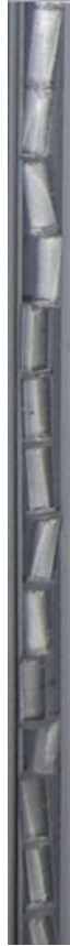
Figure 93. The single pellet string reactor tested: D_r=3 mm, d_p=2x5 mm glass cylinders and L=9 cm
