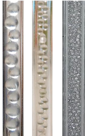
Figure 89. Packed bed millireactors used for the study of the \delta effect. D_r=4 mm, from left to right: d_p=3, 2, 1 mm
