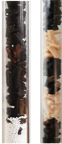
Figure 107. Left: Example of a D_r=4 mm reactor packed with catalyst quadrilobes. Right: Example of a D_r=4 mm reactor packing packed with catalyst quadrilobes in which the bed length has been elongated with inert alumina
