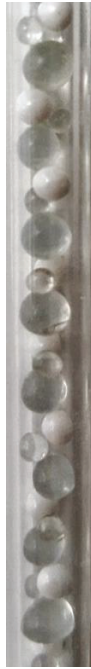
Figure 91. The polydispersed spheres packing. D_r=4 mm, d_p=2 and 3 mm glass spheres and 2.3 mm ZirBlast ® spheres
