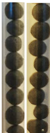
Figure 113. Examples of D_r=4 mm reactors packed with 2.8-4 mm sieved catalyst beads
