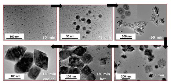
Figure 3.28: Transmission electron microscopy images of  $LiY_{5/6}Yb_{1/6}F_4$ : 0.4%  $Tm^{3+}$  samples taken at a different course of reaction from 30 min to 2 h. These images clearly show the formation of diamond morphology of nanoparticles is guided through small spherical seeds which aligns themselves in accordance to their minimum surface energy to get the most thermodynamic stable phase and morphology.
