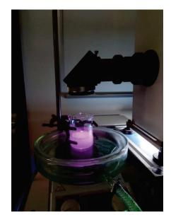
Figure 5.11: Experimental setup for degradation of methylene blue (MB).
