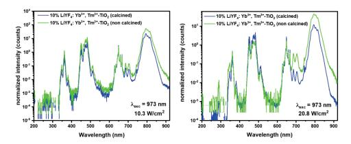
Figure 5.10: power variation upconversion emission studies for undoped  $TiO_2$  dried gel and  $LiY_{5/6}Yb_{1/6}F_4$ : 0.4%  $Tm^{3+}$  doped  $TiO_2$  samples upon 973 nm CW laser excitation. These spectra are normalized for  ${}^1G_4 \rightarrow {}^3F_4$   $Tm^{3+}$  transition.
