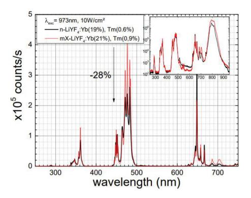
Figure 3.29: Upconversion emission spectra obtained under 10 W/cm² for the nanocrystals studied (black line) and for a single crystal (red) of the similar composition obtained by a modified Bridgman method. The doping concentrations have been measured by EDS
