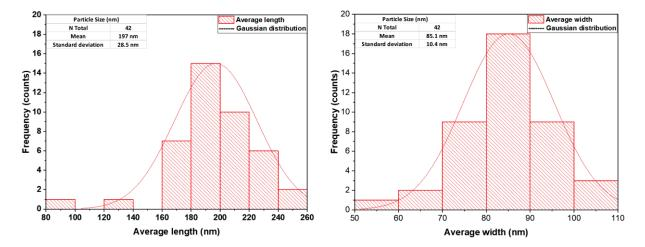
Figure 2.11: Size distribution curves along with the length (a) and width (b) of NaGd $_{5/6}$ Yb $_{1/6}$ F $_4$ : 1.2% Tm $^{3+}$  nanorods obtained from room temperature co-precipitation using hydrated inorganic salts Ln(NO $_3$ ) $_3$ ·5H $_2$ O (Ln = Gd, Tm, Yb), NaNO $_3$  and NH $_4$ F in ethylene glycol.
