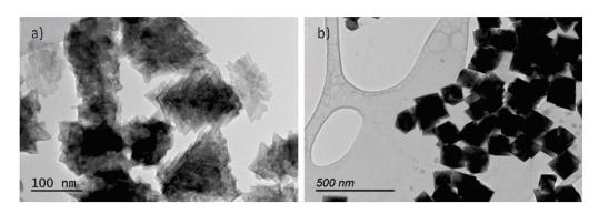
Figure 3.8: Transmission electron microscopy images of a) undoped LiYF $_4$  and b) undoped LiYbF $_4$  prepared by thermal decomposition of anhydrous molecular precursors.
