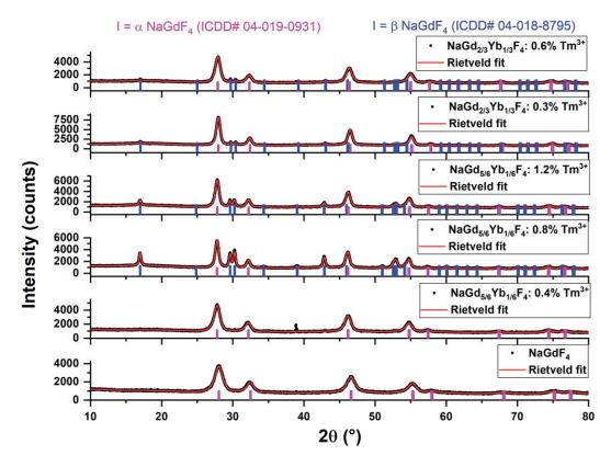
Figure 2.2: Powder XRD of NaGdF<sub>4</sub>:  $Yb^{3+}$ ,  $Tm^{3+}$  NPs obtained from the thermal decomposition of SSPs in a 1:1 mixture of ODE + OM (b).
