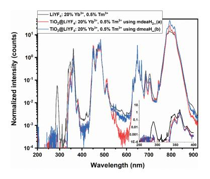
Figure 5.9: Up conversion emission studies for non-coated LiYF<sub>4</sub>:20% Yb<sup>3+</sup>,0.5% Tm<sup>3+</sup> and titania coated LiYF<sub>4</sub>:20% Yb<sup>3+</sup>,0.5% Tm<sup>3+</sup> using different ligands for functionalization, upon 972 nm CW laser excitation. These spectra are normalized with respect to  ${}^{1}G_{4} \rightarrow {}^{3}F_{4}$  Tm<sup>3+</sup> transition.
