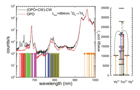
Figure 4.8: Excitation spectra of the  ${}^{1}G_{4} \rightarrow {}^{3}H_{6}$  transition with (black) or without (red) the CW IR laser at 100 mW/cm<sup>2</sup>.
