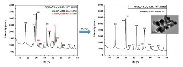
Figure 2.3: Conversion of as-prepared mixed-phase NaGd $_{5/6}$ Yb $_{1/6}$ F $_4$ : 0.8% Tm $^{3+}$  NPs (13%  $\alpha$  + 87%  $\beta$ ) to pure  $\beta$ -phase after calcination at 350 °C.
