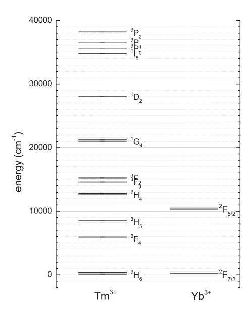
Figure 1.4: Energy level diagram for codoped Tm³+and Yb³+ system; adapted from Dulick et al. (Journal of Luminescence **1991**, 48–49, 517–521) and Bensalah et al. (Optical Materials **2004**, 26 (4), 375–383)
