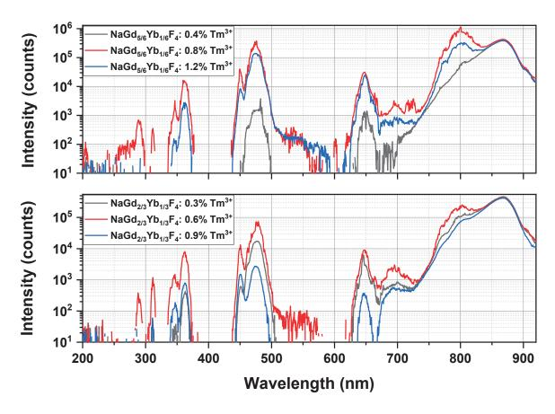
Figure 2.14: Up-conversion studies ( $\lambda_{exc}$  = 972 nm CW Laser, and slit width = 0.5 mm for entry and exit) of NaGdF<sub>4</sub>: Yb<sup>3+</sup>, Tm<sup>3+</sup> NPs obtained from the thermal decomposition method.
