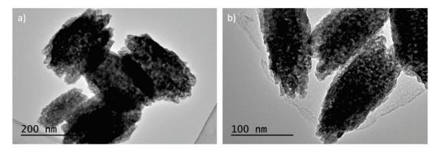
Figure 2.10: TEM images of NaGd<sub>2/3</sub>Yb<sub>1/3</sub>F<sub>4</sub>: 0.3% Tm<sup>3+</sup> (a) and NaGd<sub>5/6</sub>Yb<sub>1/6</sub>F<sub>4</sub>: 1.2% Tm<sup>3+</sup> (b) NPs obtained from room temperature co-precipitation using hydrated inorganic salts  $Ln(NO_3)_3 \cdot xH_2O$  (Ln = Gd, Tm, Yb), NaNO<sub>3</sub> and NH<sub>4</sub>F in ethylene glycol.
