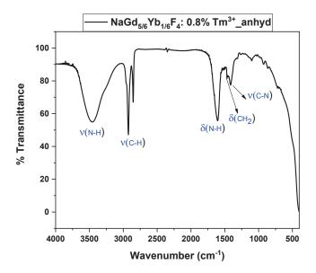
Figure 2.4: FT-IR spectra of NaGd<sub>5/6</sub>Yb<sub>1/6</sub>F<sub>4</sub>: 0.8% Tm<sup>3+</sup> NPs obtained from a) thermal decomposition of the single-source precursors [NaLn(TFA)<sub>4</sub>(diglyme)] (Ln = Gd, Yb, Tm) at 290° C in a 1:1 mixture of 1-octadecene + oleylamine.
