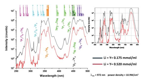
Figure 3.19: Difference in the upconversion emission intensities of the samples prepared using different concentration of precursors. These spectra were measured from dry powder in the same excitation condition for all three samples
