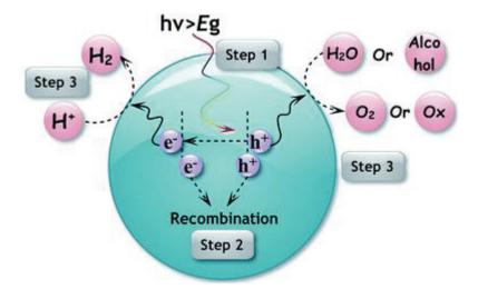
Figure 1.1: Schematic diagram of the photocatalytic reaction<sup>6</sup>.
