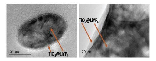
Figure 5.2: TEM images of  $TiO_2$ @  $LiY_{5/6}Yb_{1/6}F_4$ : 0.4%  $Tm^{3+}$  NPs using oleic acid as a capping ligand.
