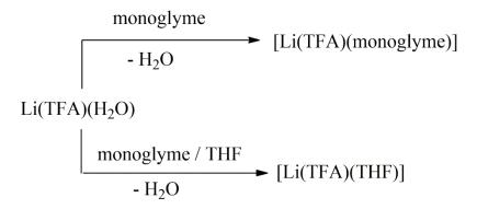
Scheme 3.1: Synthesis of anhydrous lithium precursors 1 and 2.
