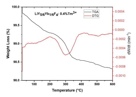
Figure 3.12: TGA and DTG curves of LiYF<sub>4</sub> doped with 20% Yb<sup>3+</sup> and 0.4% Tm<sup>3+</sup>
