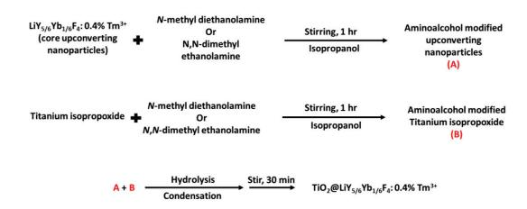
Scheme 5.1: Different steps for the synthesis of  $TiO_2@UCNPs$  shell-core structure using amino alcohols as functionalising liaand.
