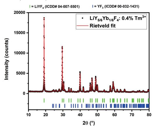
Figure 4.2: Powder XRD spectrum of LiY<sub>5/6</sub>Yb<sub>1/6</sub>F<sub>4</sub>: 0.4% Tm<sup>3+</sup> nanocrystals
