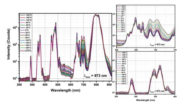
Figure 3.13: Temperature-dependent upconversion response of LiY<sub>5/6</sub>Yb<sub>1/6</sub>F<sub>4</sub>: 0.4% Tm<sup>3+</sup>.
