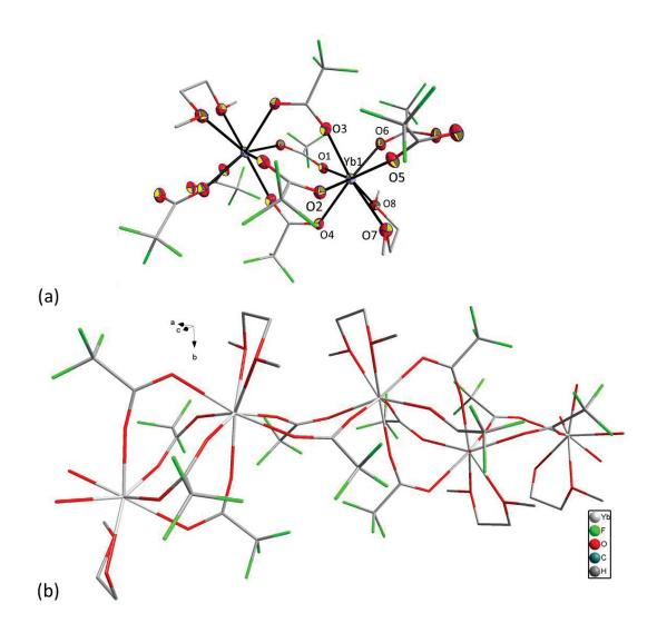
Figure 3.3: (a) Perspective view of [ $Yb(TFA)_3(monoglyme)$ ] (6) with displacement ellipsoids drawn at the 50% probability level. (b) One-dimensional structure of 6. H-atoms on monoglyme ligand have been omitted for clarity.
