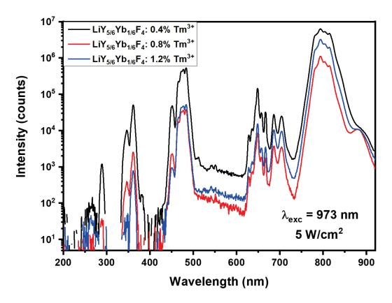
Figure 3.11: Difference in the upconversion emission intensities of the samples prepared with a different doping concentration of activator ions (Tm³+) while keeping sensitizer (Yb³+) at a fixed concentration. These spectra were measured from dry powder under similar excitation condition for all the samples.
