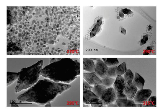
Figure 3.24: Transmission electron microscopy images of  $LiY_{5/6}Yb_{1/6}F_4$ : 0.4%  $Tm^{3+}$ samples prepared by decomposing anhydrous precursors at different temperature (from 270 °C – 315 °C).
