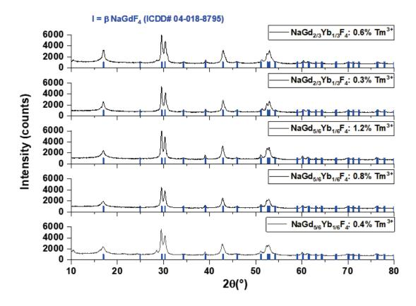
Figure 2.8: Powder XRD of NaGdF<sub>4</sub>:  $Yb^{3+}$ ,  $Tm^3+$  NPs obtained from co-precipitation reaction of hydrated inorganic salts at room temperature
