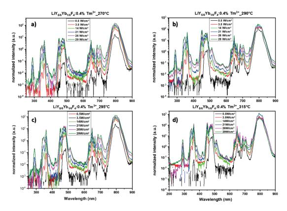
Figure 3.27: Incident power-dependent upconversion studies of LiY $_{5/6}$ Yb $_{1/6}$ F $_4$ : 0.4% Tm $^3$ +prepared by decomposing anhydrous molecular precursors at different temperatures (270 °C, 290 °C, 295 °C, and 315 °C). These samples are excited by a 973 nm CW laser.
