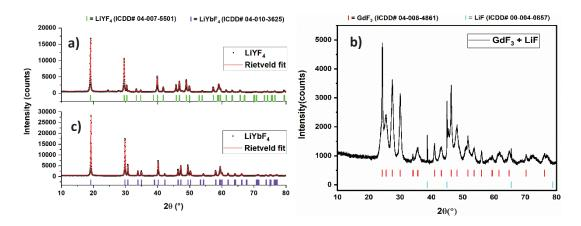
Figure 3.7: powder x-ray diffraction pattern of undoped LiLnF<sub>4</sub> (Ln = Y (a), Yb (c)) prepared by thermal decomposition of anhydrous molecular precursors in 1:1 ratio of ODE and OA. The synthesis using the Gd precursors yielded in the mixture of  $GdF_3$  and LiF (b) instead of LiGdF<sub>4</sub>. The ticks below the plot indicate the respective positions of the reflection for that particular phase.
