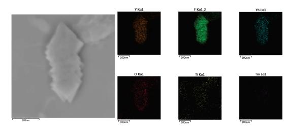
Figure 5.5: STEM imaging and EDX mapping of  $TiO_2$  coated  $LiY_{5/6}Yb_{1/6}F_4$ : 0.4%  $Tm^{3+}$  upconverting nanoparticles using N-methyl diethanolamine as a functionalizing ligand.
