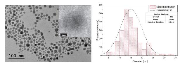
Figure 4.3: TEM and HR-TEM (inset) images of LiY $_{5/6}$ Yb $_{1/6}$ F $_4$ : 0.4% Tm $^{3+}$  nanocrystals as well as the size distribution deduced from the analysis of 235 particles.
