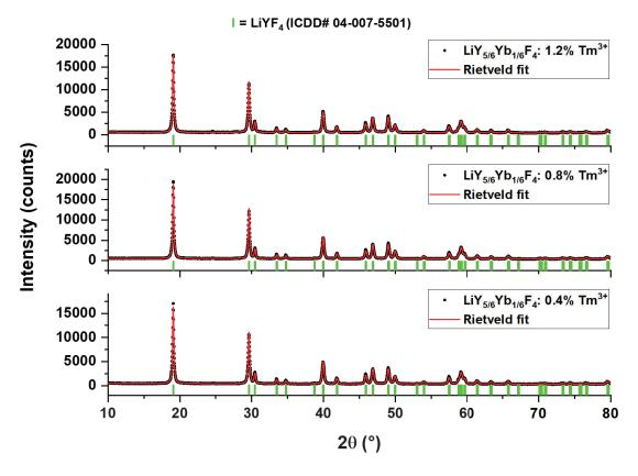
Figure 3.9: Rietveld refinement performed on X-ray diffraction pattern of a series of doped LiYF<sub>4</sub> with fixed ratio of sensitizer (Yb<sup>3+</sup>) but different ratio of activators (Tm<sup>3+</sup>) (Yb =  $^{\sim}20\%$ ; Tm = 0.4%, 0.8%, 1.2%. The ticks below the plot indicate the respective positions of the reflection for that particular phase.
