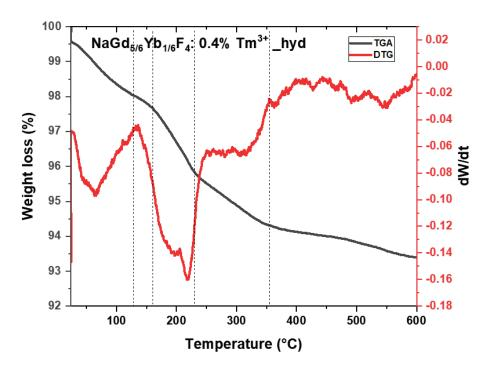
Figure 2.13: Thermogravimetric analysis (TGA) and derivative thermogravimetry (DTG) analysis of NaGd $_{5/6}$ Yb $_{1/6}$ F $_4$ : 0.4%Tm $^{3+}$  NPs obtained from the room temperature co-precipitation using hydrated inorganic salts Ln(NO $_3$ ) $_3$ ·5H $_2$ O (Ln = Gd, Tm, Yb), NaNO $_3$  and NH $_4$ F in ethylene glycol.
