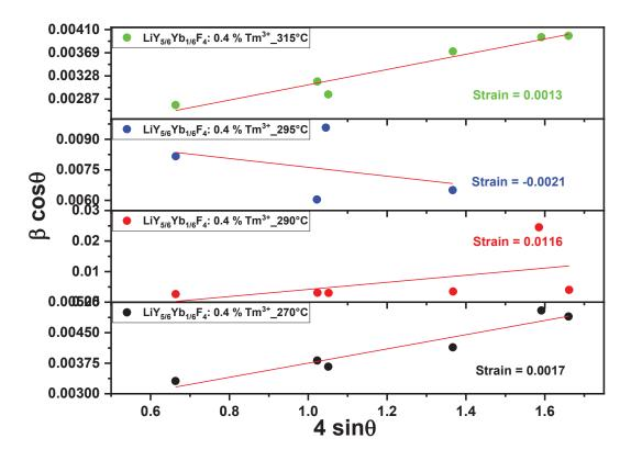
Figure 3.21: Williamson-Hall (W-H) plot derived from powder X-ray diffraction data of different samples prepared by decomposition of anhydrous precursors at varied temperatures (from 270  $^{\circ}$ C – 315  $^{\circ}$ C). The sample decomposed at 295  $^{\circ}$ C has negative strain (compression) whereas other samples have positive values of strain (tensile strain).
