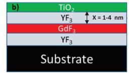
Figure 7.1: Experimental setup a) and representative figure for the different sample prepared by varying the thickness of the yttrium layer using atomic layer deposition (ALD) technique b).
