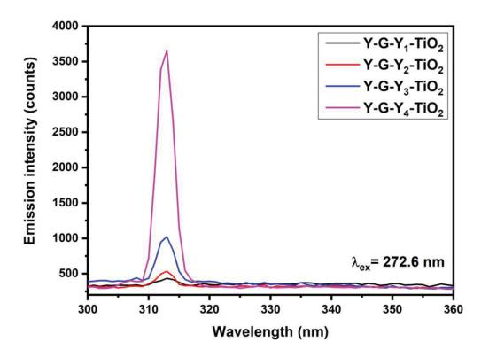
Figure 7.2: Emission spectra for different thin film samples with varying separation layer (YF<sub>3</sub>) thickness.
