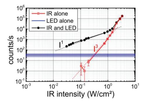
Figure 4.13: Emission intensity of the  ${}^{1}D_{2} \rightarrow {}^{3}H_{6}$  of  $Tm^{3+}$  ions in LiYF<sub>4</sub>:Yb<sup>3+</sup>,  $Tm^{3+}$  nanocrystals under dual excitation (black line) of a CW IR laser at 973 nm and an LED centred at 460 nm.
