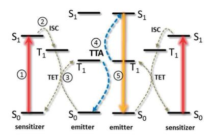
Figure 1.3: Working principle of triplet-triplet annihilation upconversion (TTA-UC).<sup>23</sup>
