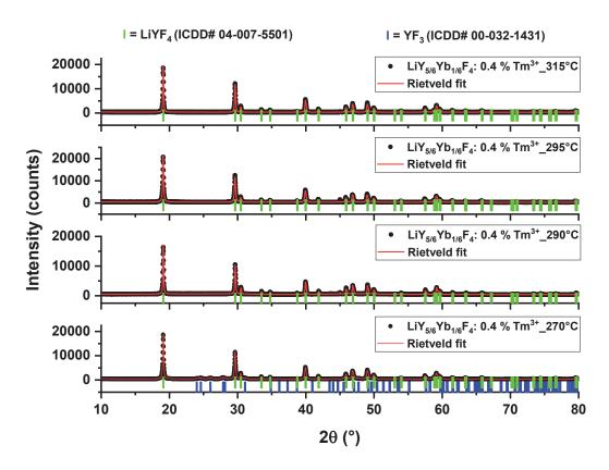
Figure 3.20: Rietveld refinement of powder X-ray diffraction pattern of different samples prepared by decomposition of anhydrous precursors at varied temperatures (from 270°C - 315°C). These peaks have been indexed with tetragonal LiYF4 and orthorhombic YF<sub>3</sub>.
