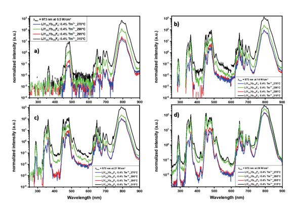
Figure 3.25: Variation of upconversion emission intensity of samples prepared at different temperatures (270 °C-315 °C).
