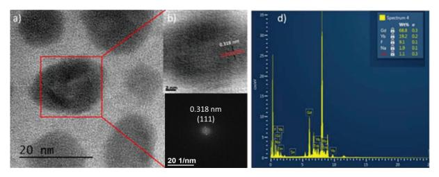
Figure 2.6: TEM (a), HRTEM (b) FFT analysis (c) and EDX analysis (d) of NaGd $_{5/6}$ Yb $_{1/6}$ F $_4$ : 0.8% Tm $^{3+}$  NPs obtained from high temperature decomposition of NaLn(TFA) $_4$ (diglyme) (Ln = Gd, Tm, Yb) in the mixture of 1-octadecene and oleylamine. The crystal structure corresponds to cubic NaGdF $_4$  (ICDD file # 04-019-0931).
