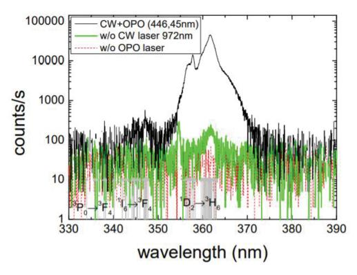
Figure 4.9: Emission spectra of  $Tm^{3+}$  ions in LiYF<sub>4</sub>:Yb<sup>3+</sup>,  $Tm^{3+}$  nanocrystals under dual excitation (black line) of a CW IR laser (~1 W/cm<sup>2</sup>) at 973 nm and an OPO laser at 446.45 nm or simple excitation with the IR laser (dashed red line) or with the OPO laser (thick green line).
