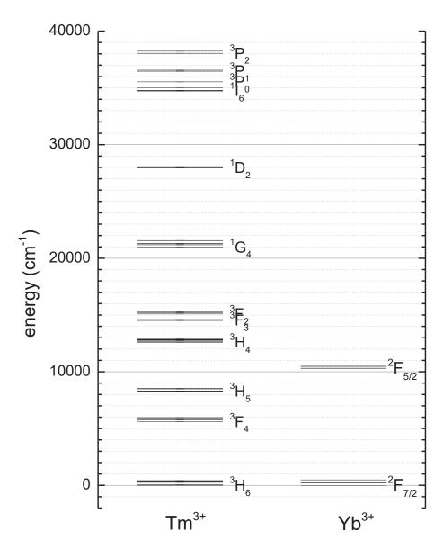
Figure 4.1: Energy level diagram for  $Tm^{3+}$  and  $Yb^{3+}$  as reported by Dulick and collaborators  $^{11}$  and also by Bensalah et al.  $^{12}$ .
