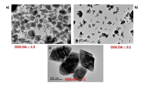
Figure 3.15: Transmission electron microscopy images of different LiY $_{5/6}$ Yb $_{1/6}$ F $_4$ : 0.4% Tm $^{3+}$  samples prepared by varying the ratio of ODE to OA as a) 1:3, b) 3:1, and c) 1:1
