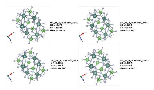
Figure 3.22: Unit cell, bond length and bond angle values for the crystal structure of different samples decomposed at different temperature (270  $^{\circ}$ C-315  $^{\circ}$ C).
