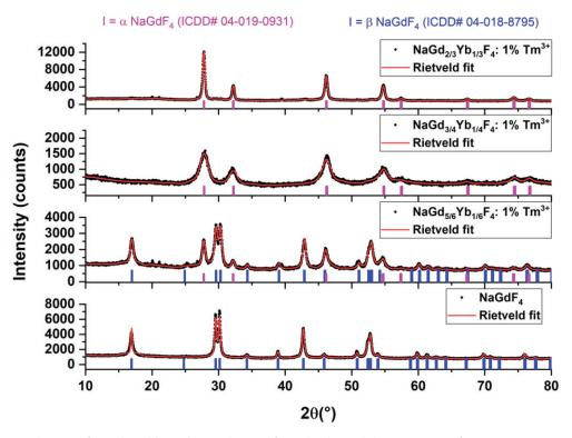
Figure 2.1: Powder XRD of NaGdF<sub>4</sub>: Yb<sup>3+</sup>, Tm<sup>3+</sup> NPs obtained from the thermal decomposition of SSPs in a 1:1 mixture of ODE + OA (a).
