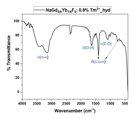
Figure 2.12: FT-IR spectrum of NaGd $_{5/6}$ Yb $_{1/6}$ F $_4$ : 0.8% Tm $^{3+}$  nanorods obtained from room temperature co-precipitation using hydrated inorganic salts Ln(NO $_3$ ) $_3$ ·5H $_2$ O (Ln = Gd, Tm, Yb), NaNO $_3$  and NH $_4$ F in ethylene glycol.
