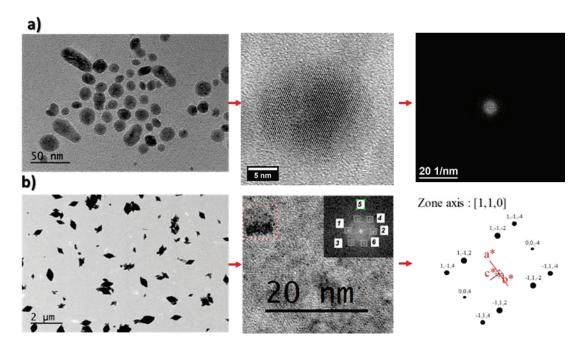
Figure 3.18: Transmission electron microscopy images of different LiY<sub>5/6</sub>Yb<sub>1/6</sub>F<sub>4</sub>: 0.4% Tm<sup>3+</sup> samples prepared by varying the concentration of precursors and their size distribution. a) 0.520 mmol/ml; b) 0.175 mmol/ml.
