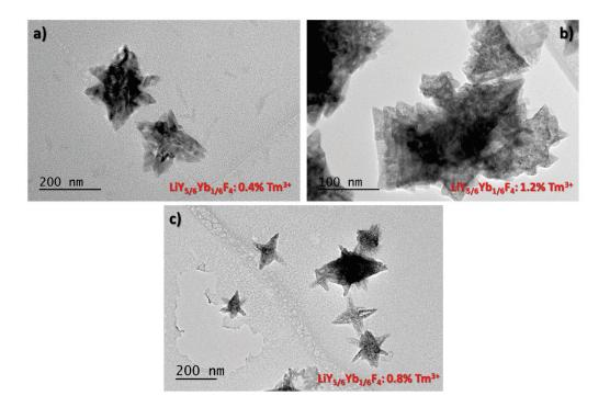
Figure 3.10: Transmission electron microscopy images of  $LiY_{5/6}Yb_{1/6}F_4$ : 0.4%  $Tm^{3+}$  (a),  $LiY_{5/6}Yb_{1/6}F_4$ : 1.2%  $Tm^{3+}$ (b) and  $LiY_{5/6}Yb_{1/6}F_4$ : 0.8%  $Tm^{3+}$ (c).
