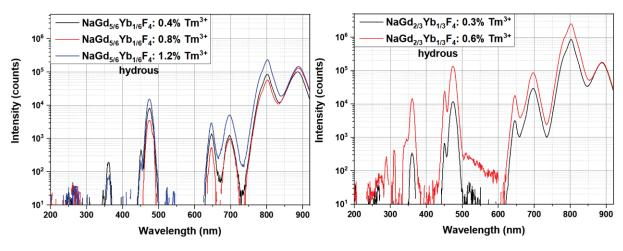
Figure 2.15: Upconversion emission spectra for NaGdF<sub>4</sub>:  $Yb^{3+}$ ,  $Tm^{3+}$ \_hyd synthesized using hydrated inorganic salts  $Ln(NO_3)_3 \cdot 5H_2O$  (Ln = Gd, Tm, Yb) with 972 nm CW laser excitation (slit width = 2 mm for both entry and exit), showing classical  $Tm^{3+}$  emission for samples with different ratio of sensitizers and activators.
