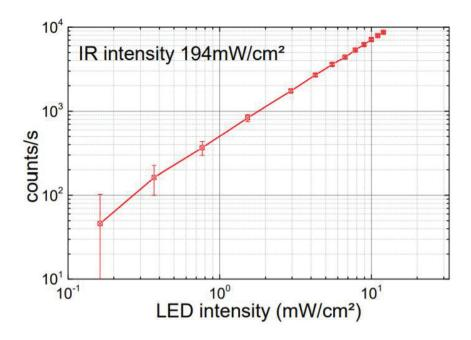
Figure 4.14: Total emission in the range 360-370 nm Tm<sup>3+</sup> ions in LiYF<sub>4</sub>:Yb, Tm nanocrystals ( $^{1}D_{2} \rightarrow ^{3}H_{6}$ ) under dual excitation of a CW IR laser at 973 nm and a LED centred at 460 nm (M455L1 from Thorlabs) with varying intensity.
