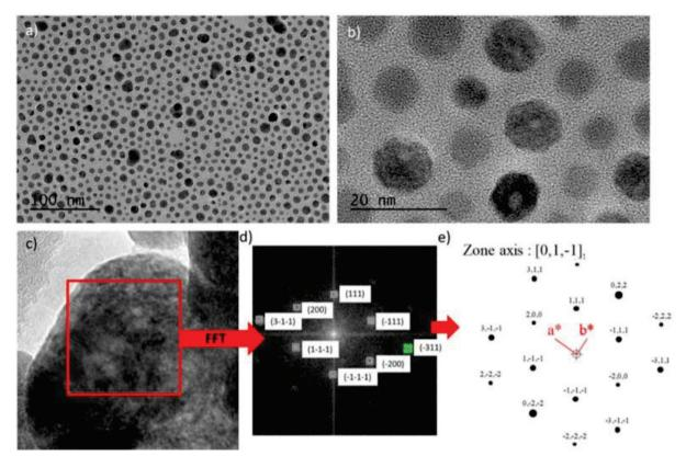
Figure 2.7: TEM (a, b), HRTEM (c) and corresponding FFT analysis (d, e) of NaGd $_{2/3}$ Yb $_{1/3}$ F $_4$ : 1% Tm $^{3+}$  NPs obtained from the high temperature decomposition of NaLn(TFA) $_4$ (diglyme) (Ln = Gd, Tm, Yb) in the mixture of 1- octadecene and oleic acid. The crystal structure corresponds to cubic NaGdF $_4$  (ICDD file # 04-019-0931).
