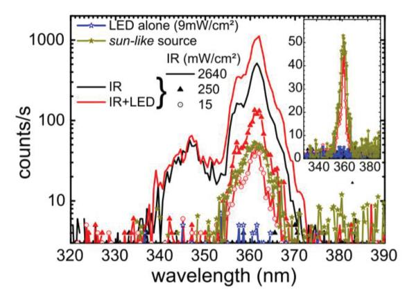
Figure 4.12: Emission spectra of Tm<sup>3+</sup> ions in LiYF<sub>4</sub>:Yb, Tm nanocrystals under dual excitation.
