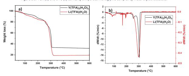
Figure 3.6: TGA (a) and DTG (b) curves of hydrated trifluoroacetate of lithium and yttrium.
