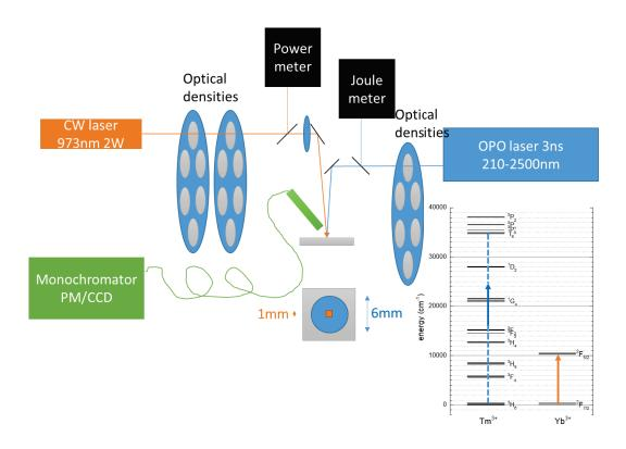
Figure 4.4: Experimental setup for excited state emission spectroscopic measurements.
