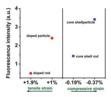
Figure 3.26: A plot of upconversion fluorescence peak intensity (green) against lattice strain of doped particle/rod and coreshell particle/rod and Yb doped LaPO $_4$  nanorod (reported by P. Ghosh et al and A. Kar et al). 40,43
