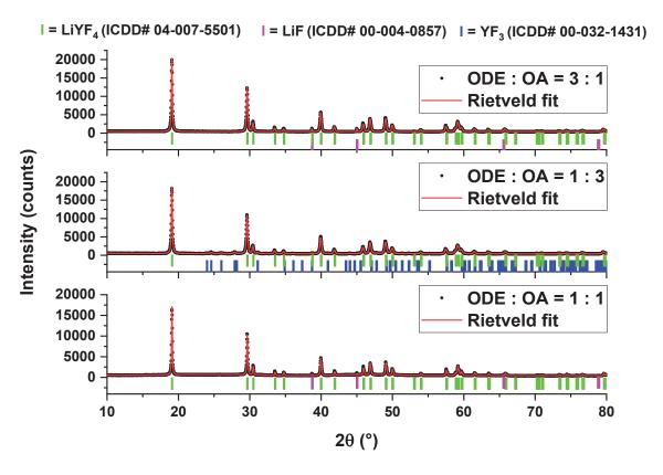
Figure 3.14: Rietveld refinement performed on X-ray diffraction pattern of three different samples prepared using different ratios of ODE and OA. The ticks below the plot indicate the respective positions of the reflection for that particular phase.
