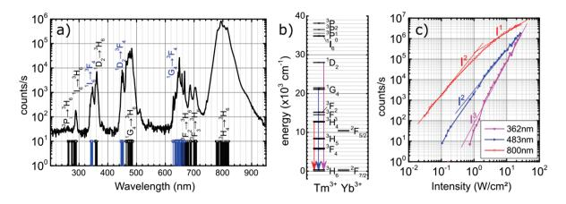
Figure 4.5: Upconversion spectra of  $LiY_{5/6}Yb_{1/6}F_4$ : 0.4%  $Tm^{3+}$  nanocrystals under a 973 nm excitation wavelength with an incidence power density of 4.32  $W/cm^2$ (a). Energy level diagram for  $Yb^{3+}-Tm^{3+}$  codoped system (b). The luminescence intensity variations of the principal emission components for the excitation intensity of the IR laser (c).
