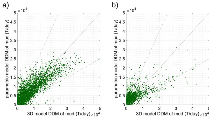
Figure III.23: Daily dredged masses of mud (a) and sand (b) at zone E computed with the parametric model vs total DDM provided by the process-based model, for the 9 simulated years.
