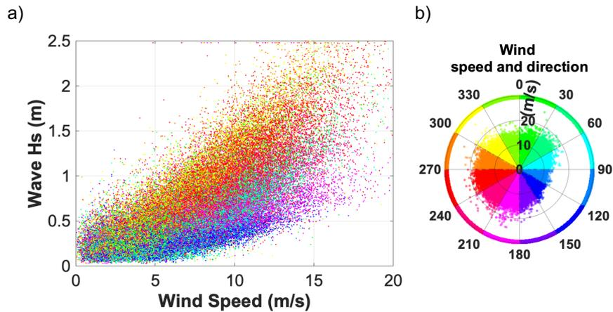
Figure III.20: a) Wind and waves correlation during the simulated period. b) Wind speed and direction during the simulated period. Waves and wind data were respectively extracted at zone V and point W specified on Figure III.14 (cf. section 3.4).
