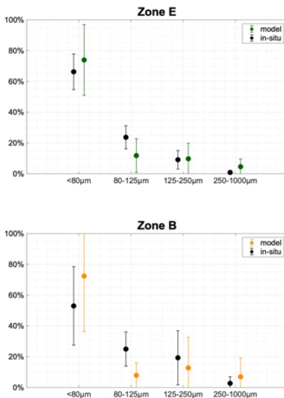
Figure III.15: Grain size comparison between in situ data and model results averaged over the 10 years period in zones E (a) and B (b).
