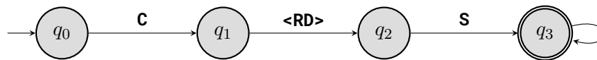
Figure 3.7: This language automaton matches \mathbf{C}\langle\mathbf{RD}\rangle\mathbf{S}.* , light paths that create caustics. It is adapted to path tracing, as vertices are sampled in the order the automaton treats them.
