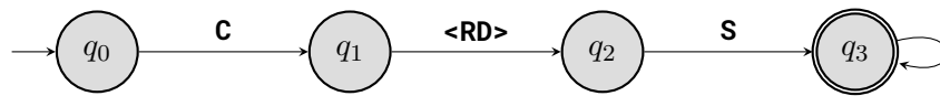
Figure 3.7: This language automaton matches \mathbf{C}\langle\mathbf{RD}\rangle\mathbf{S}\cdot* , light paths that create caustics. It is adapted to path tracing, as vertices are sampled in the order the automaton treats them.
