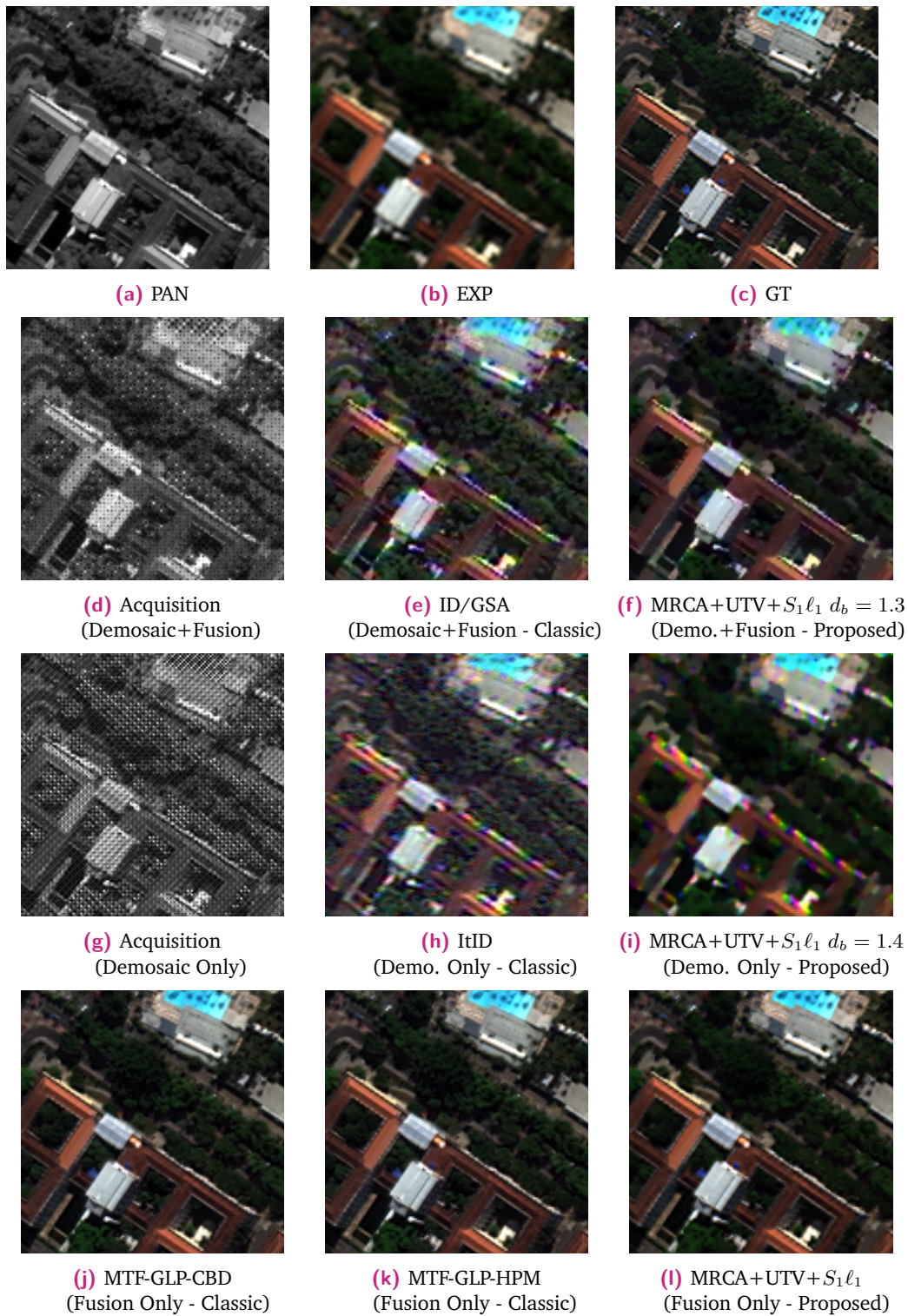
Fig. 4.12. Comparison among joint and separate fusion and demosaicing algorithms for the 8-band bundle of the Janeiro dataset ( 128 \times 128 px cropped detail). The considered acquisition setup is indicated within parentheses. The employed mask for Demosaic+Fusion is shown in Fig. 4.3d.
