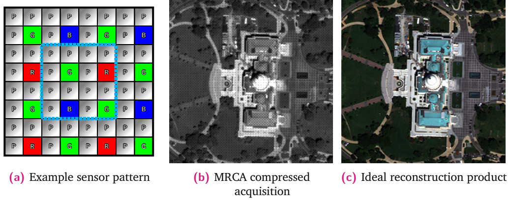
Fig. 1.5. Visual representation of the MRCA concept. In Fig. 1.5a, an example disposition of the sensors over the focal plane, with the P label referring to wideband monochromatic sensors, and R,G, and B referring to CFA with a RGB spectral response. The compressed acquisition (Fig. 1.5b) can be seen as a degraded resolution mosaiced version of the ideal acquisition to reconstruct (Fig. 1.5c).
