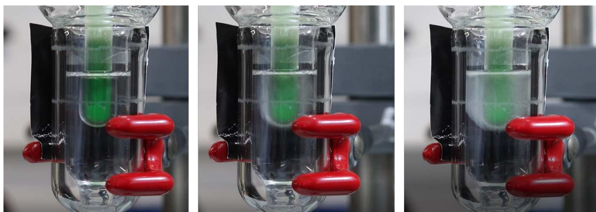
Figure 5.2: Examples of time-lapse photography, used to calculate speed and shape of freezing at 0 minutes, approximately 15 minutes and 40 minutes ( 35 \text{ g kg}^{-1} NaCl)
