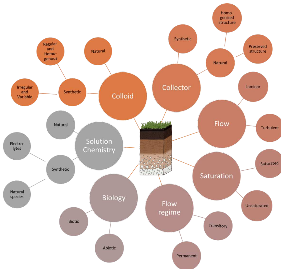
Figure 1.26: Parameters that can be complexified (inner circles) and degrees of complexity (outer circles) for experiments studying terrestrial porous media.
