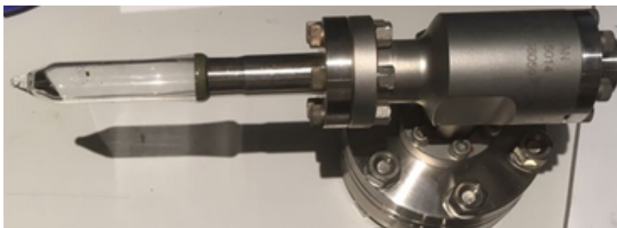
Figure 2.7: New rubidium cell before it was introduced in the setup.
