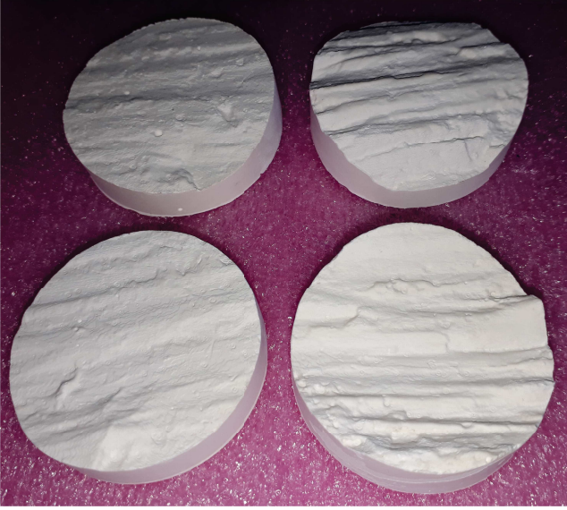
FIG. 4. Plaster faults as moulded from the 3D-printed moulds (i.e., an example of which is shown in Fig. 4). Left: S_m (top) and its complementary surface (bottom). Right: (top) and its complementary surface (bottom). The samples have a 40 mm diameter.
