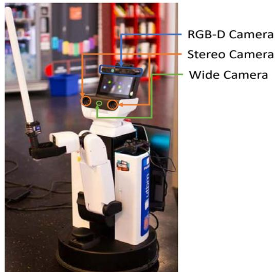
Figure 3.17: Camera system of Toyota HSR.
