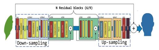
Figure 4.5: The generic architecture of ResNet-based generators
