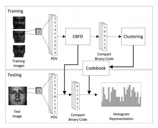
Figure 2.7: CBFD workflow for face feature extraction as proposed in [87]
