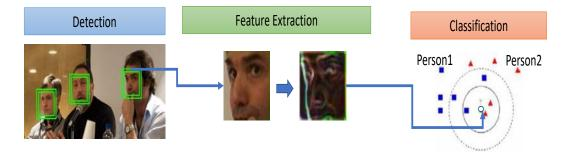
Figure 2.1: Generic architecture of an image-based facial analysis framework
