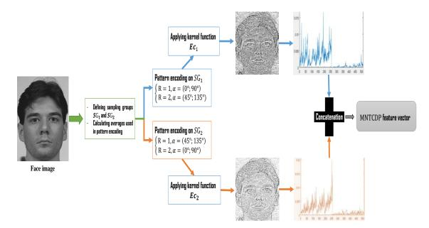
Figure 3.3: The overall framework of the MNTCDP feature vector calculation.
