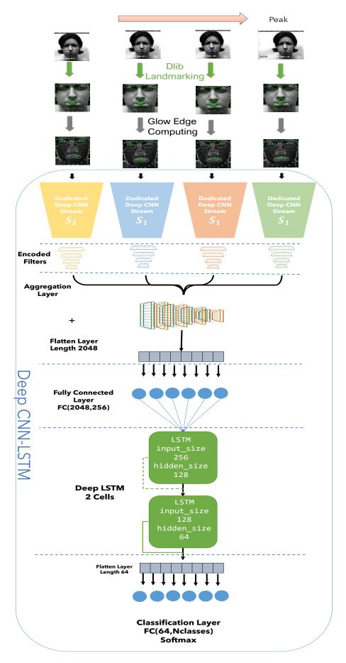
Figure 5.17: The overall pipeline of the proposed CNN-LSTM for dynamic FER model
