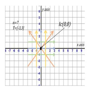
Figure 5.2: Cartesian system used to identify the pixel coordinates for each line and group.
