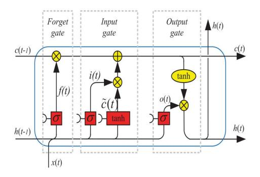
Figure 5.16: Internal configuration of the LSTM Cell
