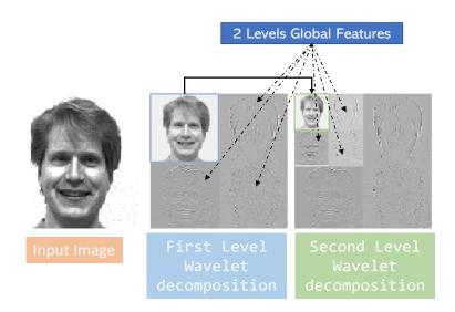
Figure 2.3: Example of extracting global features using wavelet transformations
