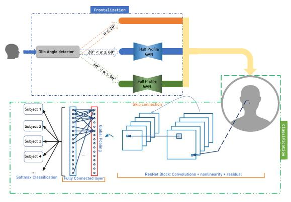
Figure 4.2: The overall architecture of the proposed PIFR framework based on GAN image translation
