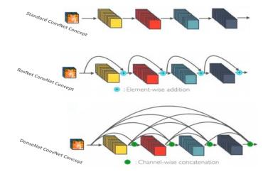
Figure 4.7: Comparison of ResNet and DenseNet residual connections
