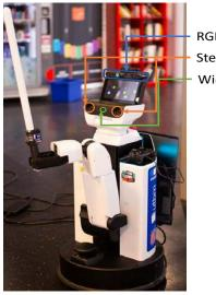
RGB-D Camera Stereo Camera Wide Camera
