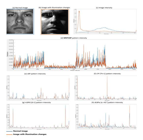
Figure 3.4: Comparing the obtained feature histograms of two images of the same person using MNTCDP, LBP, LTP, nLBPd and  $dLBP\alpha$  descriptors.
