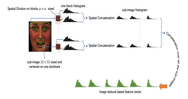
Figure 5.3: Texture feature extraction workflow based on the proposed OPD-GQMBP operator.
