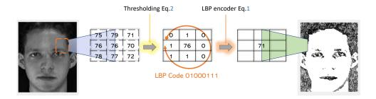
Figure 2.4: The LBP pixel transformation process.
