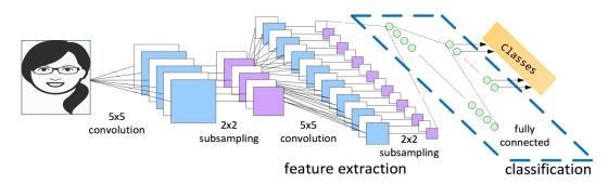
Figure 2.2: CNN-based architecture for image facial analysis
