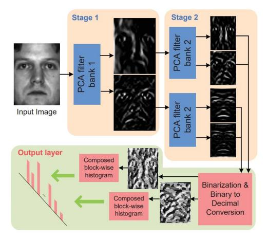
Figure 2.6: The PCANet2 learnable feature extraction method proposed in [86]
