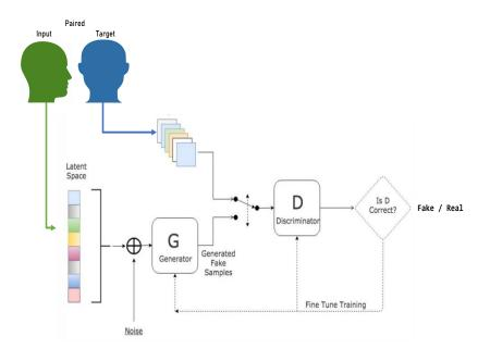
Figure 4.3: Paired GAN used for frontalization of profile image
