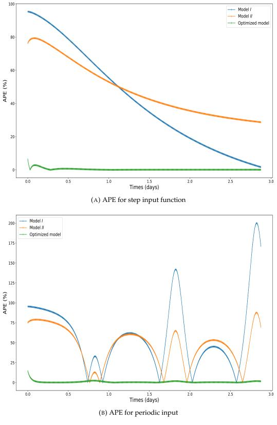
FIGURE 3.17: Evolution of APE of the medium thermal mass wall.
