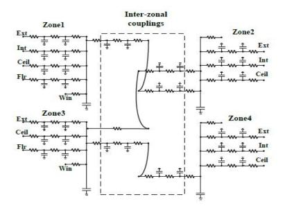
FIGURE 2.9: Resistor capacitance thermal network for multizone building [97].
