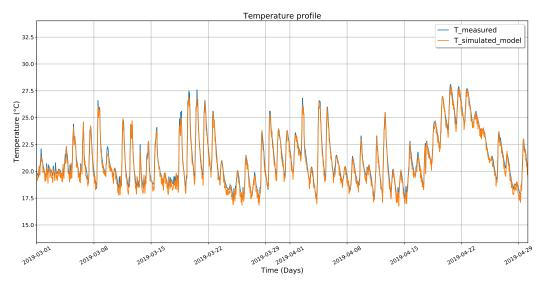
FIGURE 5.4: Validation of simplified thermal network model with measured zone temperature data (winter).
