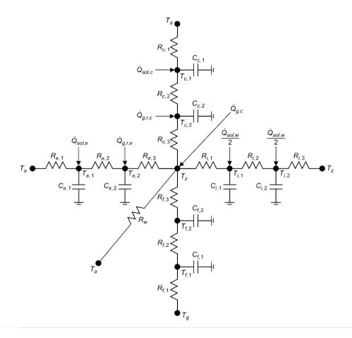
FIGURE 3.6: Thermal Network for Overall Building Model [130].
