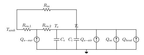
FIGURE 3.1: Thermal network model for whole building [128].
