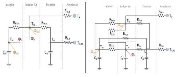
FIGURE 3.5: Building thermal structures—4R2C and 8R3C [119].
