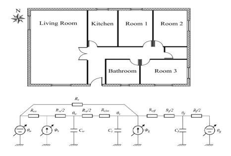
FIGURE 2.8: RC thermal network for single zone building [96].
