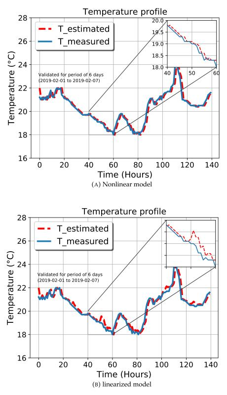
FIGURE 6.1: Validation of developed model against the measured room temperature.
