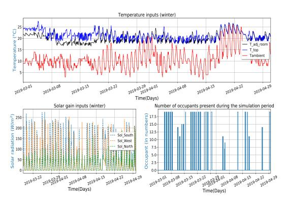
FIGURE 5.6: Measured inputs of the model: ambient and adjacent zones temperatures, solar irradiation, and occupant numbers (winter).
