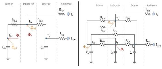
FIGURE 2.11: Building thermal structures—4R2C and 8R3C [99].
