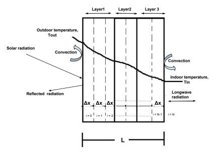
FIGURE 3.7: Heat flow through wall.
