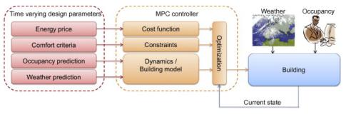
FIGURE 2.7: Basic principle of model predictive control for buildings [95].
