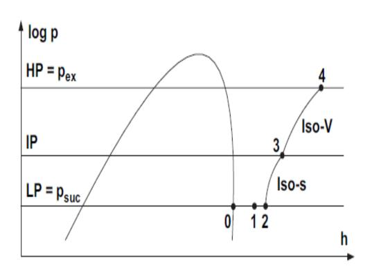
FIGURE 4.10: Thermodynamic process log(p, h) diagram [154].
