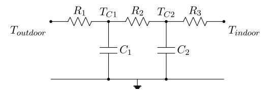
FIGURE 3.3: Simplified thermal network model - 3R2C.
