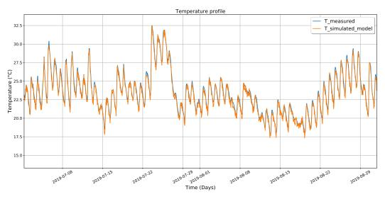
FIGURE 5.5: Validation of simplified thermal network model with measured zone temperature data (summer).
