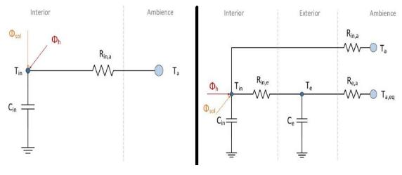
FIGURE 2.10: Building thermal structures—1R1C and 3R2C [99].
