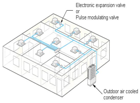
FIGURE 2.18: ASHP-VRF system with multiple indoor units [110].
