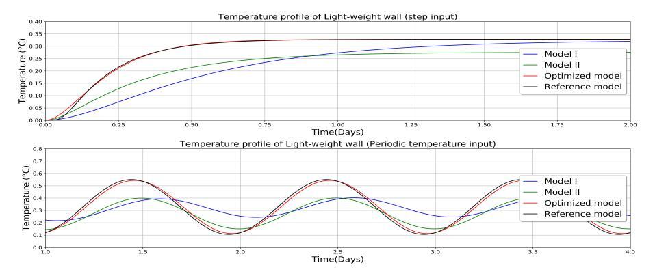
FIGURE 3.14: Temperature dynamics of reference, optimized and comparison models for light weight wall.
