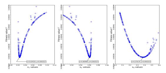
FIGURE 3.13: Optimized values of  $R_1$ ,  $R_2$ , and  $C_1$  coefficients ( $x_1, x_2$ , and  $x_4$ ) with PSO algorithm.
