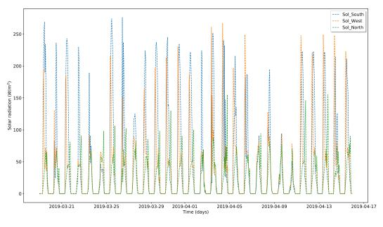
FIGURE 4.5: Measured solar radiation incident on wall surfaces.
