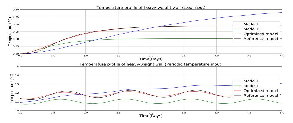
FIGURE 3.18: Temperature dynamics of reference, optimized and comparison models for heavy weight wall.
