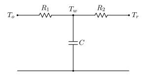
FIGURE 3.9: First order lumped parameter model - 2R1C
