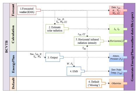
FIGURE 2.5: Process of generating a weather data file based on the forecasted weather [70].
