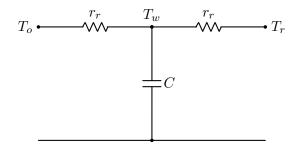
FIGURE 3.2: Simplified thermal network model - 2R1C [129].
