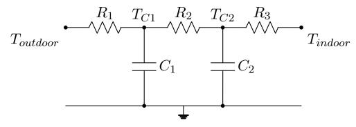
FIGURE 3.10: Simplified thermal network model - 3R2C.
