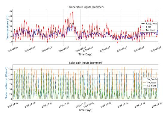
FIGURE 5.7: Measured inputs of the model: ambient and adjacent zones temperatures, and solar irradiation (summer).
