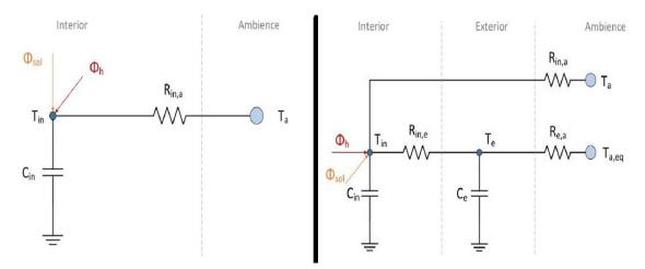
FIGURE 3.4: Building thermal structures—1R1C and 3R2C [119].
