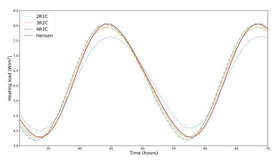
FIGURE 3.11: Comparison of simulated heat load from RC models and reference model.
