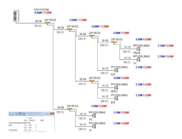
FIGURE 4.11: VRF system installed in the case study building.
