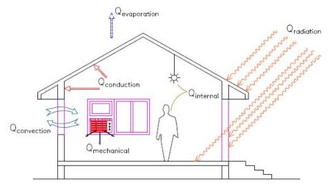
FIGURE 2.1: Heat and mass transfer processes involved in buildings [34]
