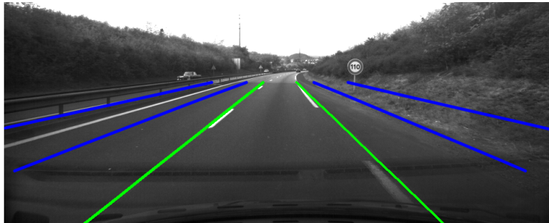
Figure 8.2: Confidence intervals for adjacent hypothesized edges for a two lanes road. Green represents the estimated edges of the ego-lane and blue illustrates the confidence intervals for the possible positions of the adjacent lanes marking.
