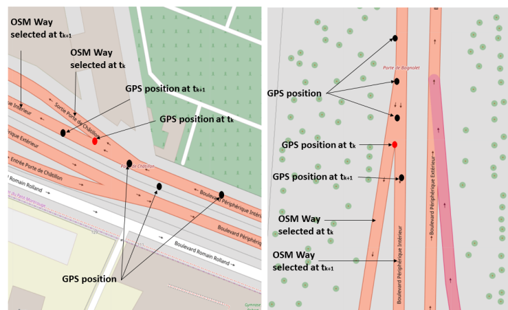
Figure 6.17: Scenarios where the map matching algorithm selects the wrong segment and leads to a false lanes number estimation
