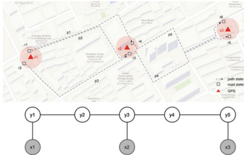
Figure 2.8: A CRF for 3 GPS observations. The map on top illustrates the simplified situation of identifying road states and path states given GPS observations in the road network. This requires 5 random variables, y_1 : \{r_1, r_2\} , y_2 : \{p_1, p_2, p_3\} , y_3 : \{r_3, r_4\} , y_4 : \{p_4, p_5\} , y_5 : \{r_5, r_6\} , to build the CRF for map matching. Thus, nodes y_1, y_3, y_5 linking with observations (black circles) are point nodes while nodes y_2, y_4 are path nodes [98]
