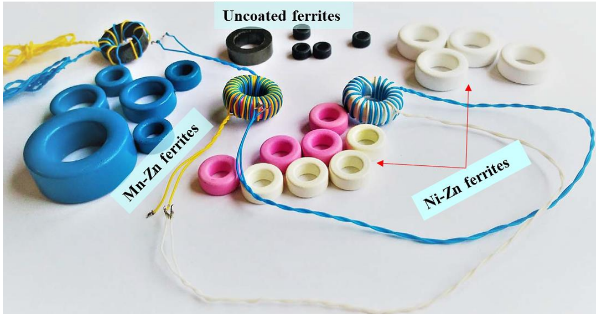
Figure 1.8 Some commercial toroidal ferrite magnetic cores (adapted from [9])
