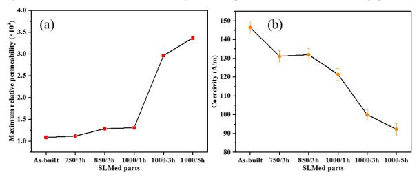
Figure 4.24 (a) The evolution of maximum relative permeability, and (b) the evolution of coercivity for SLMed Fe-3wt.%Si specimens before and after different annealed treatments
