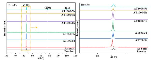
Figure 4.22 XRD analysis of SLMed Fe-3wt.%Si magnets
