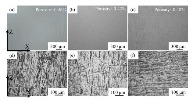
Figure 5.1 The representative OM images of the microstructures of XZ planes without etching for the SLMed silicon steels (a) Fe-3.5wt.%Si, (b) Fe-4.5wt.%Si, (c) Fe-5.5wt.%Si, and after etching (d) Fe-3.5wt.%Si, (e) Fe-4.5wt.%Si, (f) Fe-5.5wt.%Si
