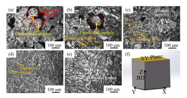
Figure 3.12 OM images (XY plane) of the SLMed parts at different LED and 3D physical model of the samples: (a) 150 J/m, (b) 210 J/m, (c) 300 J/m, (d) 420 J/m, (e) 540 J/m, (f) 3D physical model of the samples
