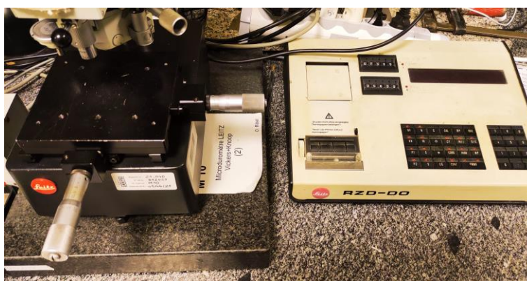
Figure 2.15 The microhardness tester
