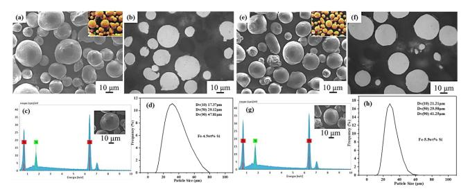
Figure 2.4 Characterization of Fe-4.5wt.%Si: (a-d) and Fe-5.5wt.%Si (e-h): (a) (e) morphology and EDS mapping (b) (f) cross-section of the particles, (c) (g) the results of EDS, (d) (h) particle size distributions
