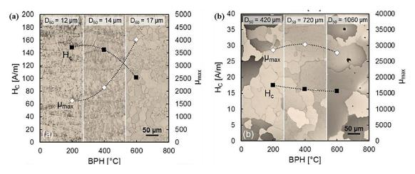
Figure 1.40 Influence of BPH temperature on the microstructure (average grain size D50) and magnetic properties of  $H_c$  and  $\mu_{max}$ : for Fe-6.7wt.%Si parts (a) as-built state, (b) after annealing at 1150 °C for 1 h [108]
