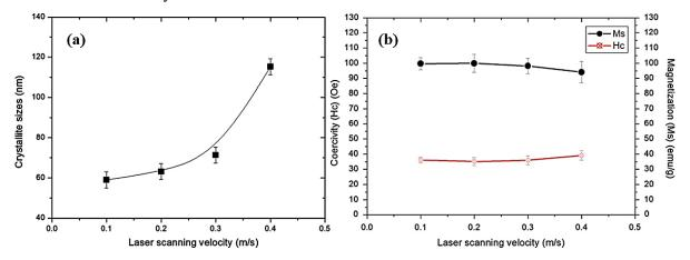
Figure 1.29 (a) Crystallite size of Fe-80wt.%Ni versus laser scanning velocity, (b) Saturation magnetization and coercivity curves for Fe-80wt.%Ni alloy with laser scanning velocity [203]
