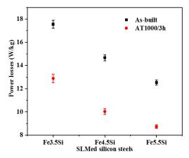
Figure 5.16 The evolution of the power losses P<sub>50-1</sub> in dynamic conditions
