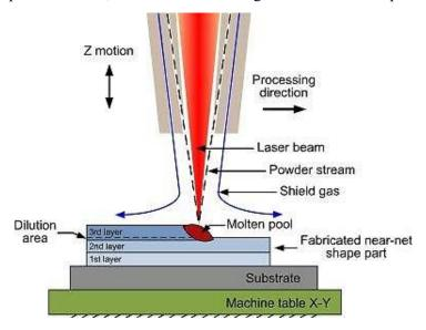
Figure 1.21 Diagram of LENS [159]
