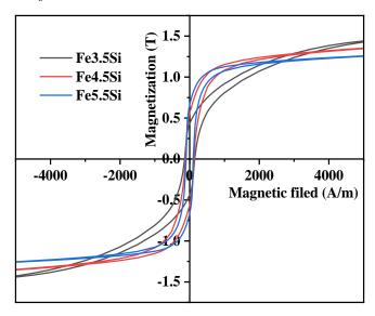
Figure 5.3 The DC hysteresis loops of three SLMed silicon steels under different Si content
