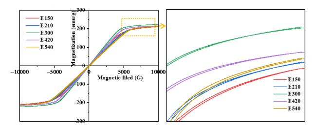
Figure 3.19 Hysteresis loops of the initial powder and SLMed samples, the right set shows the enlargement part in the low magnetic field region
