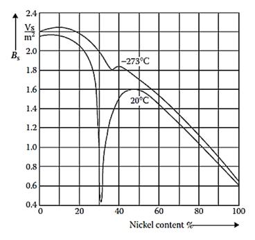
Figure 1.7 Saturation magnetic induction in iron-nickel alloys [39]
