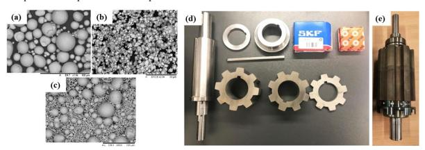
Figure 1.30 SEM micrographs of metallic powders: (a) pre-alloyed Fe-6.9wt.%Si, (b) pure iron Fe (99.9%), (c) Fe-wt.%. Si powder blend [204] and (d) Main components for the assembly of the SLMed soft magnetic rotor core, (e) Fully assembled 3D printed SRM rotor (Fe-5.0wt.%Si) [197]
