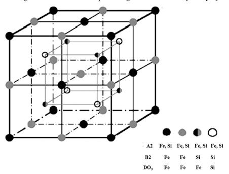
Figure 1.12 Superlattice crystal lattice of high silicon steel. For the disordered A<sub>2</sub> phase, Fe and Si can sit in any of the plotted sites. For B<sub>2</sub>, Fe prefers the sites denoted by solid black dots and gray dots, while Si prefers the sites denoted by gradient dots and open dots. For DO<sub>3</sub>, Si prefers the sites denoted by open dots, while Fe prefers all the other sites [68]
