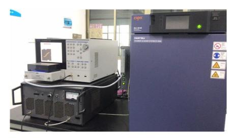
Figure 2.14 AC magnetic property measurements system
