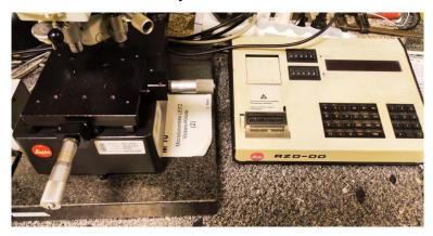
Figure 2.15 The microhardness tester
