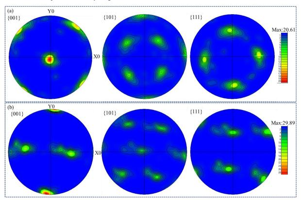
Figure 4.7 The pole figures (PF) of two different planes (a) XY plane, (b) XZ plane
