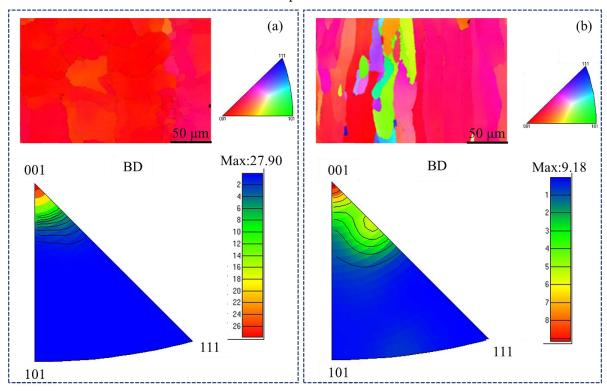
Figure 4.21 EBSD maps and IPFs after heat treatment (a) XY plane, (b) XZ plane
