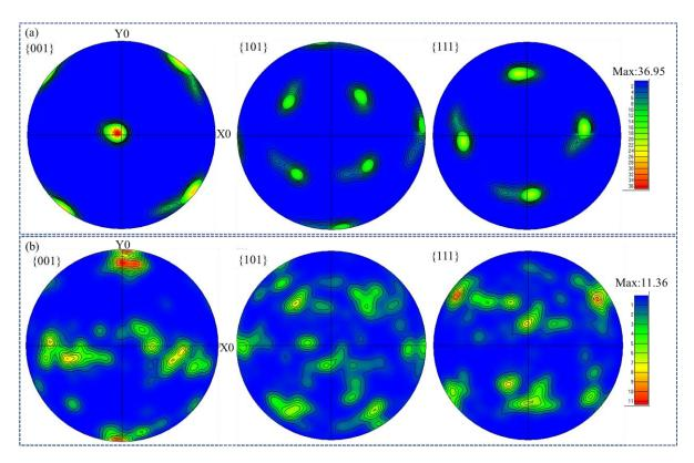
Figure 4.20 The pole figures (PF) after heat treatment of two different planes (a) XY plane, (b) XZ plane
