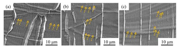
Figure 5.2 The representative SEM images of the microstructures of XZ planes after etching for the SLMed silicon steels (a) Fe-3.5wt.%Si, (b) Fe-4.5wt.%Si, (c) Fe-5.5wt.%Si
