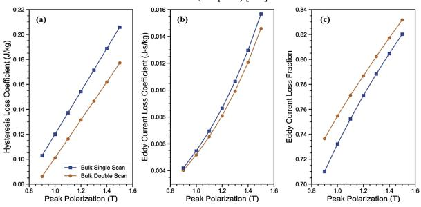
Figure 1.37 Results of magnetic characterization of the two bulk (Fe-3Si) cross-sections with different scan patterns: (a) the hysteresis loss coefficients as a function of peak polarization, (b) the eddy current loss coefficient as a function of peak polarization, (c) the fraction of total losses accounted for by the eddy current development as a function of peak polarization for an operating frequency of 60 Hz [129]
