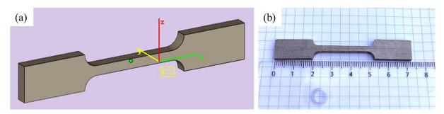
Figure 4.1 (a) 3D model, (b) an SLM fabricated sample for tensile test
