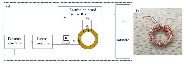
Figure 2.13 (a) A schematic of the AC magnetic measurements setup, (b) a measured sample
