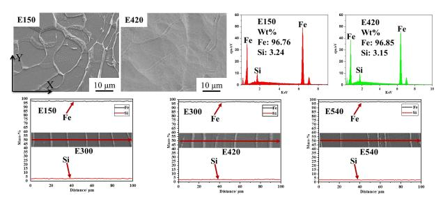
Figure 3.16 The results of EDS for the SLMed samples
