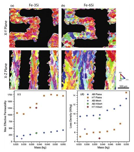
Figure 1.42 Inverse pole figure maps for the Hilbert transformer cores after annealing (a) Fe-3wt.%Si, (b) Fe-6wt.%Si [216] and Magnetic test results (c) maximum effective permeability for the HIP heat-treated samples, (d) total loss density at an applied field of 3000 A/m (adapted from [129])
