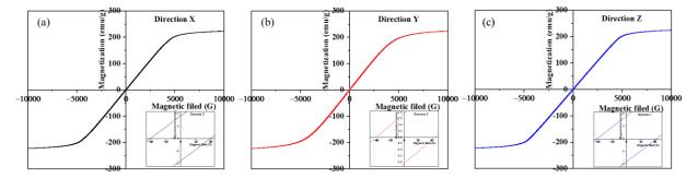
Figure 4.6 The magnetization curves in different measured directions and their enlarged-view graphs of low magnetic field
