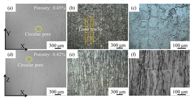
Figure 4.2 OM images of the SLMed samples (a-c) XY plane, (d-f) XZ plane
