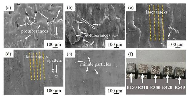
Figure 3.8 Macroscopic morphology and SEM images of surface morphology of SLMed samples at different LED: (a) Macroscopic morphology of the SLMed samples, (b) 150 J/m, (c) 210 J/m, (d) 300 J/m, (e) 420 J/m, (f) 540 J/m
