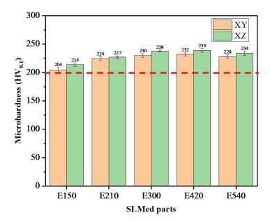
Figure 3.17 Microhardness of the SLM parts prepared at the different LED
