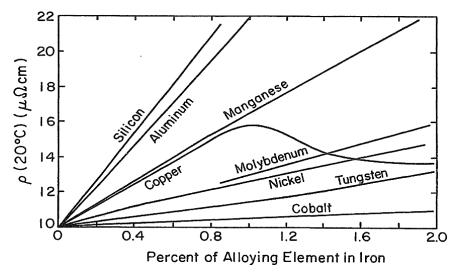
Figure 1.10 Variation in electrical resistivity of iron with the addition of selected impurities [58, 60]
