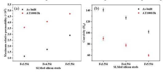
Figure 5.14 The evolution of the (a)  $\mu_{max}$ , (b) H<sub>c</sub> of the different SLMed silicon steel samples before and after annealing
