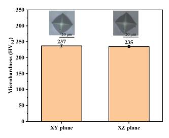
Figure 4.11 Vickers microhardness of SLMed sample
