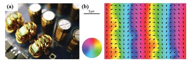
Figure 1.9 Two views of soft magnetic materials: (a) A row of three wound toroidal inductors mounted on a printed circuit board, (b) Magnetooptical Kerr effect image of the magnetization pattern on the surface of an amorphous alloy soft magnet, credits: (left to right) Billonll/Istock [9]
