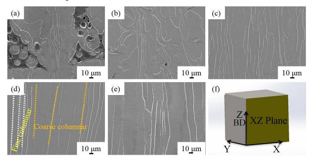
Figure 3.14 SEM images of the microstructures (XZ plane) of the SLMed specimens and 3D physical model of the samples (a-e): (a) E150, (b) E210, (c) E300, (d) E420, (e) E540; (f) The 3D physical model of the samples
