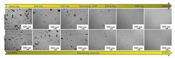
Figure 3.3 Effect of processing LED on sample porosity: the OM images of different SLMed Fe-3wt.%Si samples fabricated under the parameters of group 2
