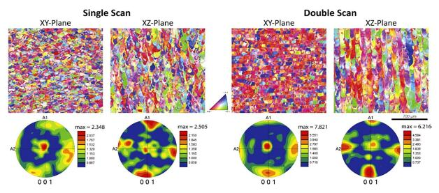
Figure 1.36 EBSD of the bulk cross-sections showing inverse pole figures of SLMed Fe-3Si specimens (top) and pole figures (bottom) for both scan patterns both normal (XY-plane) and parallel to the BD (XZ-plane) [129]
