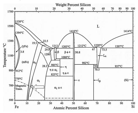
Figure 1.11 Kubaschewski phase diagram for the Fe-Si system [72]
