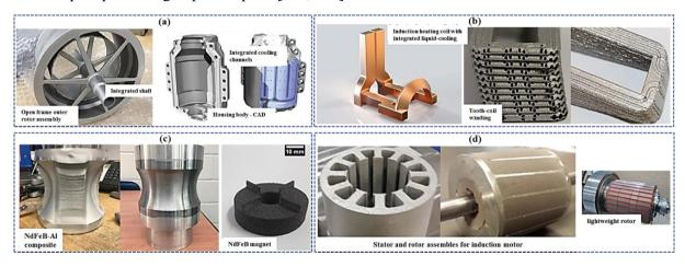
Figure 1.20 Examples of AM parts for electrical machine (a) mechanical and thermal management assemblies [112, 113]; (b) coils/windings: [117, 118]; (c) permanent magnets (PM) [119, 120], (d) stator/rotor packs: [122, 124]
