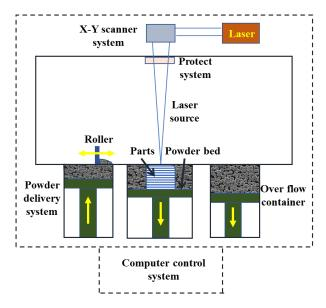
Figure 1.23 Diagram of schematic SLS/M system [161]
