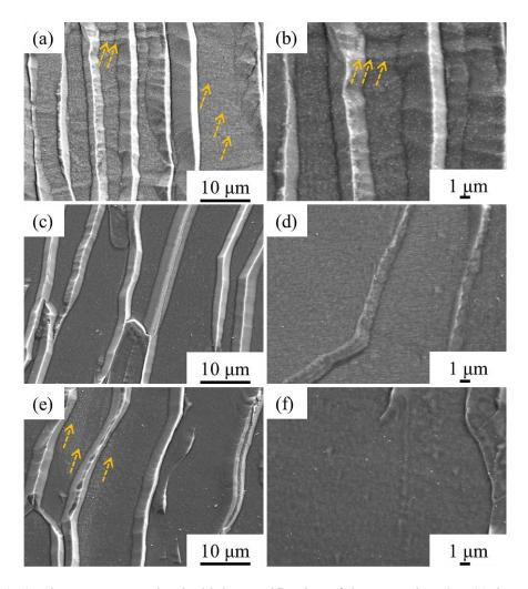
Figure 4.18 Microstructure under the high magnification of the SLMed Fe-3wt.%Si specimens observed via SEM after etching: (a-b) SLMed as-built specimen, (c-d) SLMed AT750/3hspecimen, (e-f) SLMed AT850/3h specimen
