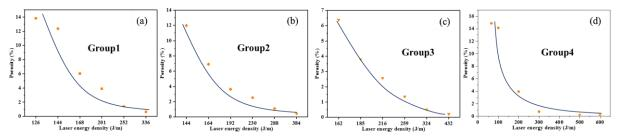
Figure 3.6 The evolution of porosity of different SLMed Fe-3wt.%Si samples (a) group1, (b) group2, (c) group3, (d) group4
