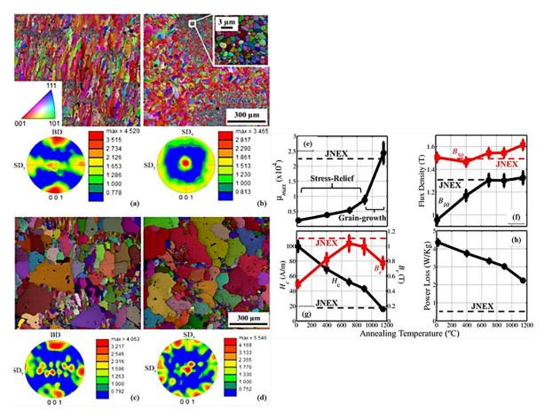
Figure 1.39 EBSD maps and PFs for SLMed Fe-6.9wt.%Si samples annealed 1h at 700 °C (a) front view, (b) top view and 1150 °C (c) front view, (d) top view; and Evolution of the magnetic properties with annealing temperature: (e)  $\mu_{max}$ , (f)  $B_{10}$  and  $B_{50}$ , (g)  $H_c$  and  $B_r$ , (h) power losses at  $B_{max}$ =1 T and f=50 Hz (adapted from [211, 212])
