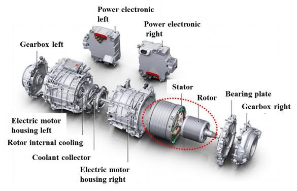
Figure 1.17 Twin motor of Audi e-tron S sportback seriers [93]
