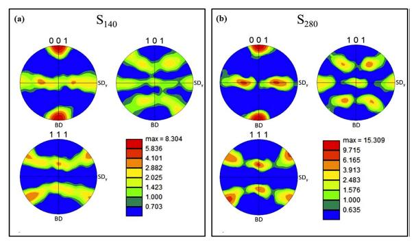
Figure 1.32 Pole figures (PF) showing the preferred orientation of the <001> crystallographic direction of SLMed Fe-6.9%wt.Si sample[209]
