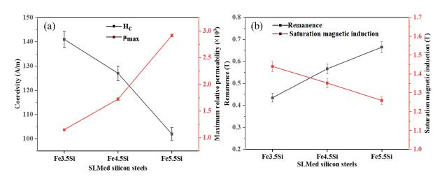
Figure 5.4 The evolution of DC magnetic properties for three SLMed silicon steels under different Si content
