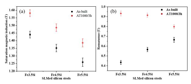
Figure 5.15 The evolution of the (a) B<sub>s</sub>, (b) B<sub>r</sub> of the different SLMed silicon steel samples before and after annealing
