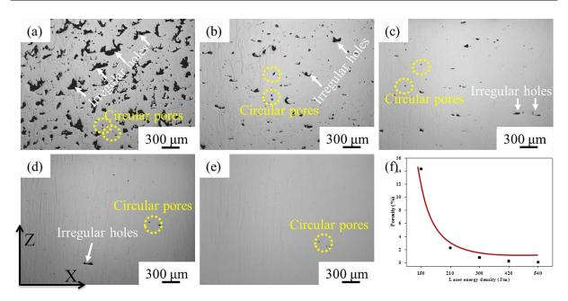
Figure 3.10 OM images of cross-sectional (XZ plane) at different LED and porosity rate of SLMed specimens at different LED: (a) 150 J/m, (b) 210 J/m, (c) 300 J/m, (d) 420 J/m, (e) 540 J/m, (f) porosity rate changes as a function of laser energy density
