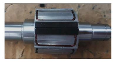
Figure 1.49 SLM rotor active part and shaft of a PM motor (Fe-Co alloy) [25]
