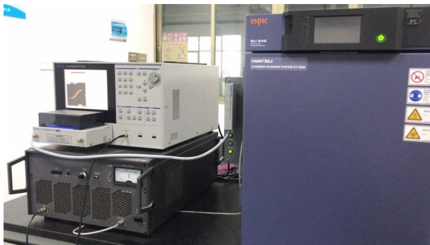
Figure 2.14 AC magnetic property measurements system
