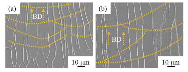
Figure 3.15 SEM images of the high magnification for representative microstructures (XZ plane) at different LEDs: (a) 300 J/m, (b) 540 J/m
