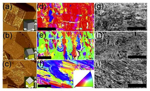
Figure 1.48 The photograph, EBSD map and SEM images of permalloy-80 built at different geometries: (a) (d) and (g) <100> geometry (b), (e) and (h) are <110> geometry, (c), (f) and (I) are designed according to <111> geometry. All the scalebars represent 200 μm [218]
