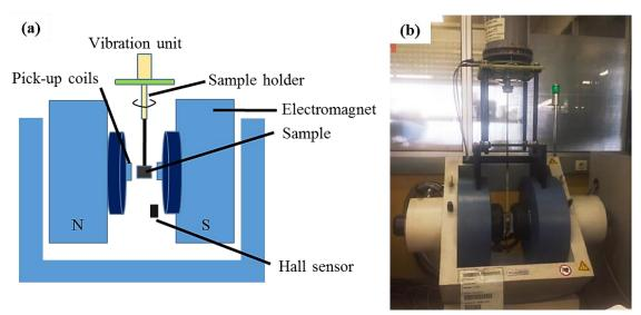
Figure 2.12 A schematic diagram and equipment of the VSM
