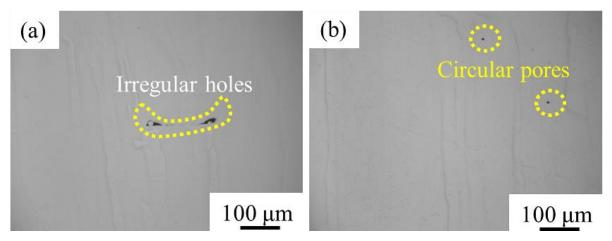
Figure 3.11 Magnification OM images of XZ plane for SLMed specimens at different LED: (a) 210 J/m, (b) 540 J/m
