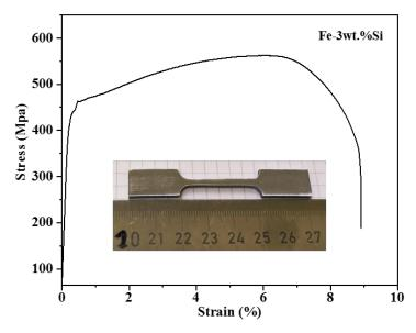
Figure 4.12 Tensile stress-strain curves for SLMed Fe-3wt.%Si part
