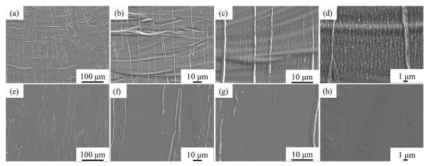
Figure 5.11 Microstructure of the SLMed Fe-5.5wt.%Si samples observed via SEM after etching: (a-d) as-built samples, (e-h) AT1000/3h samples
