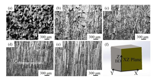
Figure 3.13 OM images of the microstructures (XZ plane) the SLMed specimens and 3D physical model of the samples: (a) 150 J/m, (b) 210 J/m, (c) 300 J/m, (d) 420 J/m, (e) 540 J/m, (f) 3D physical model of the samples
