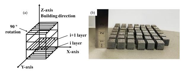
Figure 3.1 (a) Scanning strategy, (b) SLMed specimens
