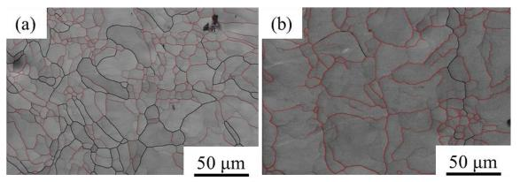
Figure 4.16 Microstructure of XY plane for SLMed Fe-3wt.%Si sample (a) as-built, (b) AT1000/3h
