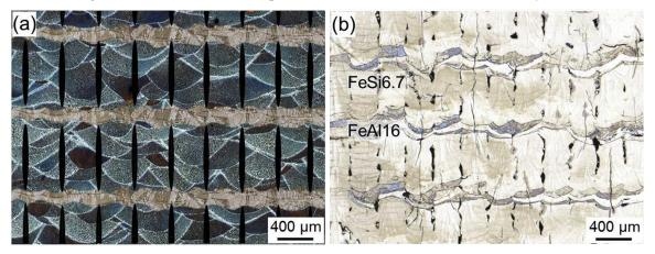
Figure 1.50 Example of an SMCs multilayered structures: (a) Schematic illustration, (b) AM Prototype of alternating layers of FeSi6.7, and FeAl16 (OM image shows part of the cross-section) [108]
