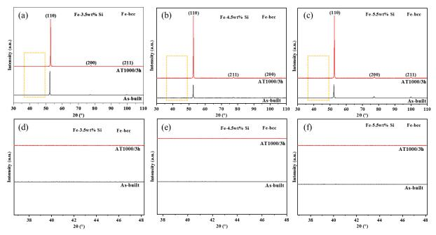
Figure 5.12 XRD spectra of the SLMed as-built samples and AT1000/3h samples
