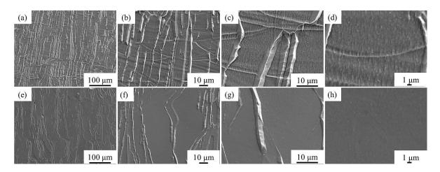
Figure 5.9 Microstructure of the SLMed Fe-3.5wt.%Si samples observed via SEM after etching: (a-d) as-built sample, (e-h) AT1000/3h sample
