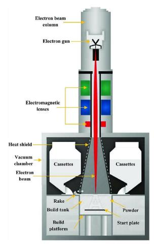
Figure 1.22 Schematic EBM system [168]
