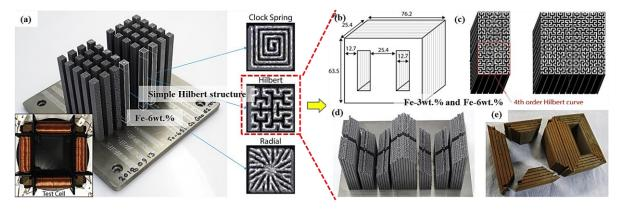
Figure 1.45 (a) SLM-build Fe-6wt.%Si thin wall cross-sections for magnetic characterization, (b) transformer core dimensions in mm (c) schematic of the Hilbert cross-section for thin and thick legs, (d) a finished SLM build (d) a partially assembled core after machining (adapted from [216])
