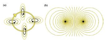
Figure 1.3 (a) Magnetic field around a loop of current, (b) a computer simulation of the cross-section showing the magnetic field lines [4]
