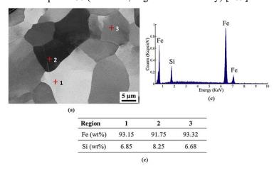
Figure 1.34 (a) SEM image of the investigated region, (b) EDX spectrum corresponding to region 1, (c) and chemical composition in the three regions under exam, of SLMed Fe-6.9%wt.Si [209]
