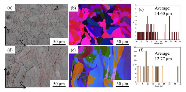
Figure 4.3 The EBSD maps of grain structure and average grain size of SLMed Fe-3wt.%Si specimen in different planes (a-c) XY plane, (d-f) XZ plane
