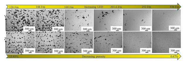
Figure 3.2 Effect of processing LED on sample porosity: the OM images of different SLMed Fe-3wt.%Si samples fabricated under the parameters of group 1
