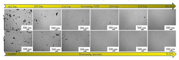
Figure 3.4 Effect of processing LED on sample porosity: the OM images of different SLMed Fe-3wt.%Si samples fabricated under the parameters of group 3
