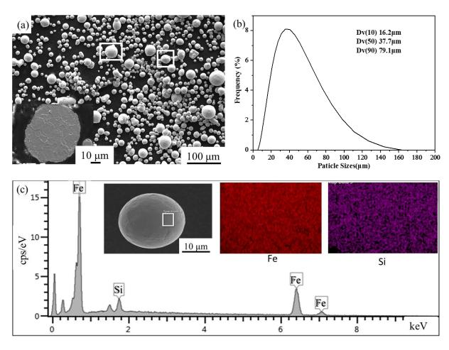
Figure 2.2 Characterization of Fe-3wt.%Si: (a) morphology and cross-section of the particles, (b) particle size distribution, (c) the results of EDS
