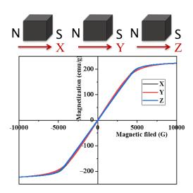
Figure 4.5 The hysteresis loops of SLM produced sample along with three directions of measurements
