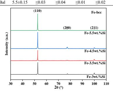
Figure 2.5 XRD spectra of the raw powders
