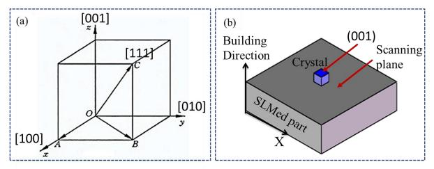
Figure 4.10 (a) A simple cubic crystal structure, (b) A simple schematic diagram of SLMed part with cubic texture
