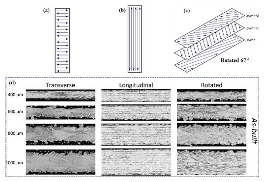
Figure 1.35 (a)-(c) Schematics of the scan patterns, (d) microstructures from the thin wall SLMed Fe-3Si samples [129]
