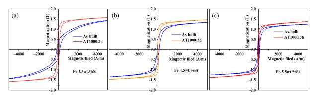
Figure 5.13 The measured DC hysteresis loops of three types of SLMed silicon steels (a) Fe-3.5wt.%Si, (b) Fe-4.5wt.%Si, (c) Fe-5.5wt.%Si
